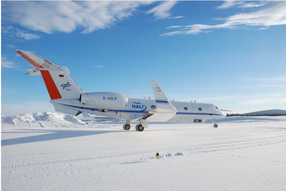
**Figure 3.4:** GLORIA mounted in the belly pod below the HALO research aircraft. The photograph was taken just before take-off for research flight PGS19 on 13 March 2016. Photographer: Björn-Martin Sinnhuber.
