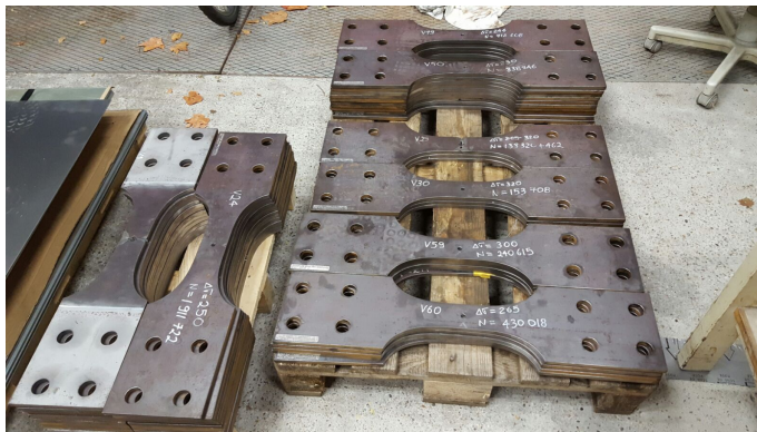
Figure 4.29: Steel S355J2+N. Tested specimens - After fatigue testing.
