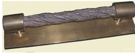
Figure 1.4: Wire rope - Original sample of the wire rope invented by Albert. It had 18 mm of diameter and consisted of three strands with four wires. Its calculated breaking load was 6000 kgf and it was tested for first time on 23.07.1834 on a depth of 484 m.
