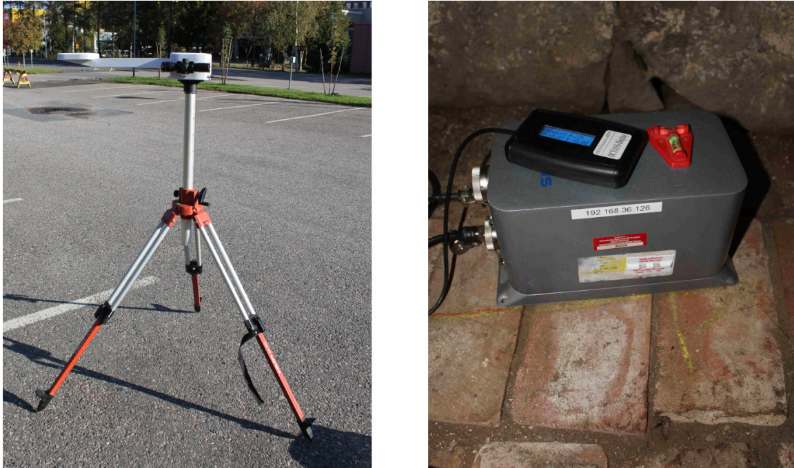
Figure 3.7: Azimuth Pointing System (APS) of the University of Oulu (left) and GIPP gyroscope of type iXblue OCTANS (right). Both instruments were used to correctly align the seismometers to true North during the installation or dismantling, respectively.
