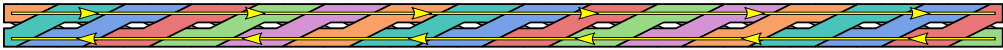
Figure 1.9: Coupling currents induced by a time-dependent magnetic field perpendicular to the wide face of the cable.
