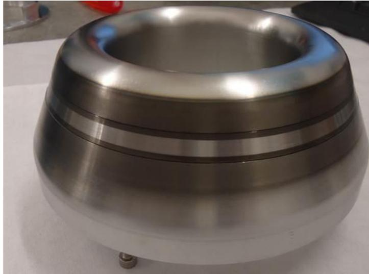
**Fig. 1.3.3:** MIG mock-up cathode with coated emitter edges.
