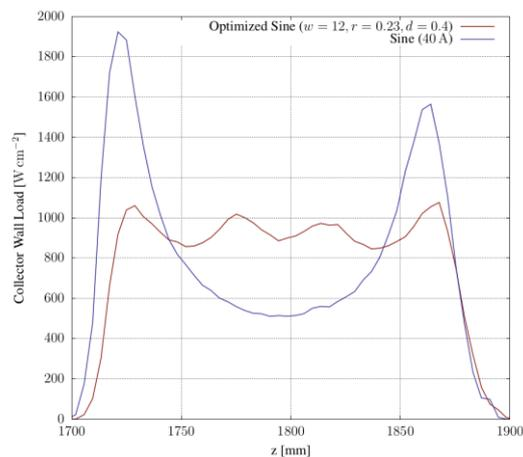
**Fig. 1.4.3:** Obtained averaged power density for the case of sinusoidal sweeping (blue) and sweeping with the advanced current waveform (red).
