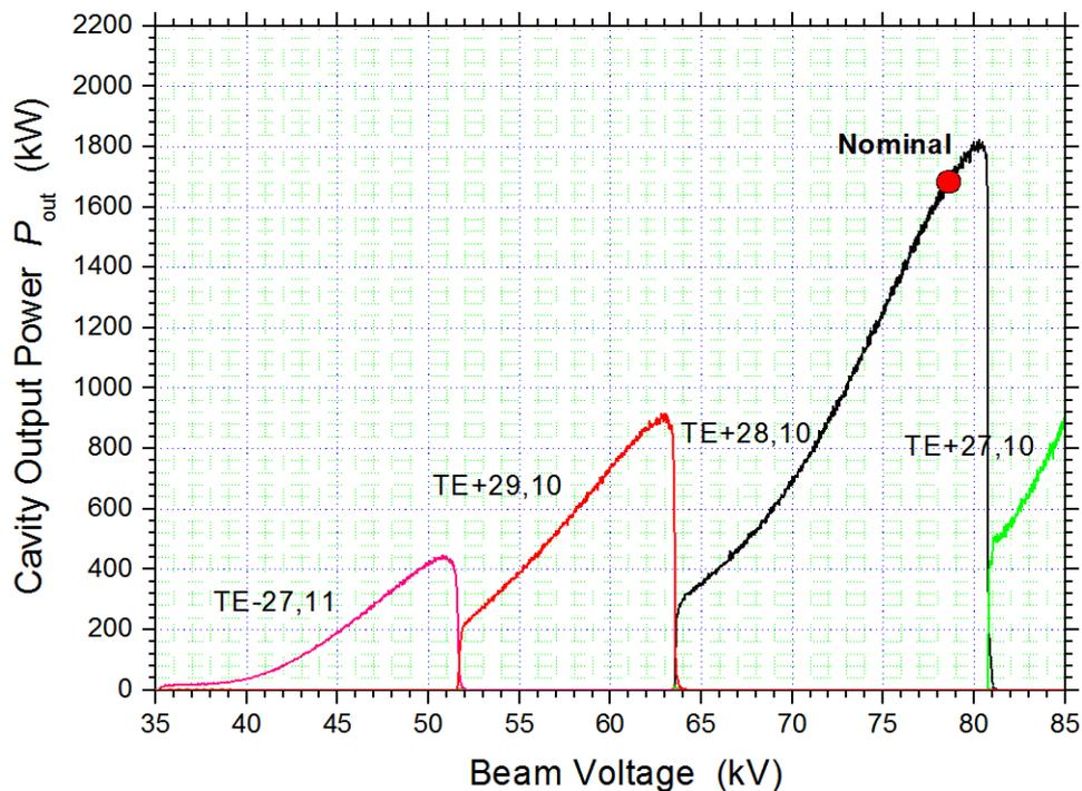
Fig. 1.1.1: Simulation of the TE<sub>28,10</sub>-mode gyrotron start-up considering 83 competing modes.
