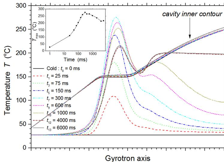
**Fig. 1.4.1:** Temperature profile along the inner contour of the cavity of the EU gyrotron for ITER, as obtained by transient multi-physics modelling. The change of the inner contour due to the thermal expansion is also shown. The inset shows the evolution of the maximum temperature with time.
