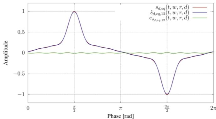
**Fig. 1.4.2:** Proposed current waveform for the enhanced sweeping concept, indicating the shape of the pre-defined current, its approximation by a Fourier series and the (negligible) corresponding difference  $e$ .
