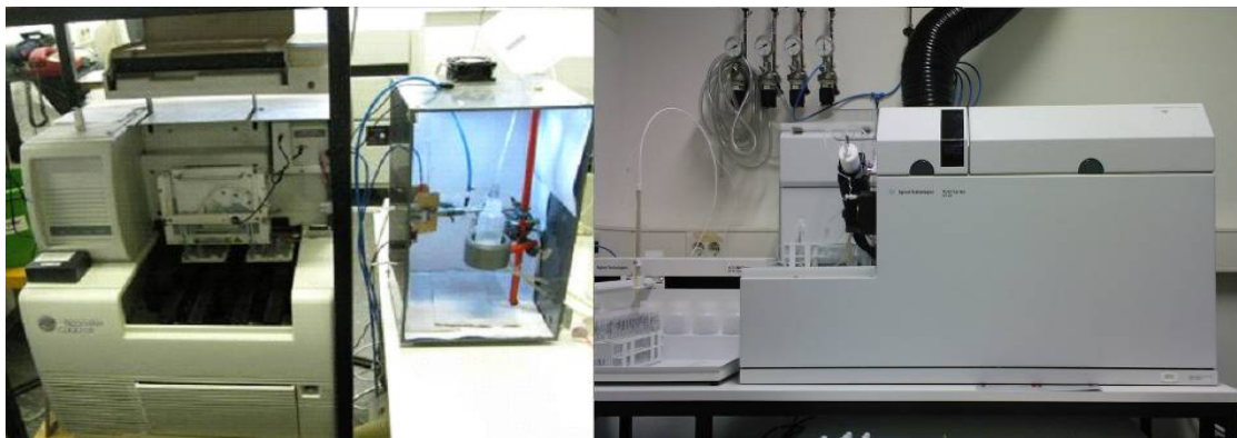
Figure 6: Hyphenation of CE and ICP-MS by the homemade interface
