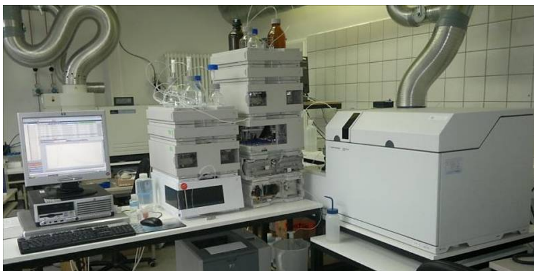
Figure 7: Hyphenation of HPLC with ICP-MS for MCCE setup
