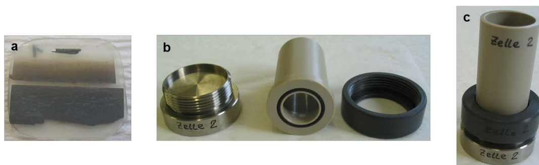
Figure 40: OPA thin section and sorption cell used for spatially resolved synchrotron radiation investigations: a: OPA thin section, b: parts of sorption cell, c: assembled sorption cell.
