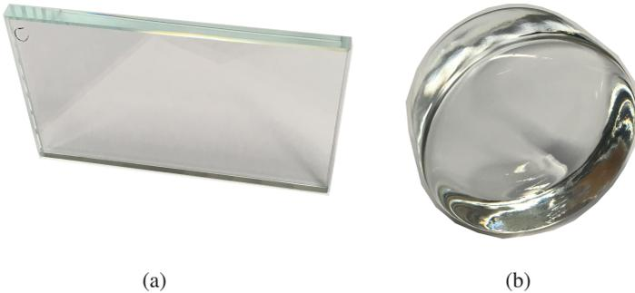
Figure 1.3: Different types of test objects: (a) a glass plate with a simple geometry is a cooperative test object; (b) a glass gob whose surface structure shows many variations is an uncooperative test object.
