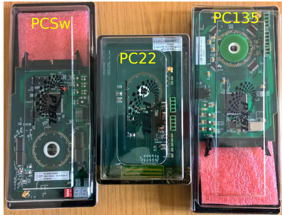
Figure 5.15: Photograph of the DCD and Switcher probe cards.
