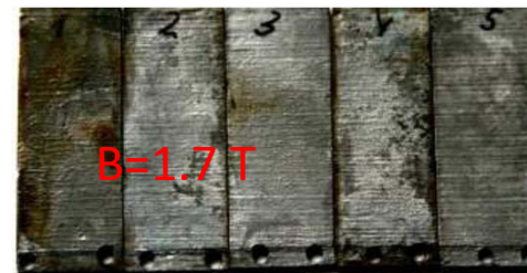
Corrosion of RAFM in PbLi under B-field
