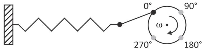
**Figure 3.2.:** Hooke's spring model for ideal elastic matter. A rotational movement with a constant angular frequency  $\omega$  is transferred as sinusoidal deformation to an elastic spring.
