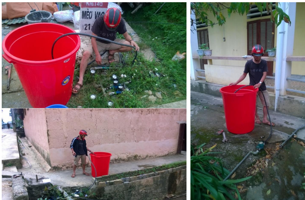
Figure 5.11. Measuring accurate meter on site
