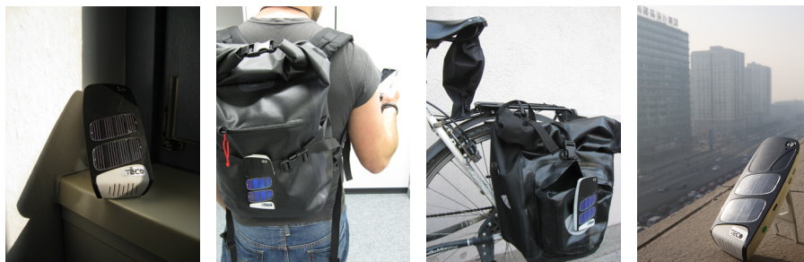
Figure 8.: The TECO Envboard [34] is a handheld multi-sensor platform for research and development.
