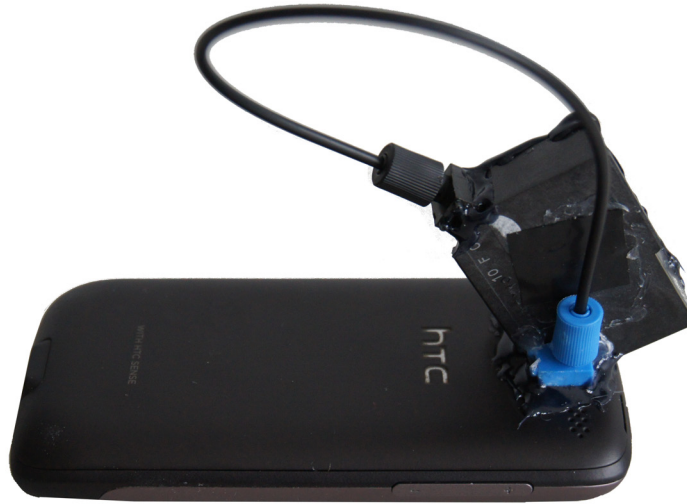
Figure 29.: HTC Desire phone with 1 st generation (proof-of-concept) prototype built from a Sharp GP2Y1010 dust sensor and an optical fiber devkit.
