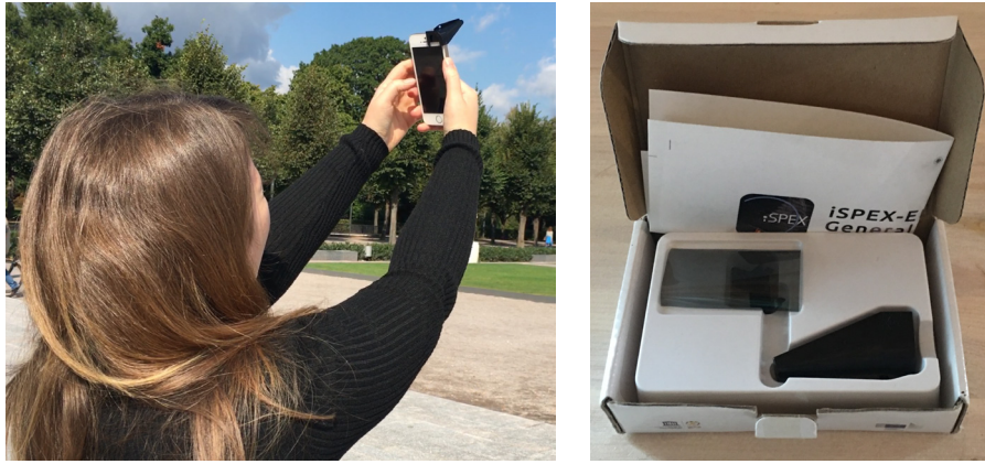
Figure 63.: Exploratory study 3: Participatory Air Quality Sensing using the iSPEX clip-on module [217] for the iPhone 5s .
