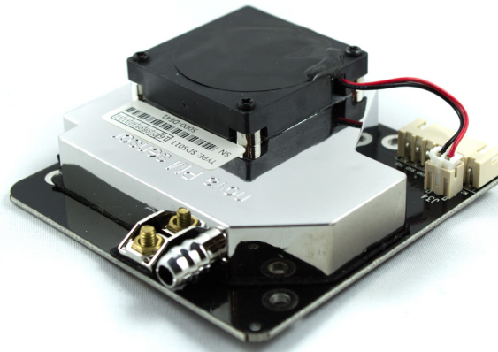
Figure 48.: Nova Fitness SDS011 laser-scattering sensor used in our experiments (image by UBAHNVERLEIH 1 ).
