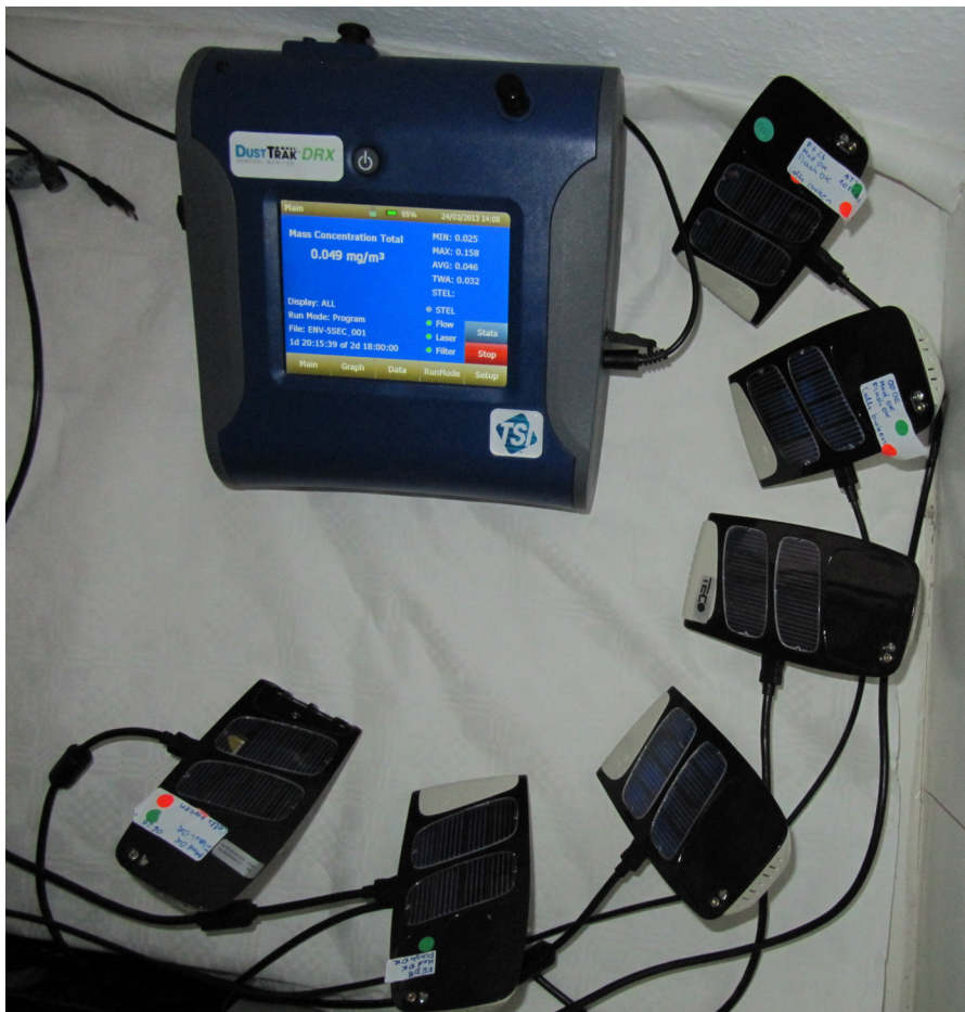
Figure 15.: Setup of the indoor lab evaluation: Six Envboards and the DRX8533 as reference.
