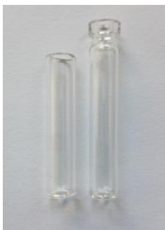
Figure 7.5.: Left: vial after removal of the top part; right: crimped photo glass vial. Adapted with permission from reference [184]. Copyright (2017) American Chemical Society (ACS).
