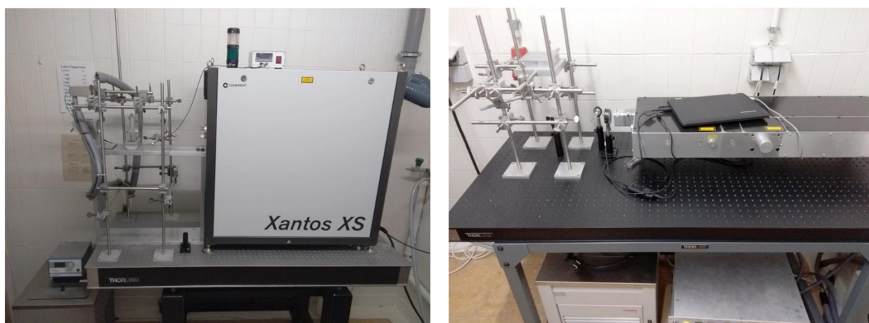
Figure 2.3.: Experimental PLP setup employed for polymer fabrication and photochemical end group transformation, utilizing an excimer laser (left side) or tunable-wavelength laser (right side).
