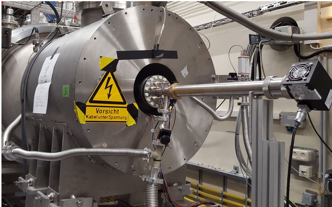
Figure VIII.4.: ELIOTT ion source inside the superconducting magnet of the rear section. At the end of the superconducting magnet, the ELIOTT vacuum feedthrough with the rods of the inner electrodes can be seen. Plastic screws were used at the feedthrough in order to electrically insulate the ELIOTT hull. The evacuated light guide was prolonged with another 540 mm long pipe in order to operate the UV lamp outside the magnetic field of the rear section superconducting magnet (right edge of the picture). Behind the light guide, electrical cables and the deuterium gas supply can be seen going into the magnet.
