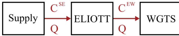
Figure A.9.: Simplified model of the ELIOTT vacuum setup at the rear section. The conductance C and the gas flow Q determine the pressures in the three volumes.
