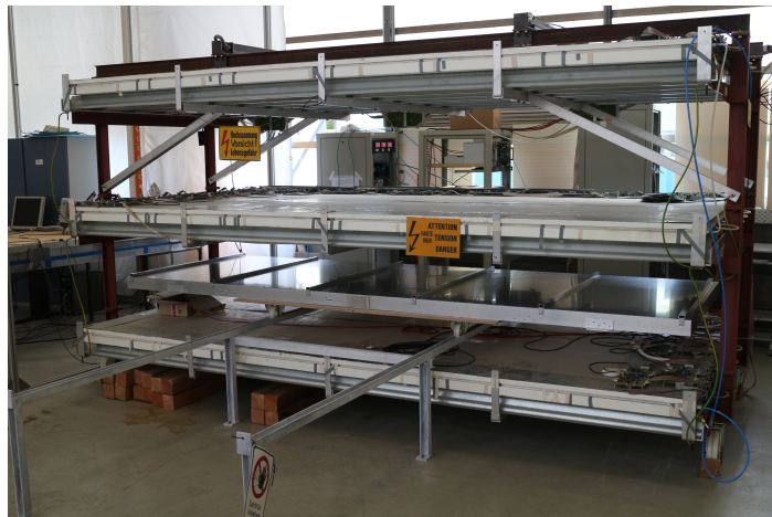
Figure 3.3: Muon telescope of the KASCADE muon tracker re-purposed for characterization of SSDs during the EA and production phases of AugerPrime.
