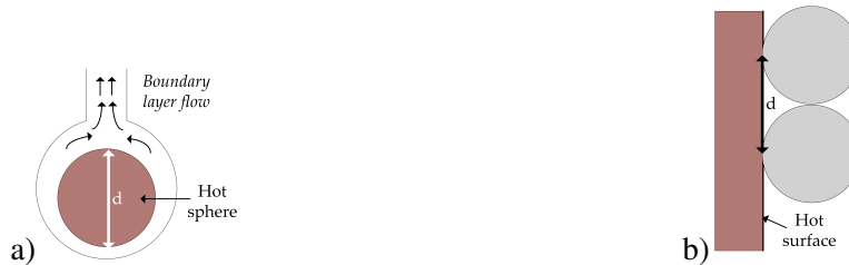
Figure A.1: a) Boundary layer flow around a single sphere (adapted from Ref. [213]); b) schematic illustration of the flow length at the tank wall in a packed bed
