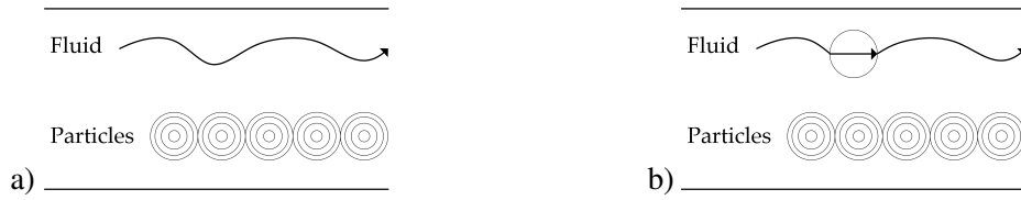
Figure 5.2: Schematic heat transfer models, a) fluid: dispersed plug flow, solid: concentric isotherms, b) modified effective thermal conductivity of fluid including solid phase (adapted from Ref. [146])
