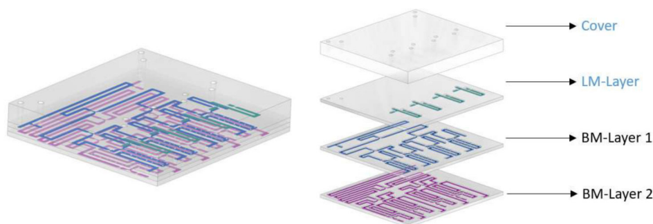
Figure 5.11. 3D-model and exploded view of the submodule, BM-Incubation, for mixing without cooling unit. Four layers of the module are shown: Cover, LM-layer, BM-layer 1, and BM-layer 2. The extra layers required for a standalone T-Module are marked in blue.
