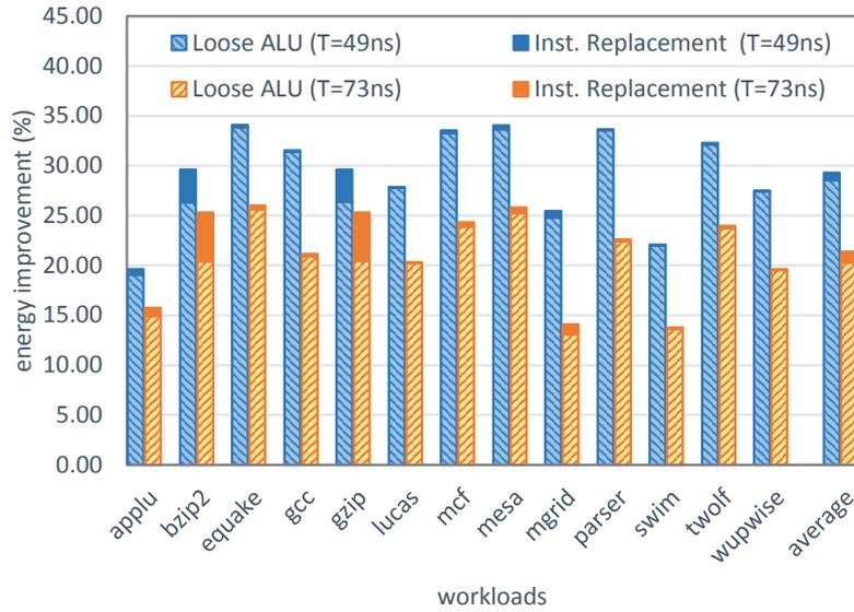
Figure 4.8: Energy improvement over the baseline (Tight ALU). The additional improvement is also calculated for when `addition` / `subtract` are replaced by `increment` / `decrement` when possible (clock period is 73ns and 49ns).
