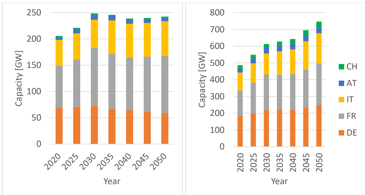
Figure 22: Cumulated conventional capacity development (left) and the total installed capacity (right) in the CRM Policies scenario in Switzerland and its neighbouring countries.
