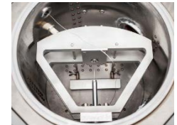
Nail penetration test in ARC
