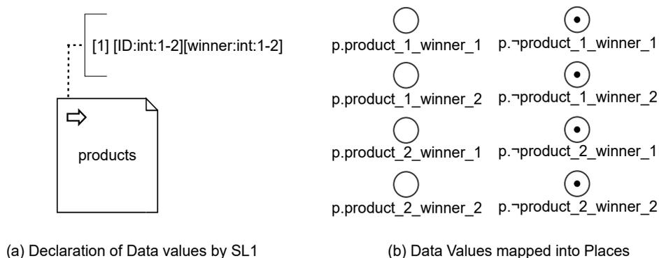
Figure 4: Mapping the Data Values to Petri Net Places
