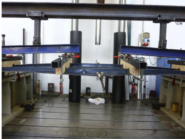
Fig. 11. Failure mode (local buckling of the upper flange) of curved trapezoidal sheets profile (39/333), thickness 0.63 mm. Configuration A.
