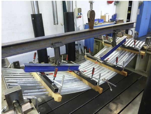
Fig. 9. Failure mode (plastic deformation) of curved sinusoidal sheets profile (18/76), thickness 1.00 mm. Configuration A.
