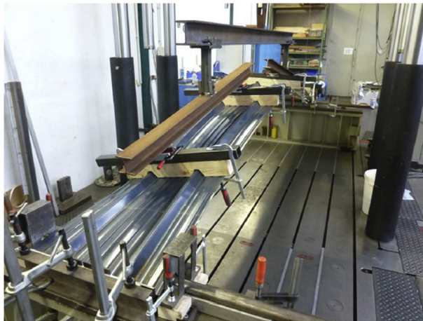
Fig. 18. Side view of the failure mode (buckling of the arch) of curved trapezoidal sheets profile (39/333), thickness 0.63mm. Configuration B.
