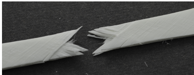
Figure 3.52: Failed \pm 45^\circ off-axis specimen after tensile test. Close-up view of fracture area.
