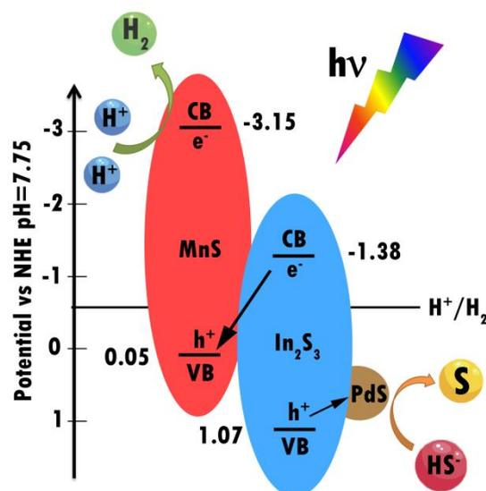
**Fig. 8** The band structure and photocatalytic mechanism of MI-Pd under visible light irradiation
