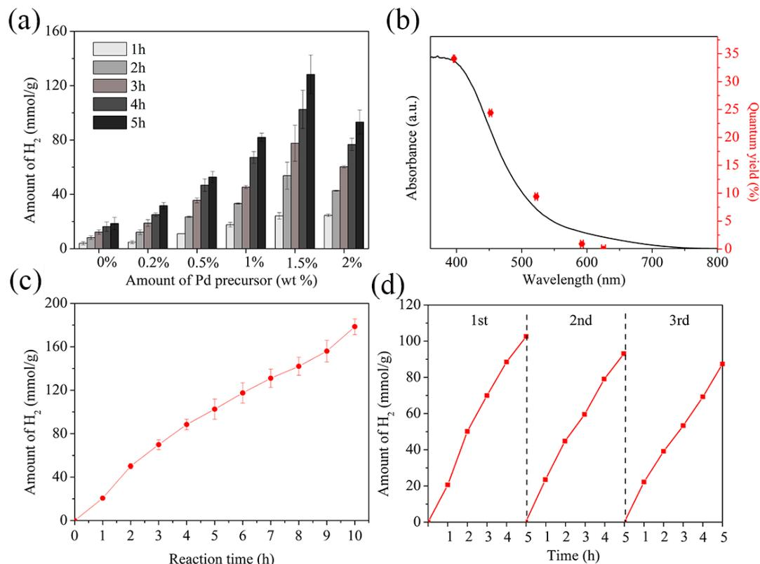
**Fig. 1** Photocatalytic hydrogen production rate of MI, and MI-Pd X % (X = 0.2 ~ 2) (a); ultra-violet and visible light diffuse reflectance spectra and apparent quantum yield at different wavelength of MI-Pd 1.5 % (b); 10 h long period photocatalytic hydrogen production rate of MI-Pd 1.5 % (c); three rounds cyclic photocatalytic hydrogen production rate of MI-Pd 1.5 % (d)
