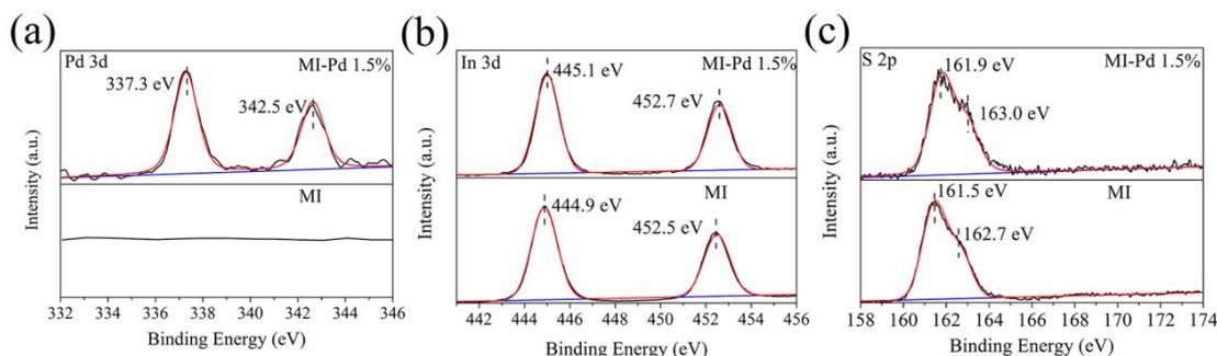
**Fig. 4** X-ray photoelectron fine spectra Pd 3d (a), In 3d (b), and S 2p (c) of MI, and MI-Pd 1.5%
