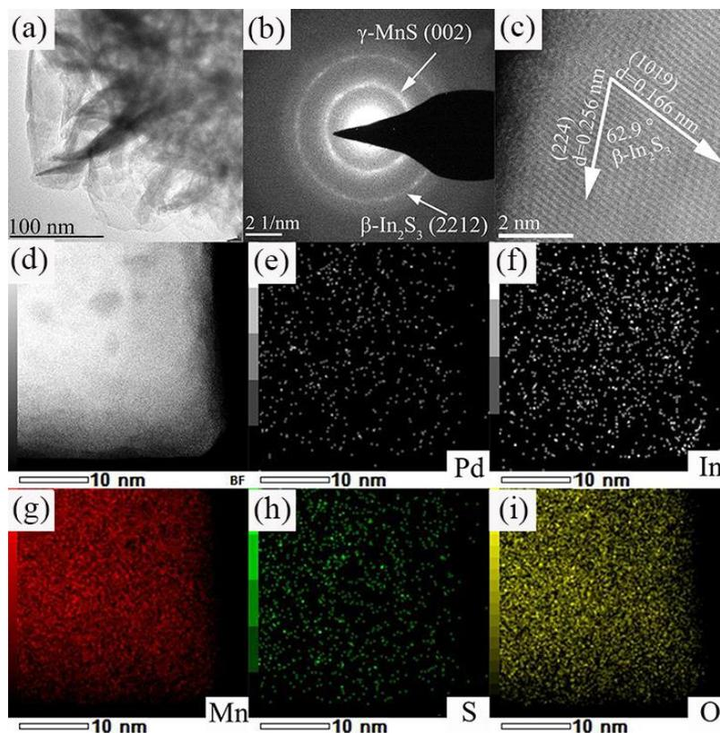
**Fig. 3** Transmission electron microscope image (a), selected area electron diffraction (beam diameter: 200 nm) image (b), spherical aberration corrected scanning transmission electron microscope atomic resolution high-angle annular dark-field image (c), and energy dispersive X-ray spectrum element maps - selected area (d), element Pd (e), element In (f), element Mn (g), element S (h), element O (i) of MI-Pd 1.5%
