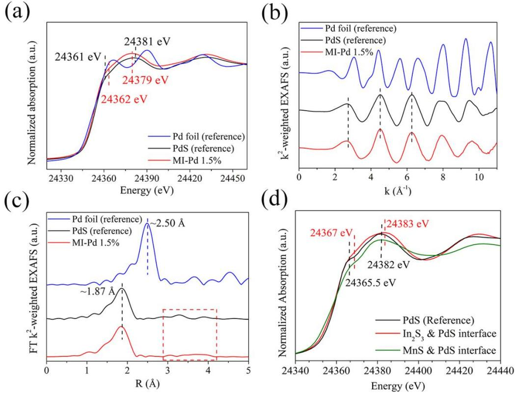
**Fig. 5** Normalized X-ray absorption near edge spectra (a),  $k^2$ -weighted extended X-ray absorption fine spectra (b), and Fourier-transformed  $k^2$ -weighted extended X-ray absorption fine spectra (c) of MI-Pd 1.5% (fresh), Pd foil reference and PdS reference; theoretical X-ray absorption near edge spectra (d) of  $\text{In}_2\text{S}_3$  & PdS interface, MnS & PdS interface and PdS reference
