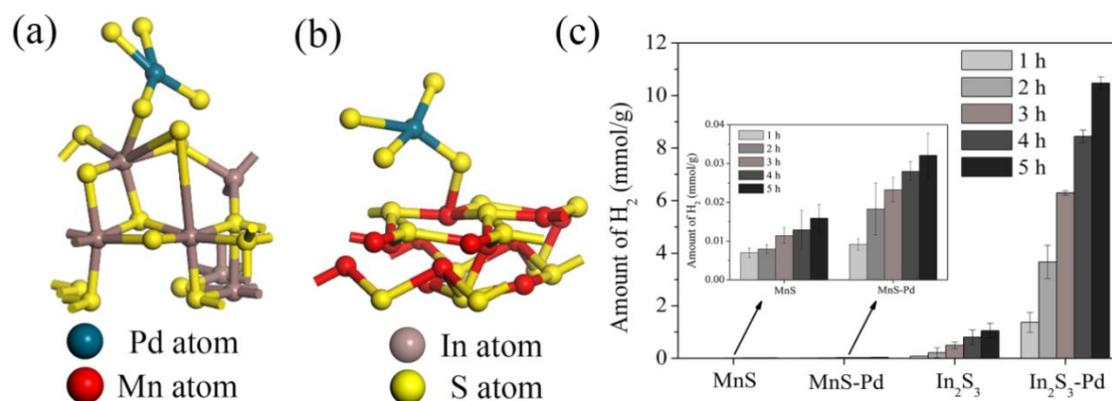
**Fig. 6** The model structures of In<sub>2</sub>S<sub>3</sub> & PdS interface (a) and MnS & PdS interface (b); photocatalytic hydrogen production over MnS, MnS-Pd, In<sub>2</sub>S<sub>3</sub>, and In<sub>2</sub>S<sub>3</sub>-Pd within 5 h. (The added Pd precursor amount is 1.5% which is consistent with MI-Pd 1.5%)(c)
