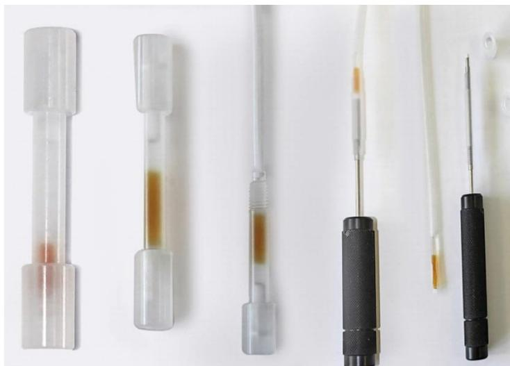
**Figure 28:** Procedure to transfer a swollen gel from the swelling device to the tubing.
