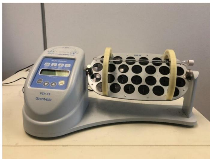
**Figure 56:** Vertical rotating shaker 360° PTR-35 Grant-Bio adapted for 5 mm NMR tubes.
