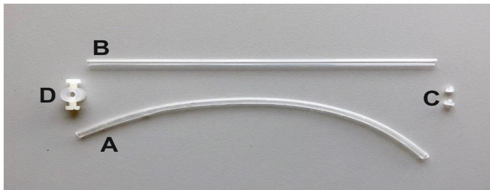
**Figure 13:** 5 mm stretching device designed by Kummerlöwe for all commonly used solvents. The device is composed of a Kalrez tube (A), an open cut 5 mm NMR tube (B), a specially designed Polychlorotetrafluoroethylene (PCTFE) screw (C) and a Kel-F/PCTFE cap with 2 screws (D).
