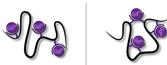
Figure 2.18: Gadolinium(III)-decorated linear metallopolymers vs Gd(III)-SCNPs. For their suitability as contrast agents for magnetic resonance imaging, the Gd(III)-containing substances require reduced internal flexibility, achieved by crosslinking the chains into nanoparticles.
