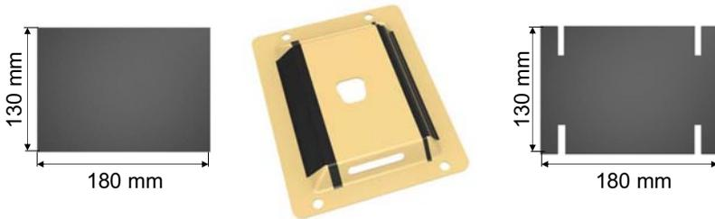
Figure 5-14: Two SMC sheets for the demonstrator of GRK 2078
