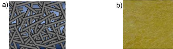
Figure 2-4: Structure of a sheet molding compound(a) and real material (b)
