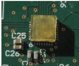
Figure 3.14: Sensor covered with a protecting cap.
