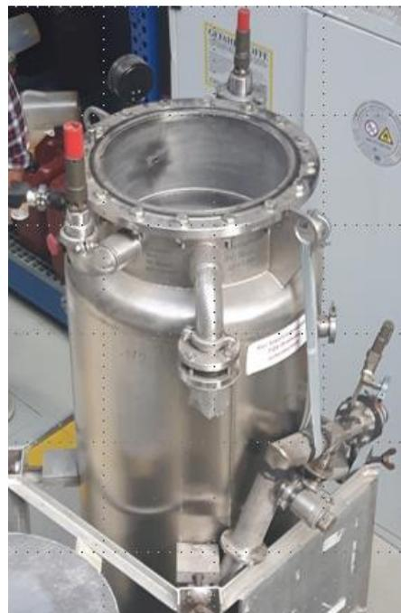
Fig. 23: Experimental set-up CRYO-VESSEL for two phase cryogenic hydrogen blow-downs
