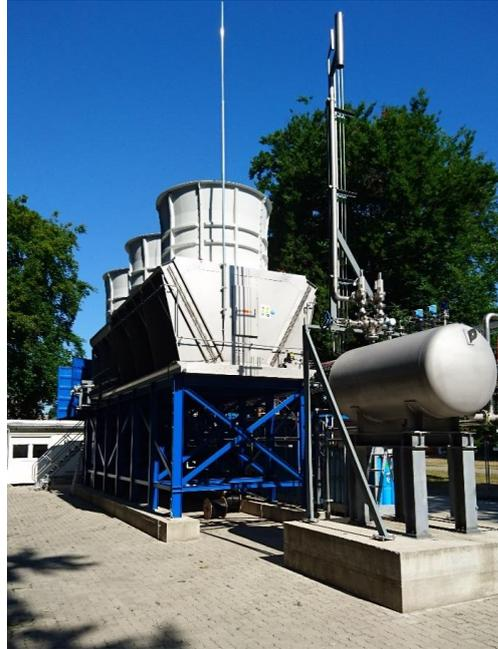
Fig. 8: Test facility MONIKA with a Rankine cycle of supercritical propane.
