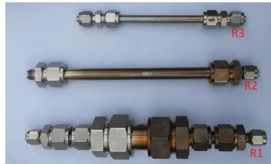
Fig. 26: Tested catalytic reactor variants
