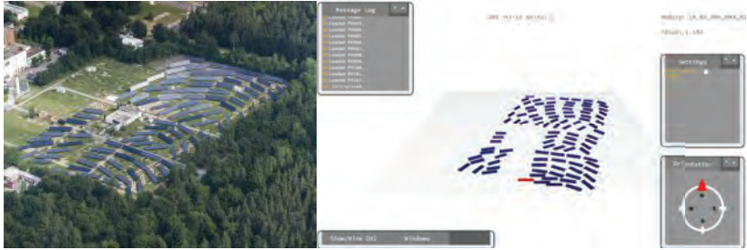
Figure 4.9.: Left image shows an aerial view of the KIT 1 MW Solar Plant at the Karlsruhe Institute of Technology, Eggenstein-Leopoldshafen. The right picture shows the data display built with the BORA framework. Blue colour represents the solar panel that is generating power; whereas the red colour represents no power generated.
