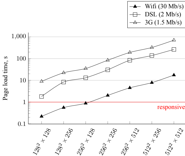
Figure 4.24.: Latency for multi-resolution slicemaps on slower network presets, i.e., Wifi, DSL, and 3G.
