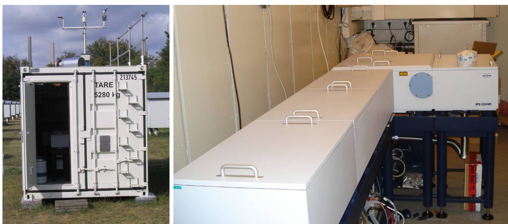
Figure 2.2: Shipping container (left panel) and TCCON FTIR spectrometer (right panel) at KIT - Campus North, Karlsruhe, Germany. Figures were taken by Dr. Thomas Blumenstock.
