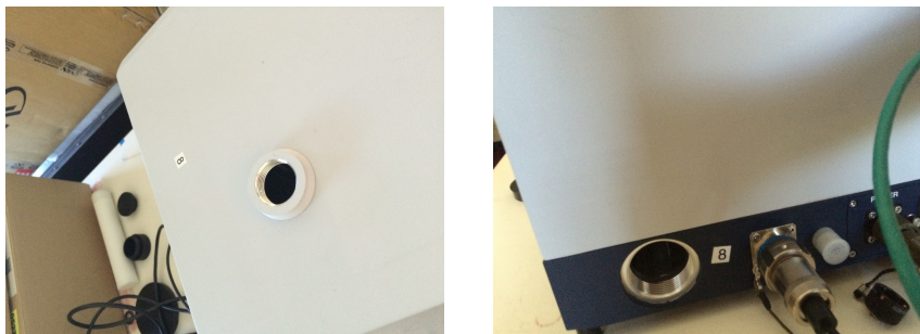
Figure 2.8: Two apertures located on the top and lower side of the EM27/SUN instrument are open for the ventilation.
