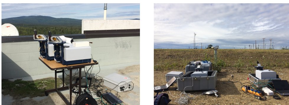
Figure 5.2: Side-by-side measurements on the GI roof, UAF (left) and at Poker flat (right) using the KIT and LANL EM27/SUN FTIR spectrometers.
