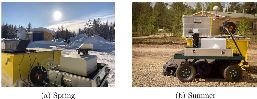
Figure 2.5: The EM27/SUN spectrometer operated at FMI, Sodankylä in early spring (a) and summer (b). The right figure was taken by Dr. Friedrich Wilhelm Klappenbach.
