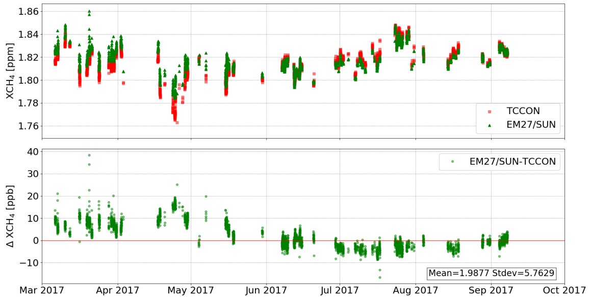
Figure 4.18: Time series of XCH_4 from the TCCON 125HR and the EM27/SUN instruments (upper panel) and the bias between them (lower panel).
