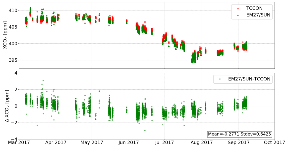
Figure 4.16: Time series of XCO 2 from the TCCON 125HR and the EM27/SUN spectrometers (upper panel) and the bias between them (lower panel).
