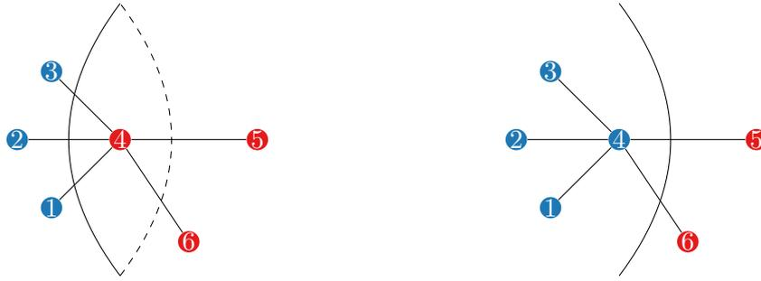
Figure 4.1: Moving vertex 4 from the red block to the blue block has a gain of 1. Before the move, three edges were cut. After the move, only two edges are cut.
