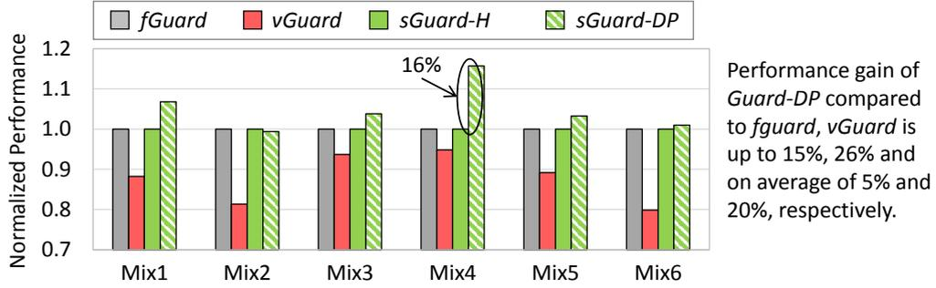
Figure 9.6: Comparison results of the average performance between *sGuard-DP*, *sGuard-H*, *vGuard* and *fGuard* techniques under *static* workloads that consist of different multiple applications.
