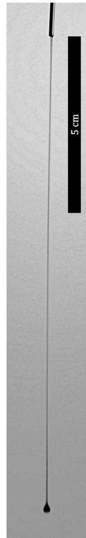
**Figure 1.1:** Formation of a long surfactant filament, dripping from a nozzle.
