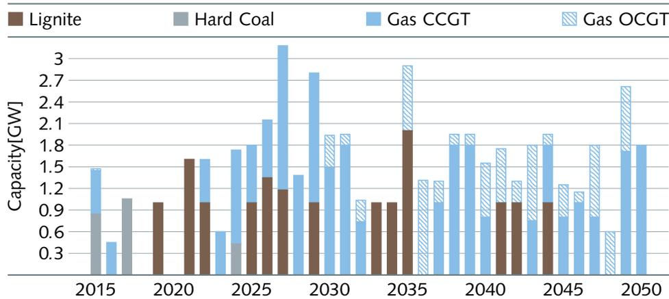
**Figure 7.5 | Newly constructed capacities in reference scenario.** In the beginning, lignite power plants are chosen as the most profitable investment. However, starting in 2021, investments in OCGTs and CCGTs are also favorable. With the rising carbon prices in mid-2030's, lignite-fired power plants are no longer being built and gas-fired power plants remain as an economically favorable technology.
