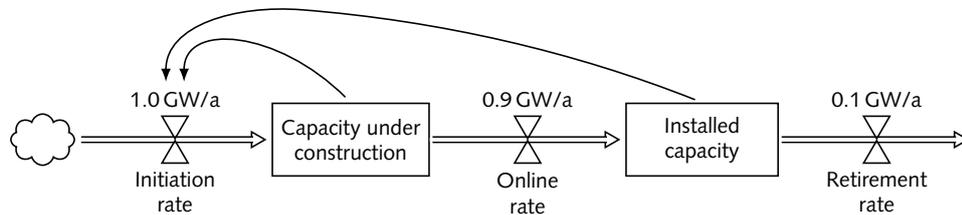
**Figure 3.5 | Capacity stocks and flows in a system dynamics model.** This diagram shows an exemplary flowchart (cf. Ford, 1997), in which the stocks (“capacity under construction” and “installed capacity”) describe the current state of the system and are used as the basis for deriving decisions as well as actions, for example, the initiation rate. The rates, on the other hand, describe the actions in the system, which in turn cause changes to the inventory levels (Pereira and Saraiva, 2011).
