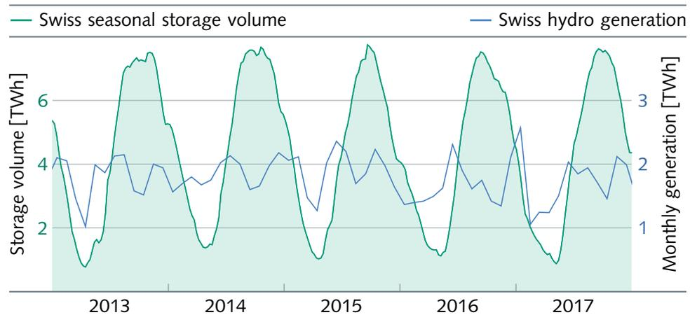
**Figure 9.10 | Historical and simulated storage volumes.** In contrast to the storage level, which has a clear annual profile, the generation of hydropower does not exhibit a pronounced recurrent pattern. This suggests that the monthly generation through water turbines excluding pumped storage lies within certain limits, but reacts dynamically to market developments.
