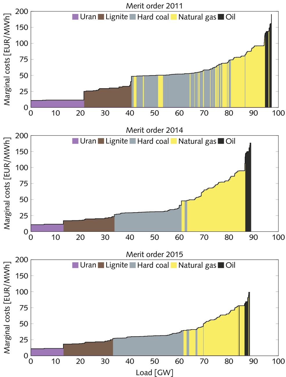
**Figure 4.2 | The merit order of the conventional capacities in Germany.** When examining the different merit orders, two aspects stand out. First, the total capacity has been severely reduced as a result of the nuclear phase-out. Second, the marginal costs, especially for coal and gas-fired power plants, are sharply lower. *Sources:* EEX (2016); BNetzA (2016d).
