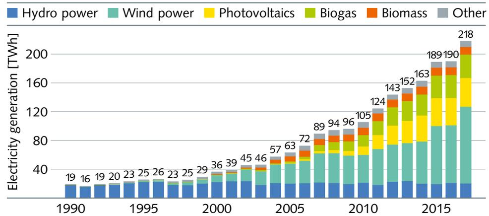
**Figure 2.7 | Renewable electricity generation in Germany.** Since the introduction of the EEG in 2000, the generation from renewable energies has increased strongly. Biogas, photovoltaics and wind power plants account for the largest share of this development. As the potential of hydropower in Germany has already been widely exploited early on, its generation has remained comparatively constant. *Source: BMWi (2018c).*
