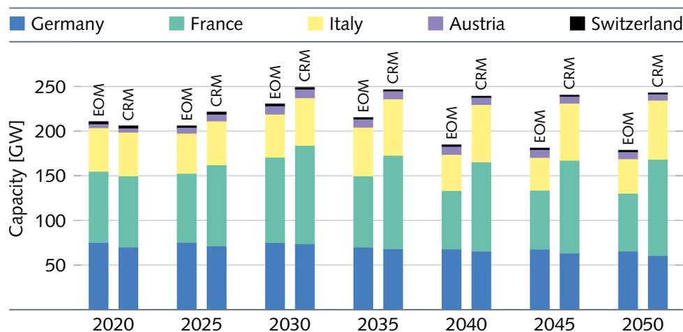
**Figure 9.7 | Cumulated conventional capacity.** The main differences between the EOM and in the CRM Policies scenario can be seen in France and Italy. There, the introduction of capacity markets leads to higher capacities from 2025 onwards and to a more constant conventional capacity development than in the EOM scenario.
