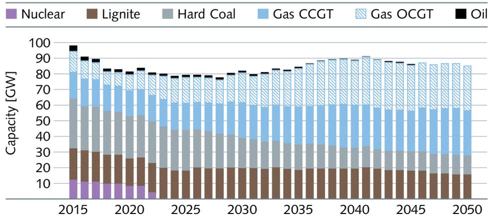
**Figure 7.9 | Capacities in the capacity market scenario.** The central capacity market leads to a high volume of power plant capacities, whereby the differences compared to the reference scenario are almost exclusively due to a higher investment in OCGTs. This is due to the fact that these additional power plants are rarely used or, in extreme cases, are not used at all and, therefore, their low fixed costs are decisive.
