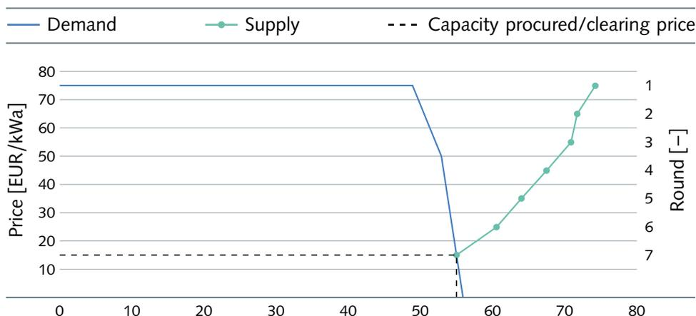
**Figure 7.2 | Descending clock auction.** In this schematic illustration of a descending clock auction, it can be observed how the supply of electricity generators and the demand of the regulator converge. The oversupply in the first round of almost 20 GW is gradually reduced, and completely eliminated in the seventh round, resulting in a clearing price of 15 EUR/kWa and contracted capacities of 55 GW.
