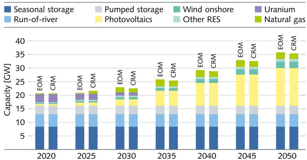
**Figure 9.8 | Swiss capacity in the EOM and CRM Policies scenario.** The most significant developments are the complete decommissioning of nuclear power plants by 2035, which are being replaced by new investments in gas-fired combined cycle power plants and the expansion of renewable energies, especially photovoltaics.
