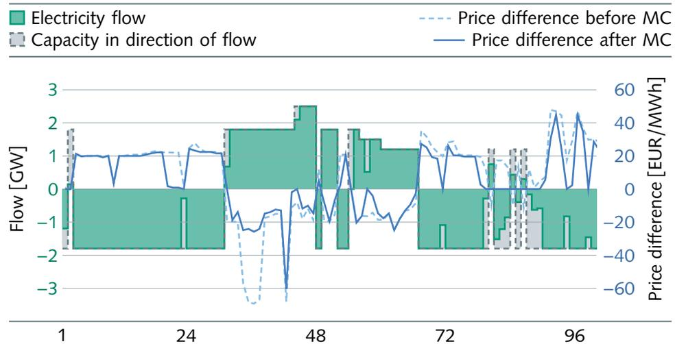
**Figure 8.1 | Market coupling.** The simulated electricity flow and price difference between Germany and France for a period of 100 hours in 2012 is depicted. In most cases, the available interconnecting capacity of up to 2.5 GW is used to its full extent, yet in some cases, the price difference still exceeds 60 EUR/MWh. If the capacity is not fully utilized, both market areas share an identical price after market coupling.
