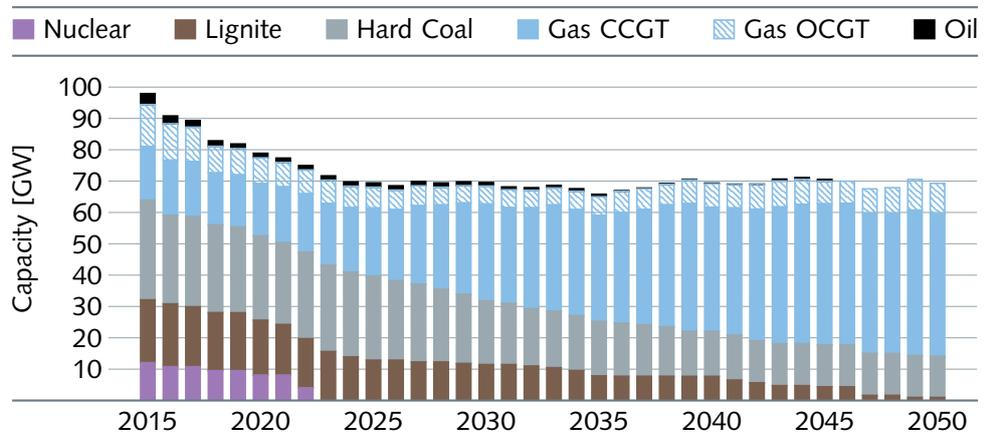
**Figure 7.15 | Development of the conventional capacities with a lignite phase-out.** In this phase-out scenario, the construction of additional lignite-fired power plants is prohibited, but existing plants may remain in operation. Compared to the reference scenario, lignite capacities are largely replaced by additional gas-fired power plants.
