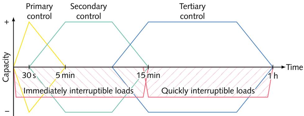
**Figure 2.6 | Chronological sequence of the usage of the operating reserves and interruptible loads.** Transmission system operators have three different reserves at their disposal, which can be utilized successively if a power imbalance occurs. Additionally, since the amendment to the Energy Industry Act of 20 December 2012, quickly or immediately interruptible loads can be accessed if negative balancing power is required.
