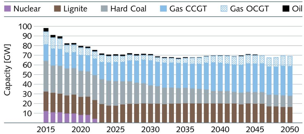
**Figure 7.6 | Dispatchable capacities in the reference scenario.** The capacity development shows that coal-fired power plants are steadily being replaced by CCGTs. However, lignite power plants remain highly profitable mainly due to the low fuel costs and only slightly increasing carbon certificate prices in the reference scenario.
