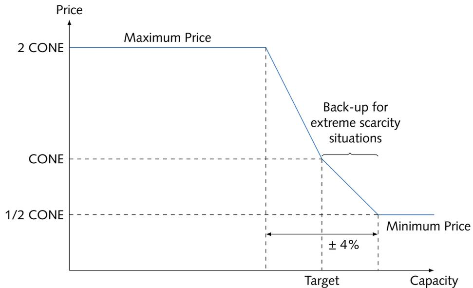
**Figure 7.1 | Capacity demand curve.** To be more robust against market power, the demand curve should be elastic near the targeted capacity level and, ideally, reflects the marginal value of firm energy. Source: Cramton and Ockenfels (2012).
