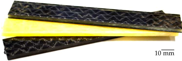
Figure 3.6: From bottom to top: continuous carbon fibre SMC, discontinuous glass fibre SMC and hybrid continuous-discontinuous glass/carbon fibre SMC.
