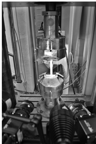
Figure 4.3: Tensile test setup with stereo digital image correlation (DIC).
