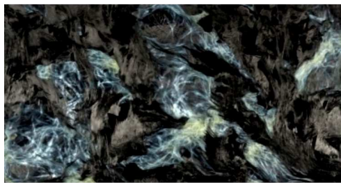
Figure 2.22: Hybrid glass/carbon fibre reinforced SMC sheet in interlayer configuration based on stacking of chopped glass and carbon fibres reinforced semi-finished sheets prior to moulding and manufactured within the framework of the IRTG (GRK 2078).
