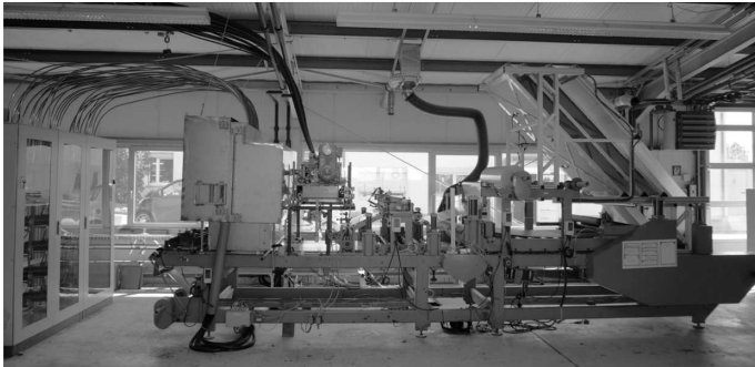
Figure 3.1: SMC manufacturing line at Fraunhofer ICT (image provided by Fraunhofer ICT).
