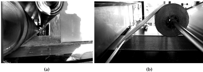
Figure 3.2: Feeding of fibrous reinforcement to the conveyor belt: chopped glass fibres (a) or unidirectional non-crimp carbon fibre fabric (b) (images provided by Fraunhofer ICT).
