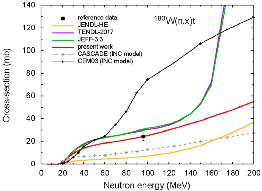
Fig.14 Triton production cross-section for  $^{180}\text{W}$ .
