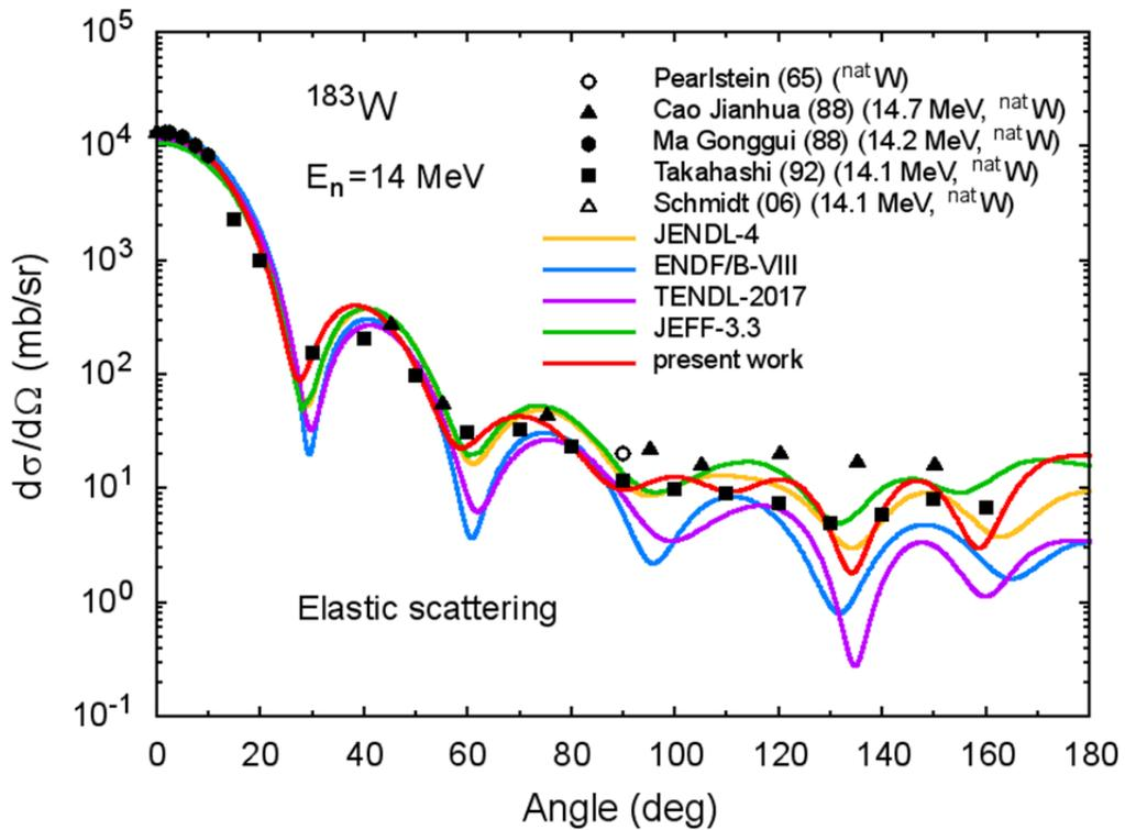
Fig.25 Elastic scattering angular distribution of neutrons for  $^{183}\text{W}$  irradiated with 14 MeV neutrons.
