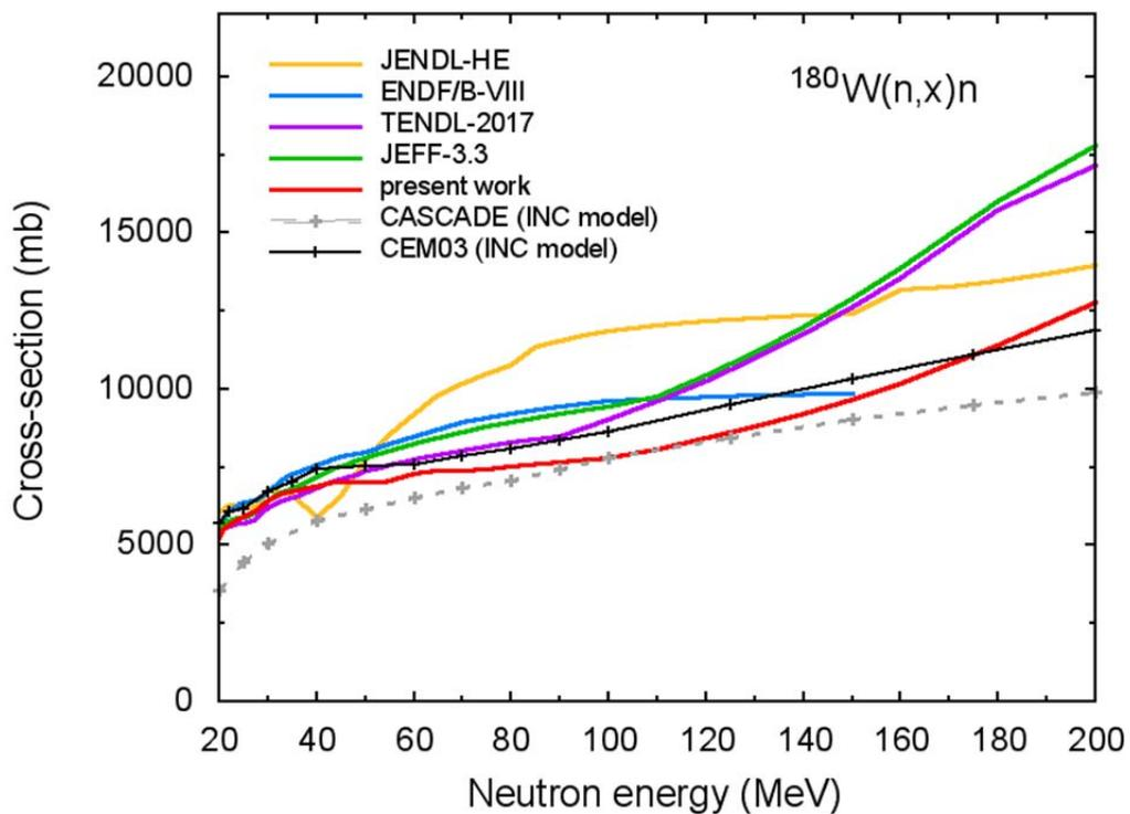
Fig.11 Neutron production cross-section for  $^{180}\text{W}$ . See explanations in the text.
