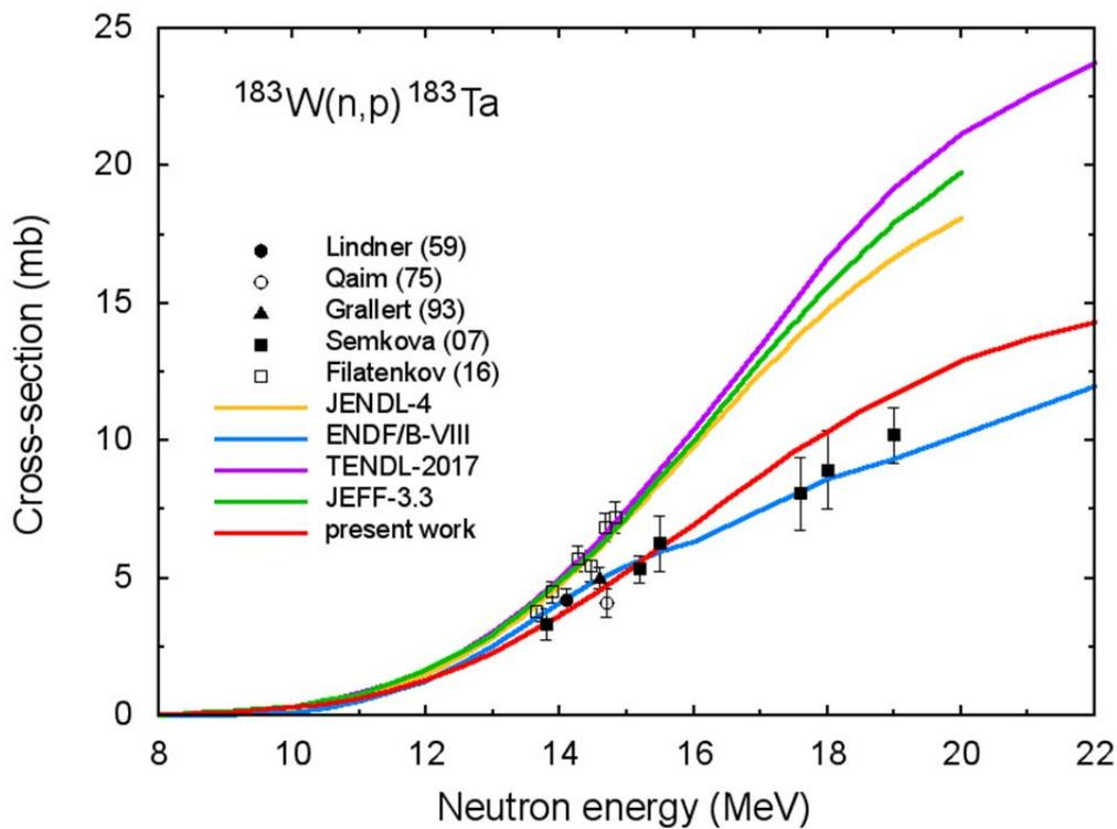
Fig.31 (n,p) reaction cross-section for  $^{183}\text{W}$ .
