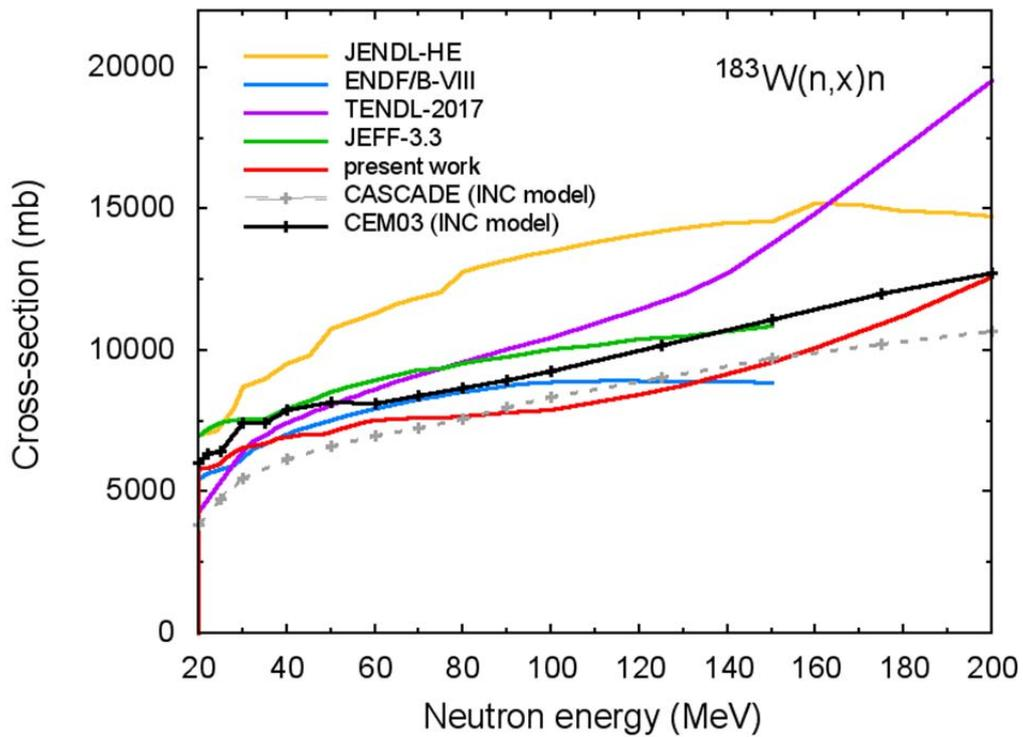
Fig.40 Neutron production cross-section for  $^{183}\text{W}$ .
