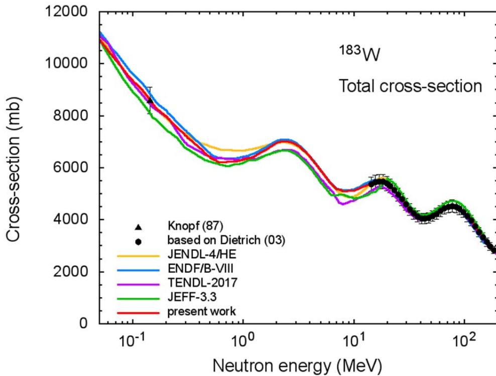
Fig.18 Total reaction cross-section for neutron irradiation of  $^{183}\text{W}$  evaluated in the present work, measured data, cross-section derived using experimental data for tungsten isotopes  $^{182,184,186}\text{W}$  (“based on Dietrich (03)”), and data taken from different libraries. See explanations in the text.
