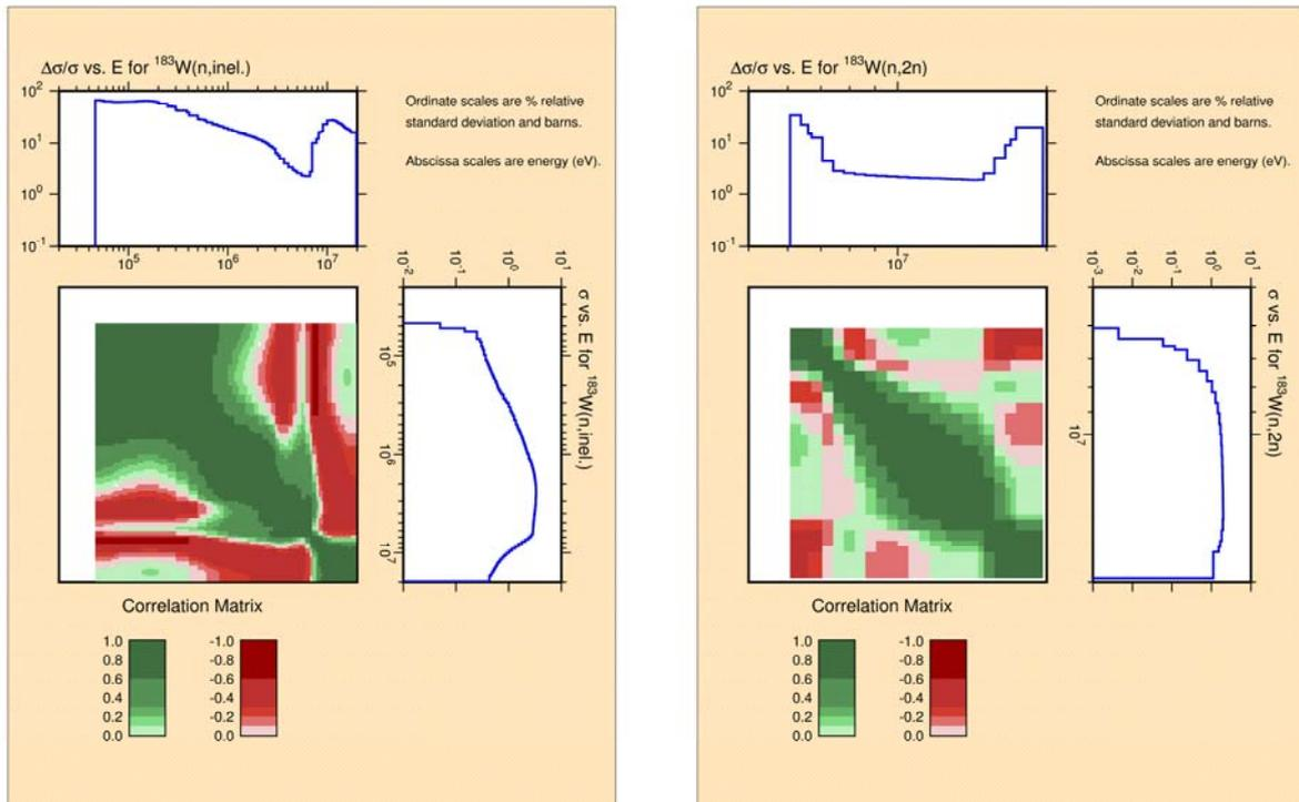
Fig.48 Example of covariance matrices calculated for neutron inelastic scattering cross-section (n,n)' and (n,2n) reaction cross-section for  $^{183}\text{W}$ . Plots were prepared using the NJOY code.
