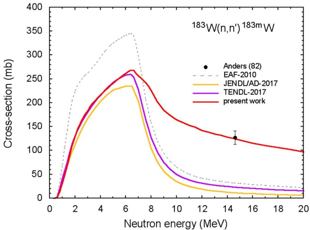
Fig.28 Inelastic scattering cross-section with production of  $^{183m}\text{W}$  isotope in the metastable state ( $T_{1/2}=5.25$  s). See discussion in the text.
