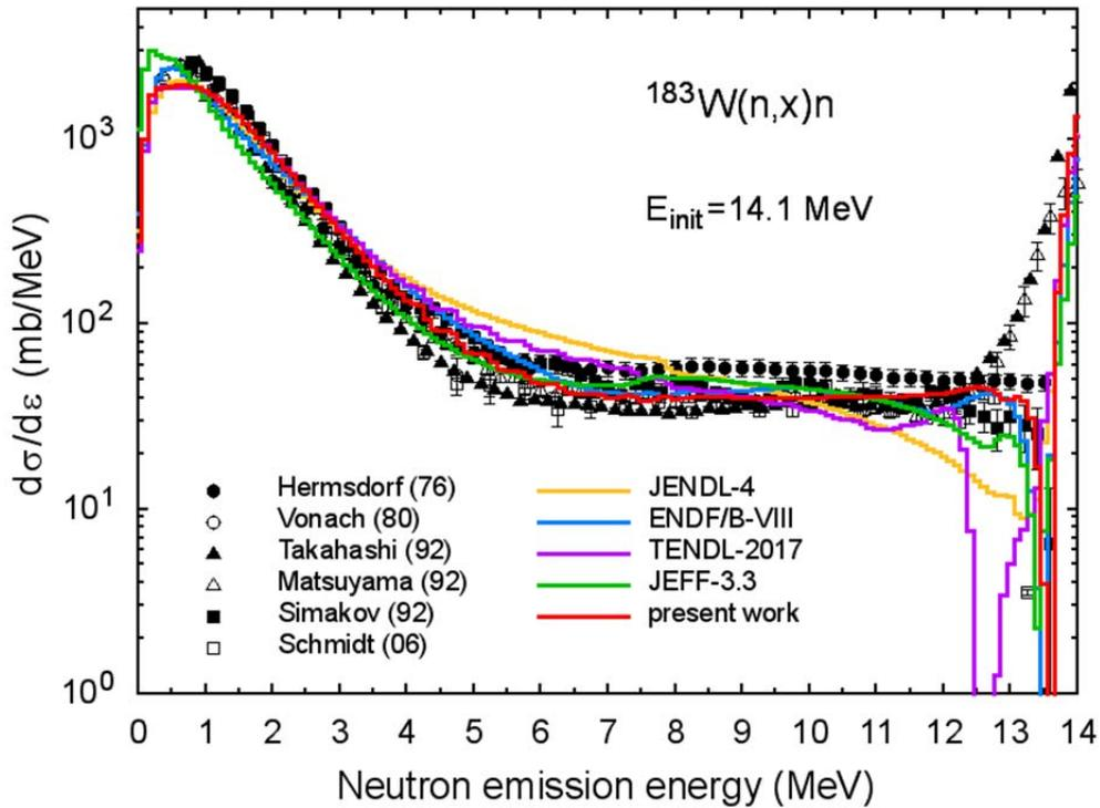
Fig.36 The same as in Fig.35 at neutron incident energy 14.1 MeV
