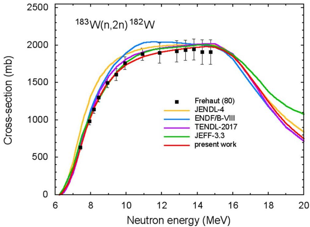
Fig.30 (n,2n) reaction cross-section for  $^{183}\text{W}$ .
