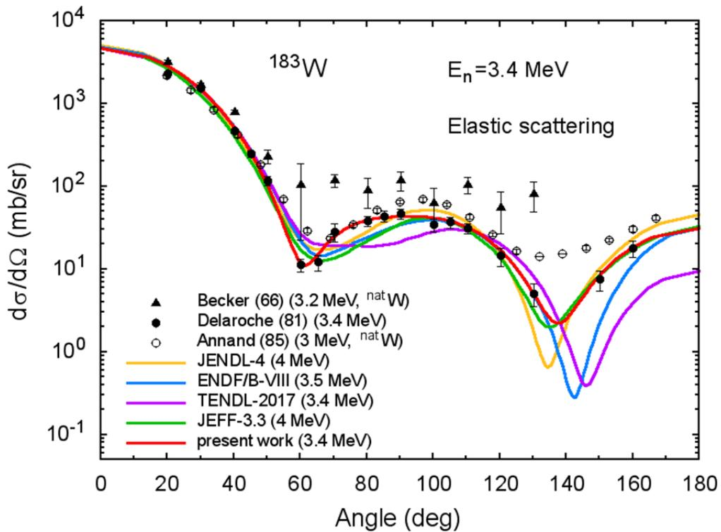
Fig.23 Elastic scattering angular distribution of neutrons for  $^{183}\text{W}$  irradiated with 3.4 MeV neutrons.
