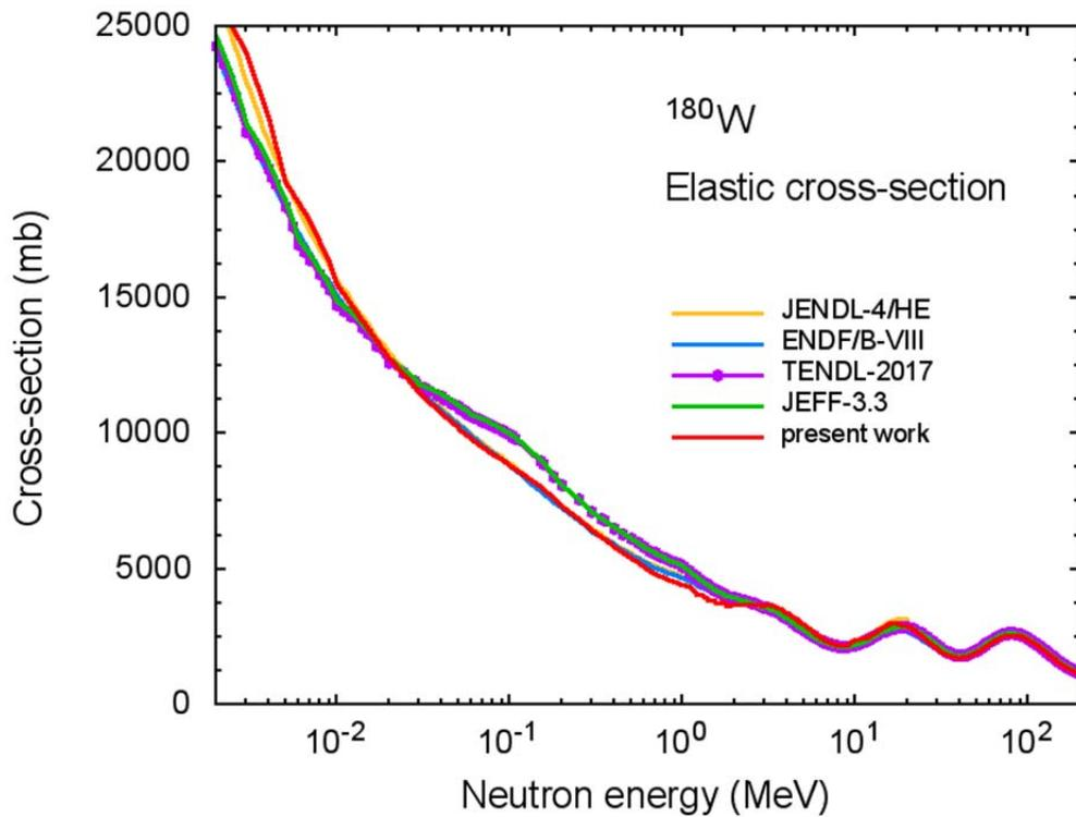
Fig.3 Cross-section for elastic neutron scattering for  $^{180}\text{W}$  evaluated in the present work, measured data, and data taken from different libraries.
