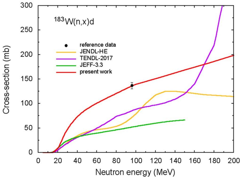
Fig.42 Deuteron production cross-section for  $^{183}\text{W}$ .
