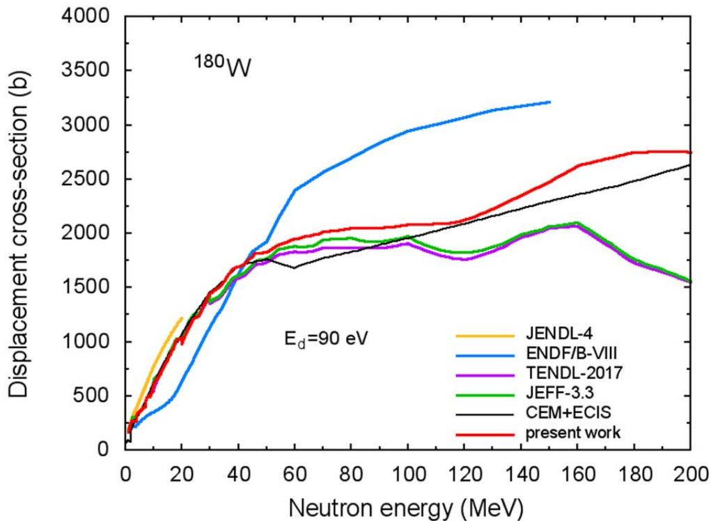
Fig.17 Atomic displacement cross-section for  $^{180}\text{W}$ .
