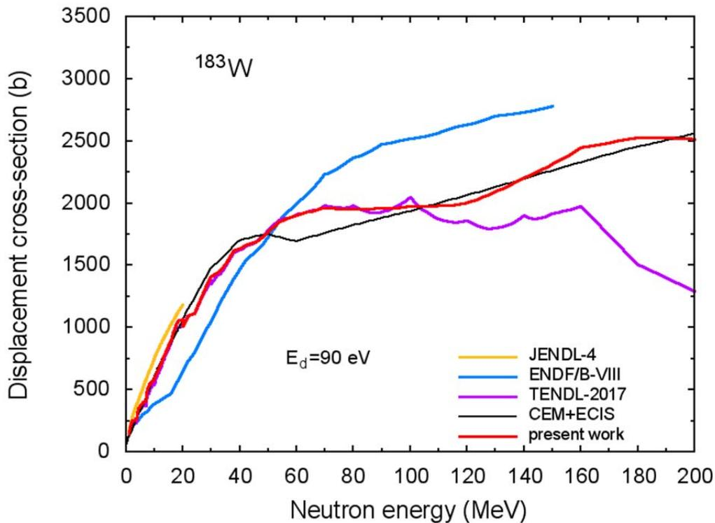
Fig.47 Atomic displacement cross-section for  $^{183}\text{W}$ .
