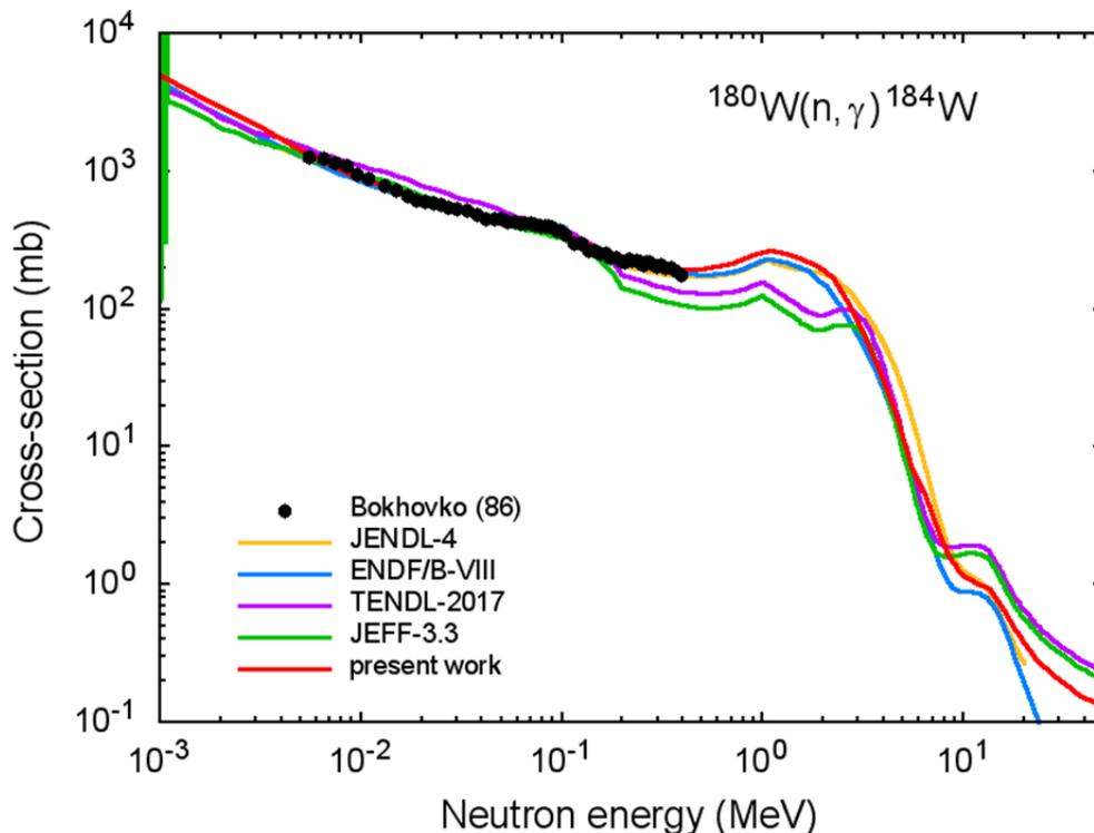
Fig.5 (n,γ) reaction cross-section for  $^{180}\text{W}$ .
