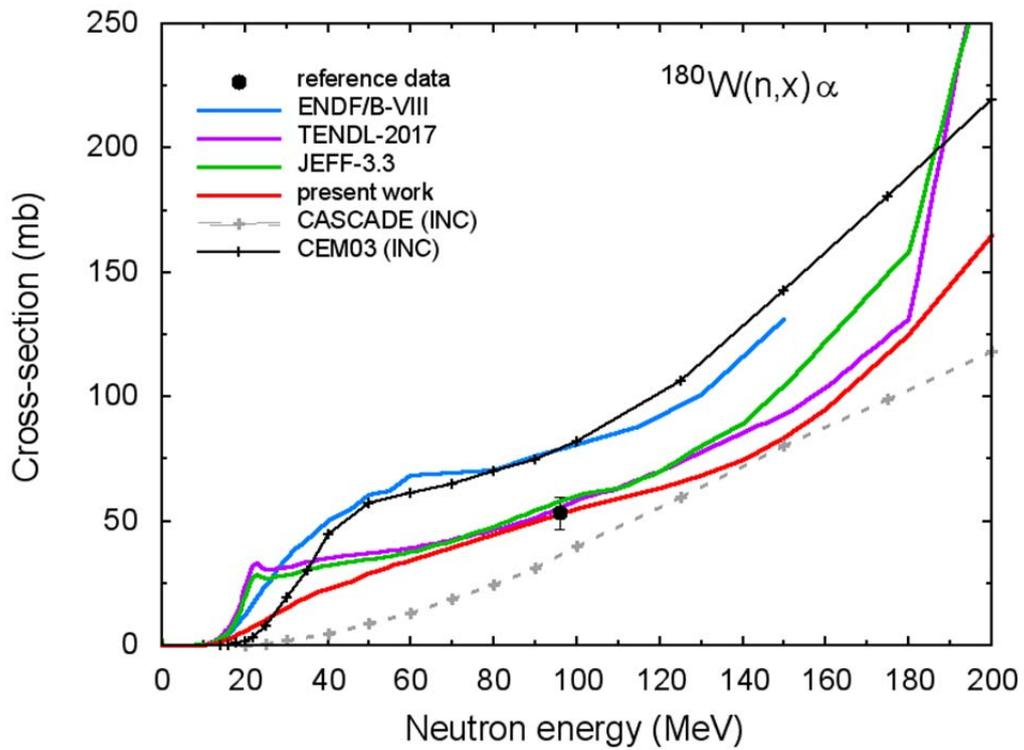
Fig.16  $\alpha$ -particle production cross-section for  $^{180}\text{W}$ .
