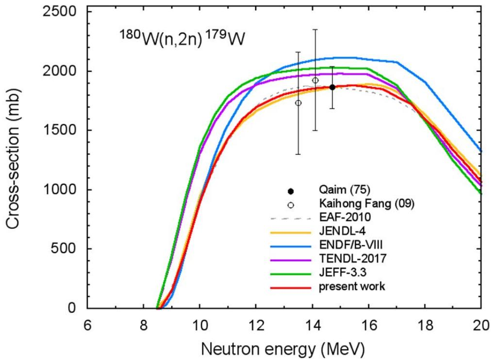
Fig.6 (n,2n) reaction cross-section for  $^{180}\text{W}$  equal to the sum of  $^{179g}\text{W}$  and  $^{179m}\text{W}$  production cross-sections.
