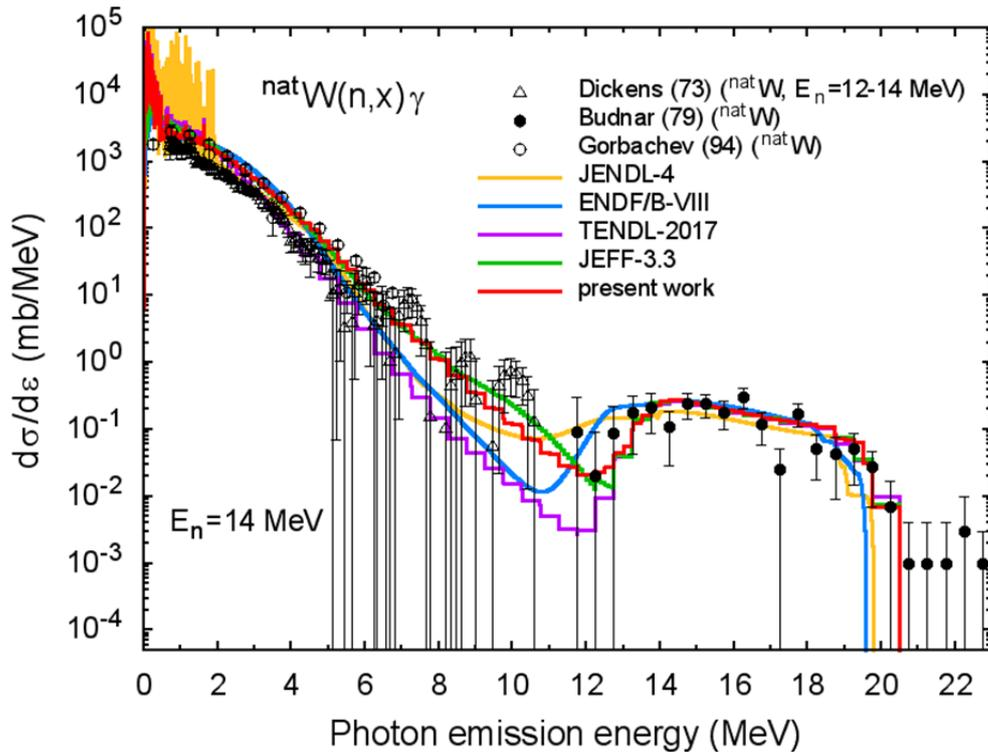
Fig.39 Photon energy distributions for irradiation of natural tungsten with 14 MeV neutrons. The values marked as "present work" are obtained using data for stable tungsten isotopes:  $^{180}\text{W}$  (this work),  $^{182}\text{W}$  [1],  $^{183}\text{W}$  (this work),  $^{184}\text{W}$  [77], and  $^{186}\text{W}$  [1].
