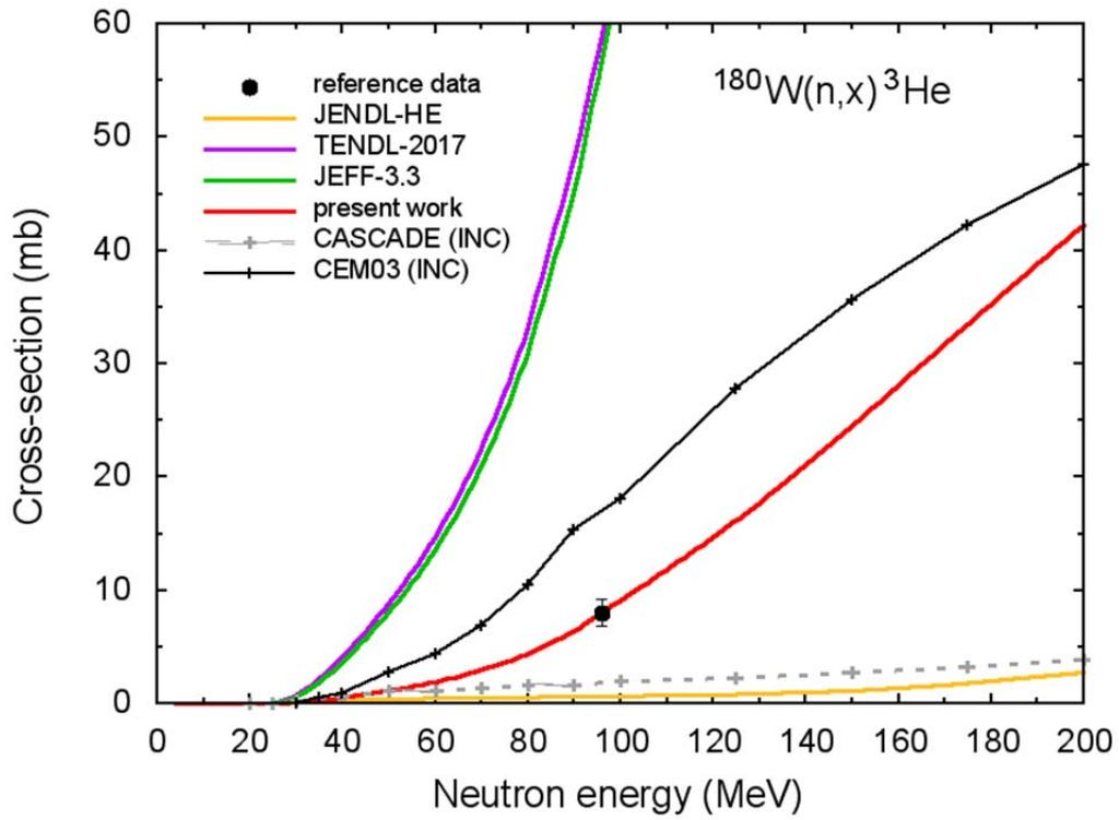
Fig.15  $^3\text{He}$  production cross-section for  $^{180}\text{W}$ .
