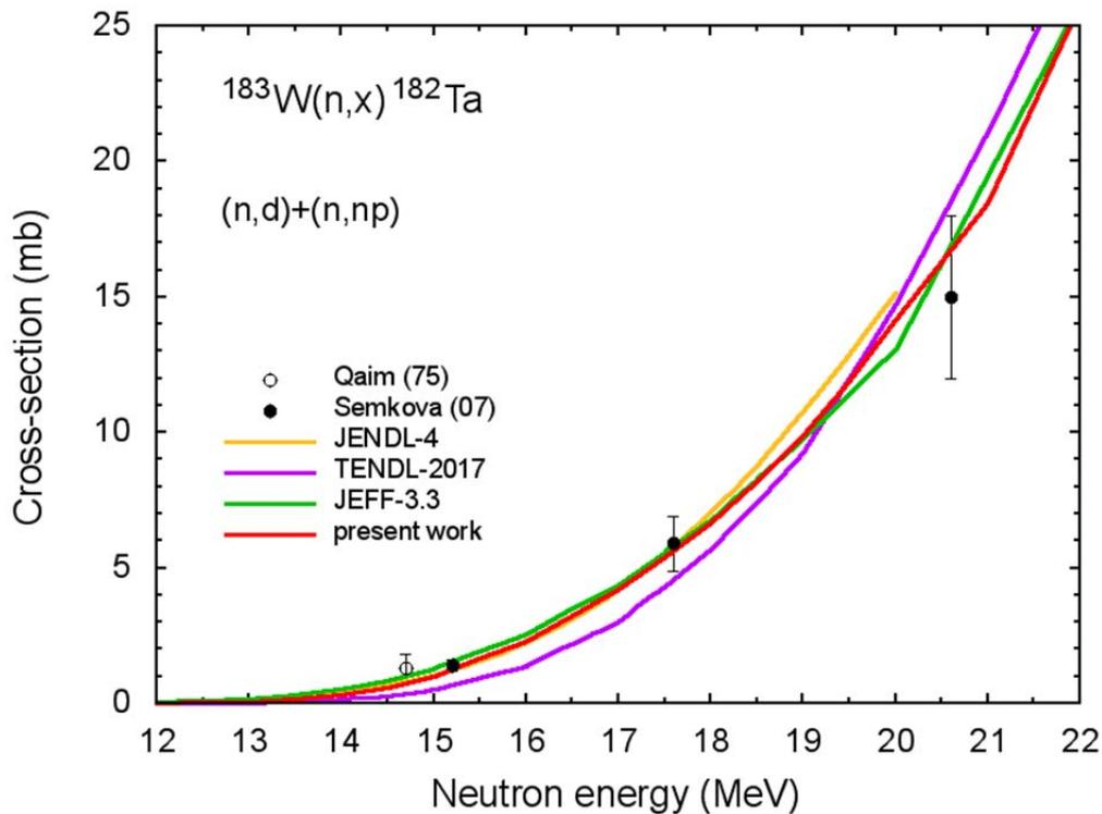
Fig.34 Sum of (n,d) and (n,np) reaction cross-section for  $^{183}\text{W}$ .
