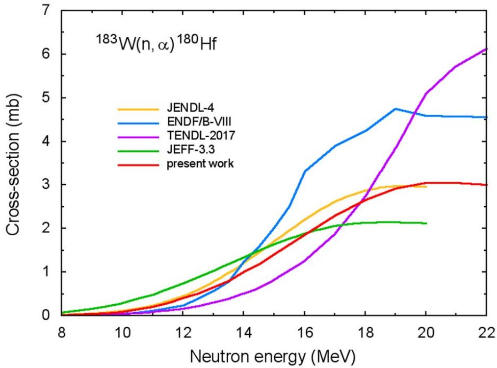
Fig.32 (n,α) reaction cross-section for  $^{183}\text{W}$ .
