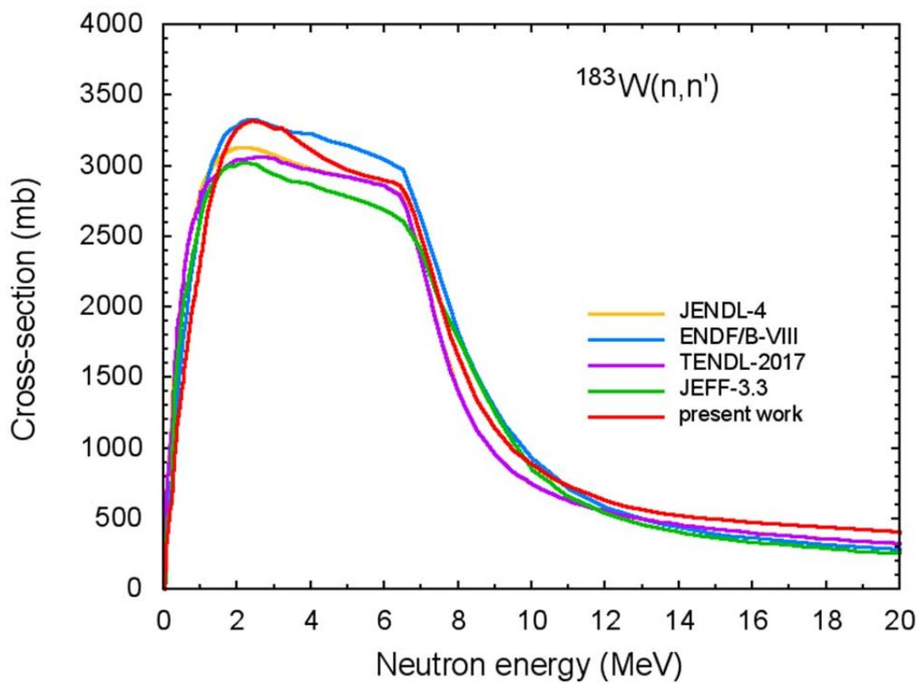
Fig.27 Inelastic scattering cross-section  $^{183}\text{W}(n,n')$ .
