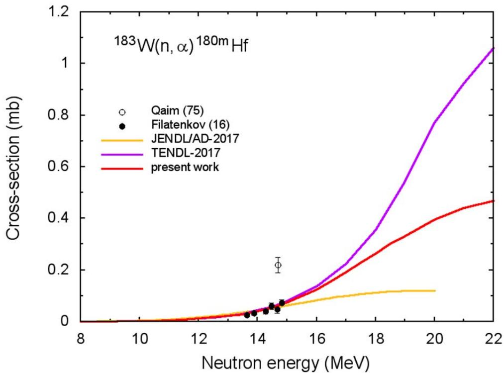
Fig.33 (n,α) reaction cross-section for  $^{183}\text{W}$  with production of  $^{180}\text{Hf}$  in the metastable state.
