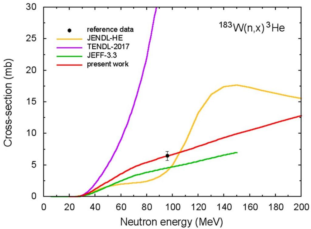
Fig.44  $^3\text{He}$  production cross-section for  $^{183}\text{W}$ .
