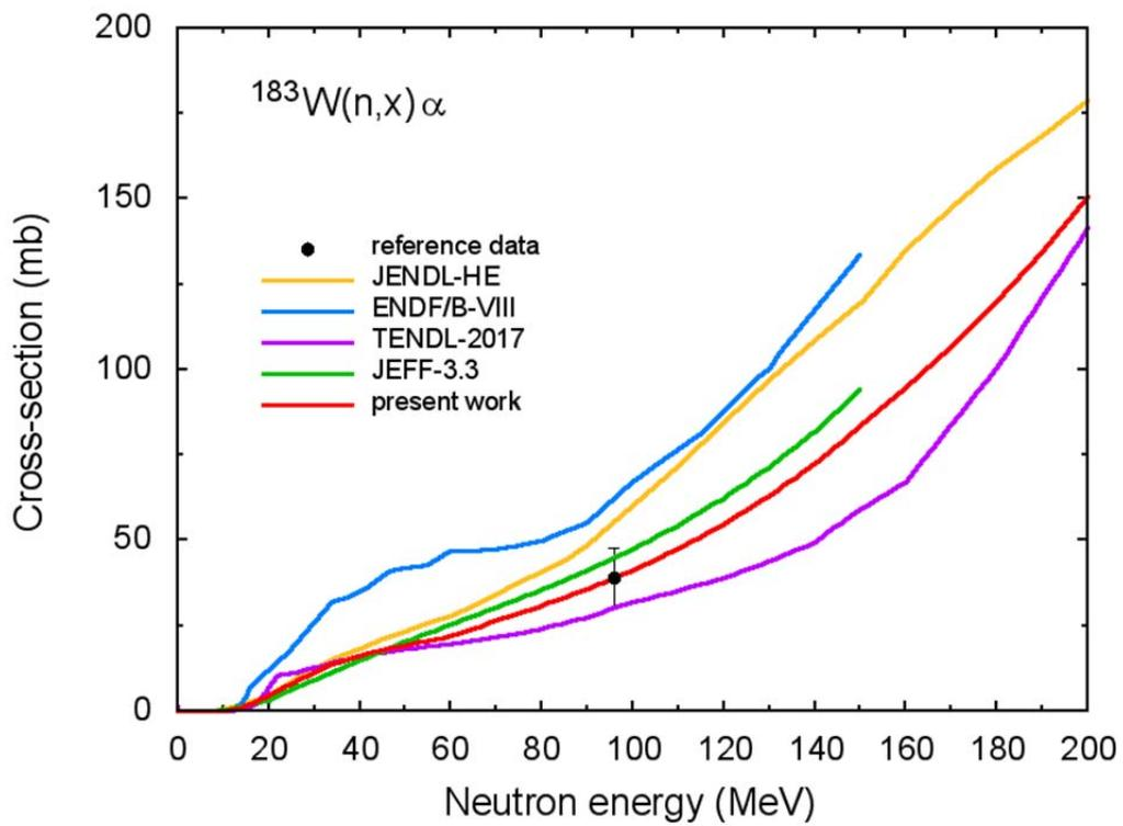
Fig.45  $\alpha$ -particle production cross-section for  $^{183}\text{W}$ .
