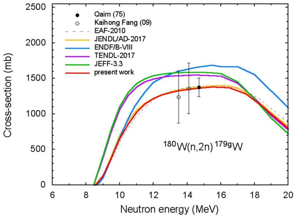
Fig.7 (n,2n) reaction cross-section for  $^{180}\text{W}$  with the production of  $^{179g}\text{W}$  in the ground state.
