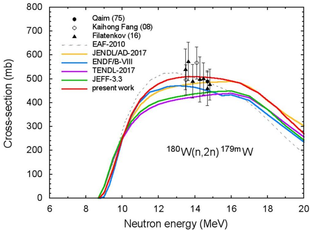
Fig.8 (n,2n) reaction cross-section for  $^{180}\text{W}$  with the production of  $^{179\text{m}}\text{W}$  in the metastable state ( $T_{1/2} = 6.4$  m).
