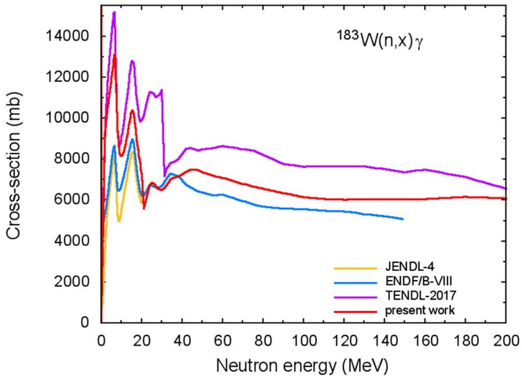
Fig.46 Photon production cross-section for  $^{183}\text{W}$ .
