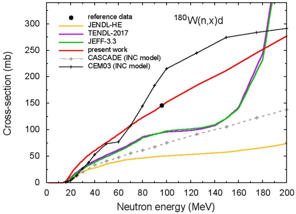
Fig.13 Deuteron production cross-section for  $^{180}\text{W}$ .
