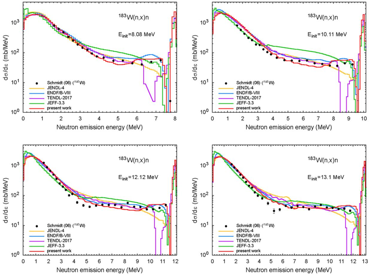
Fig.35 Neutron energy distributions for  $n+^{183}\text{W}$  reactions at different incident energies
