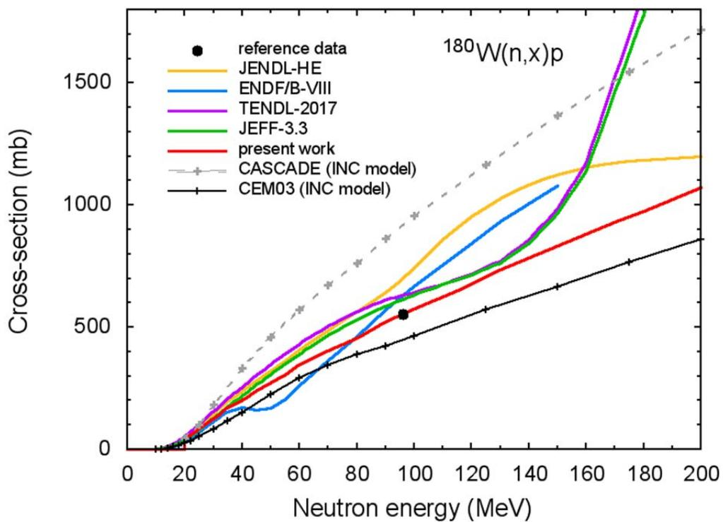
Fig.12 Proton production cross-section for  $^{180}\text{W}$ .
