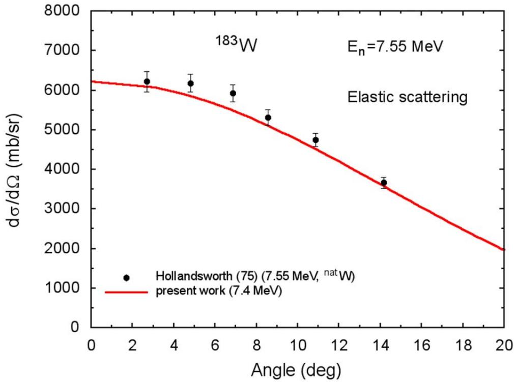
Fig.24 Elastic scattering angular distribution of neutrons for  $^{183}\text{W}$  irradiated with 7.55 MeV neutrons.
