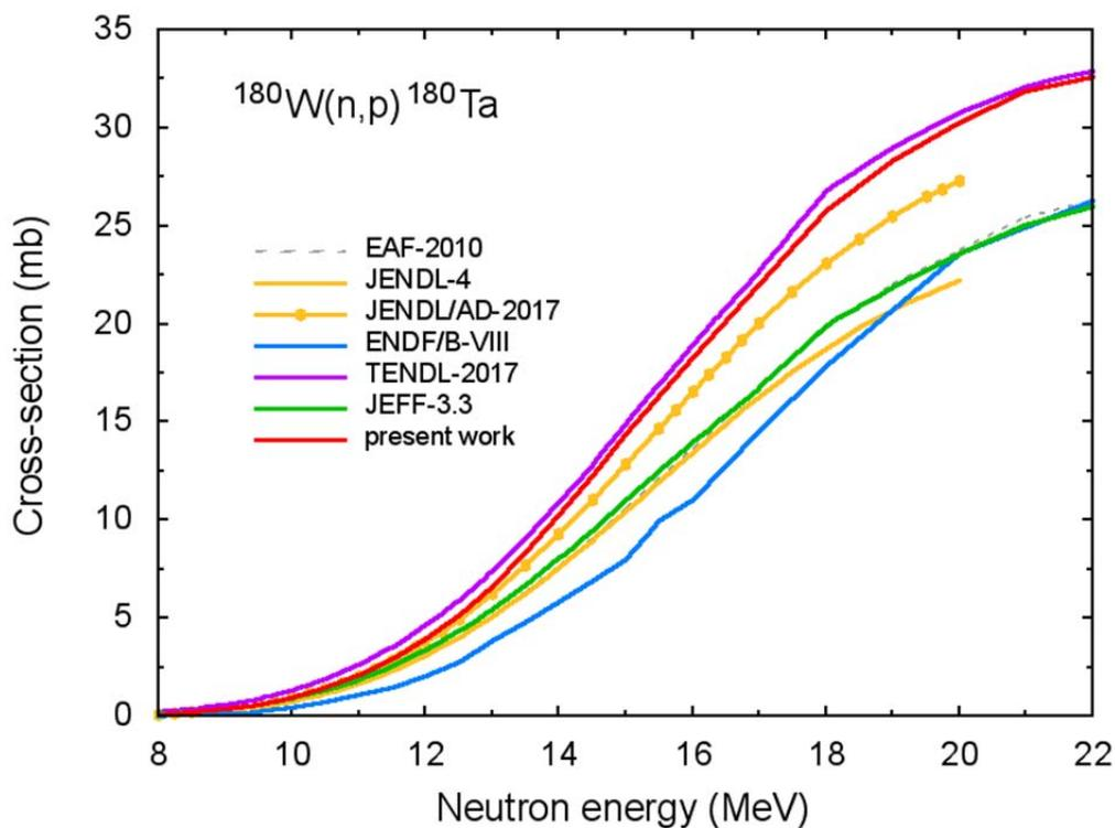
Fig.9 (n,p) reaction cross-section for  $^{180}\text{W}$  equal to the sum of  $^{180\text{g}}\text{Ta}$  and  $^{180\text{9m}}\text{Ta}$  production cross-sections.
