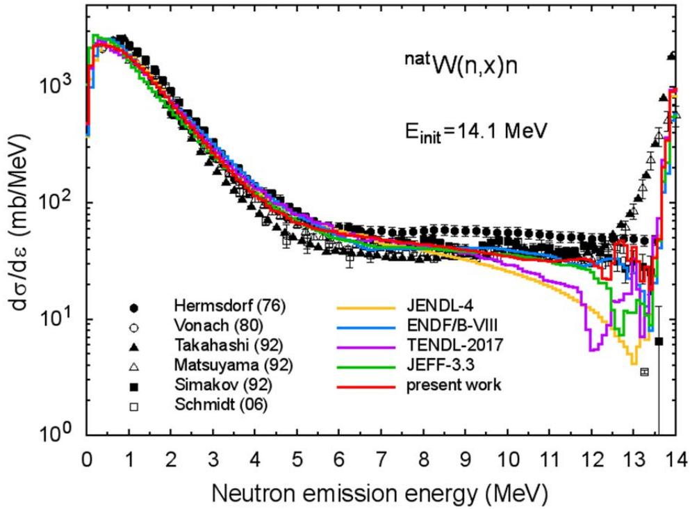
Fig.37 Neutron energy distributions for irradiation of natural tungsten with 14.1 MeV neutrons. The values marked as "present work" are obtained using data for stable tungsten isotopes:  $^{180}\text{W}$  (this work),  $^{182}\text{W}$  [1],  $^{183}\text{W}$  (this work),  $^{184}\text{W}$  [77], and  $^{186}\text{W}$  [1].
