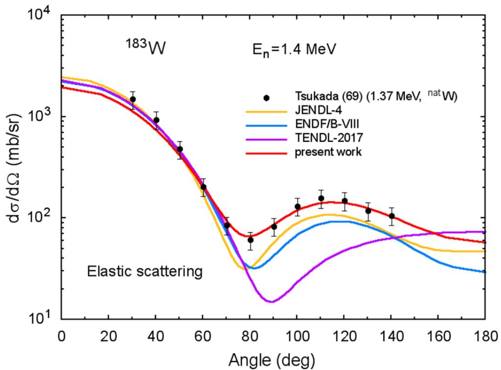
Fig.21 Elastic scattering angular distribution of neutrons for  $^{183}\text{W}$  irradiated with 1.4 MeV neutrons.
