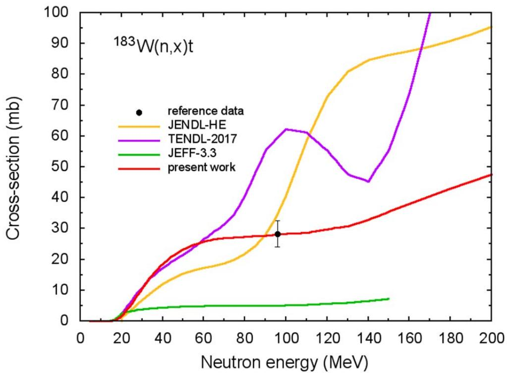
Fig.43 Triton production cross-section for  $^{183}\text{W}$ .
