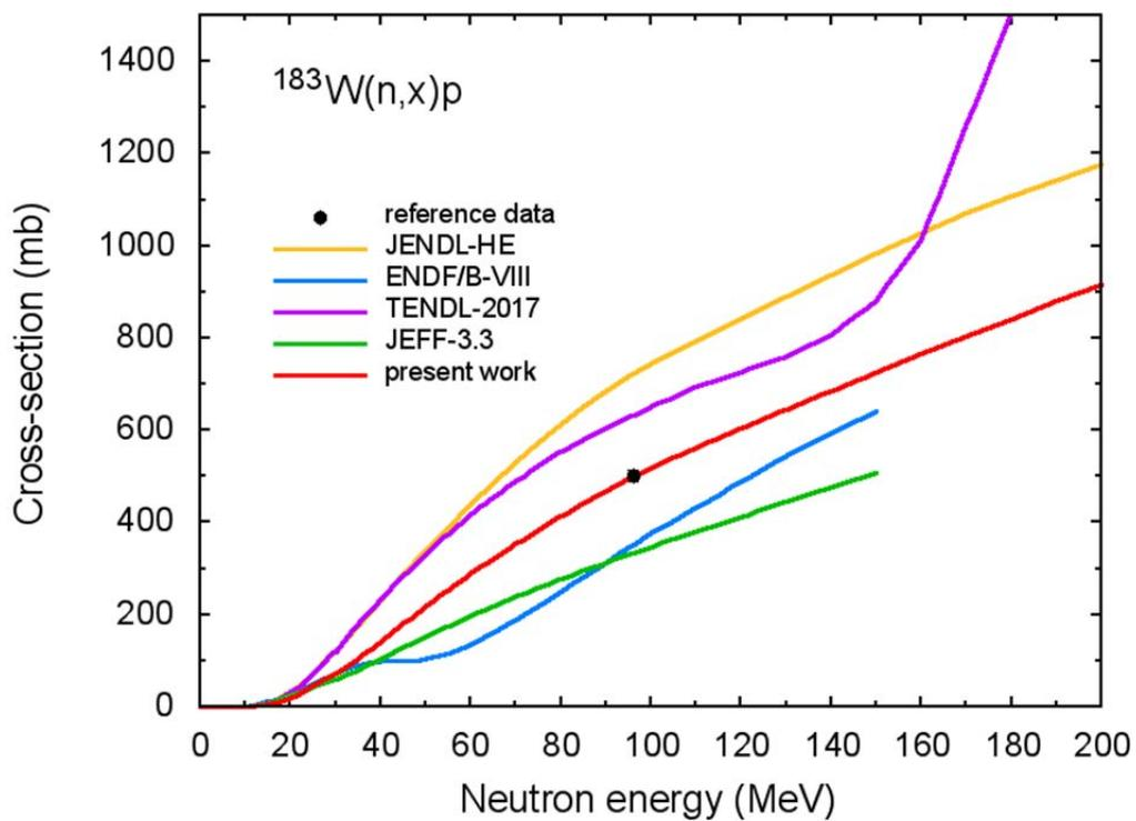
Fig.41 Proton production cross-section for  $^{183}\text{W}$ .
