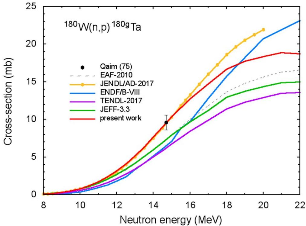
Fig.10 (n,p) reaction cross-section for  $^{180}\text{W}$  with the production of  $^{180}\text{Ta}$  in the ground state.
