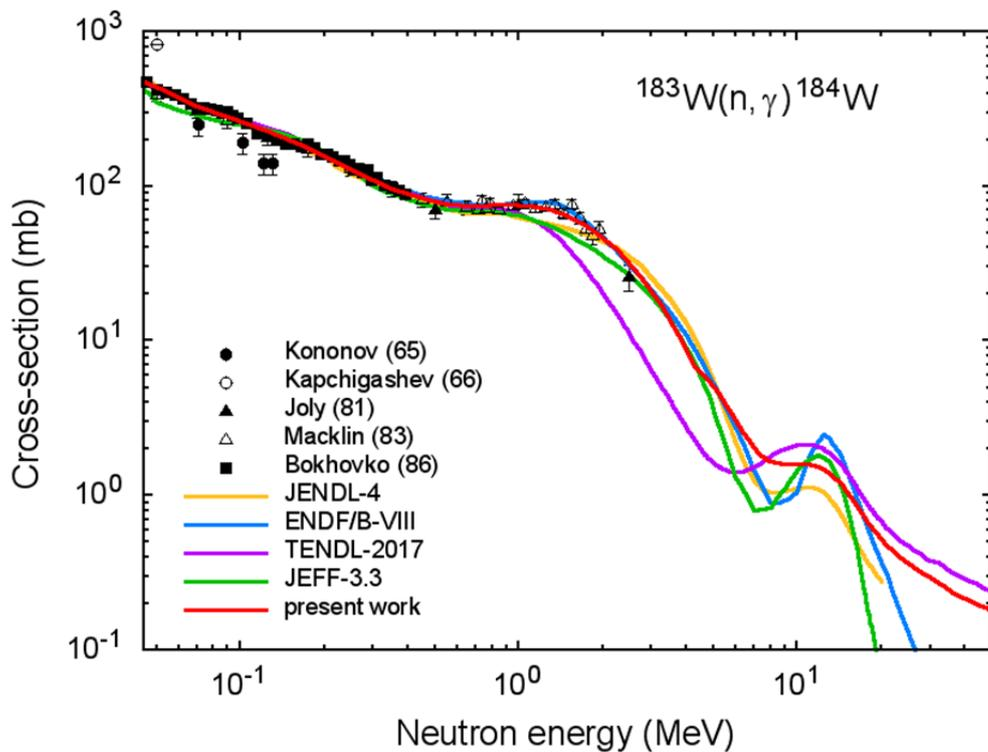
Fig.29  $(n,\gamma)$  reaction cross-section for  $^{183}\text{W}$ .
