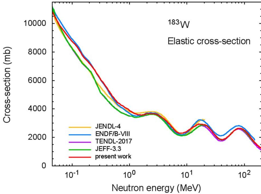
Fig.20 Elastic cross-section for neutron irradiation of  $^{183}\text{W}$ .
