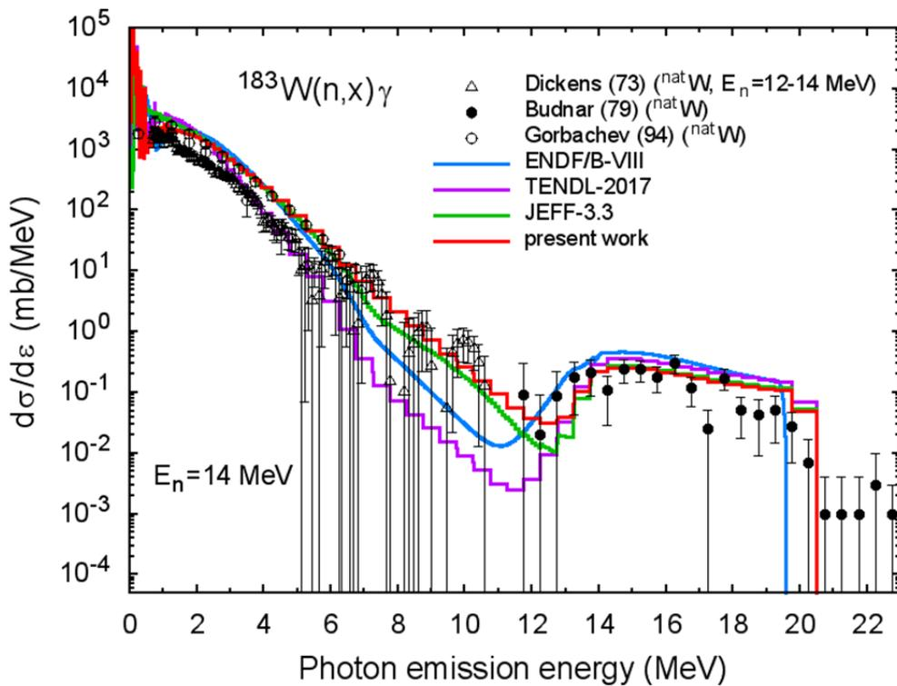
Fig.38 Photon energy distribution for  $n+^{183}\text{W}$  reactions at 14 MeV neutron energy.
