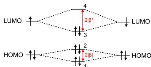
**Scheme 1.** Orbital correlation diagram from TCNQ anion-radicals to  $(TCNQ)_2^{2-}$  showing the dimer level splitting  $2|\beta|$  and  $2|\beta^*|$  for the HOMO- and LUMO-derived dimer orbitals, respectively. LUMO becomes SOMO when it is singly occupied. Orbital No 3 is the bonding combination of the two SOMO orbitals.<sup>[11]</sup>
