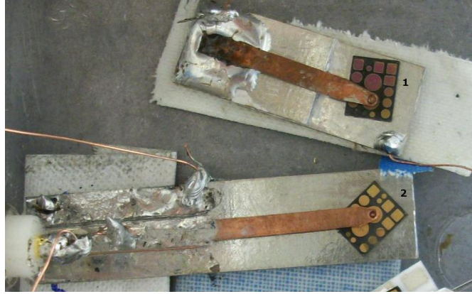
Fig.84 – Photo of the thermal treated wafer with purple surface on the metallic contact (denoted with 1 ) and of the not heated SiC wafer (denoted with 2 ). Both wafers are attached to a conductive plate with a spring contact. The plate and the spring are electrically isolated from each other.
