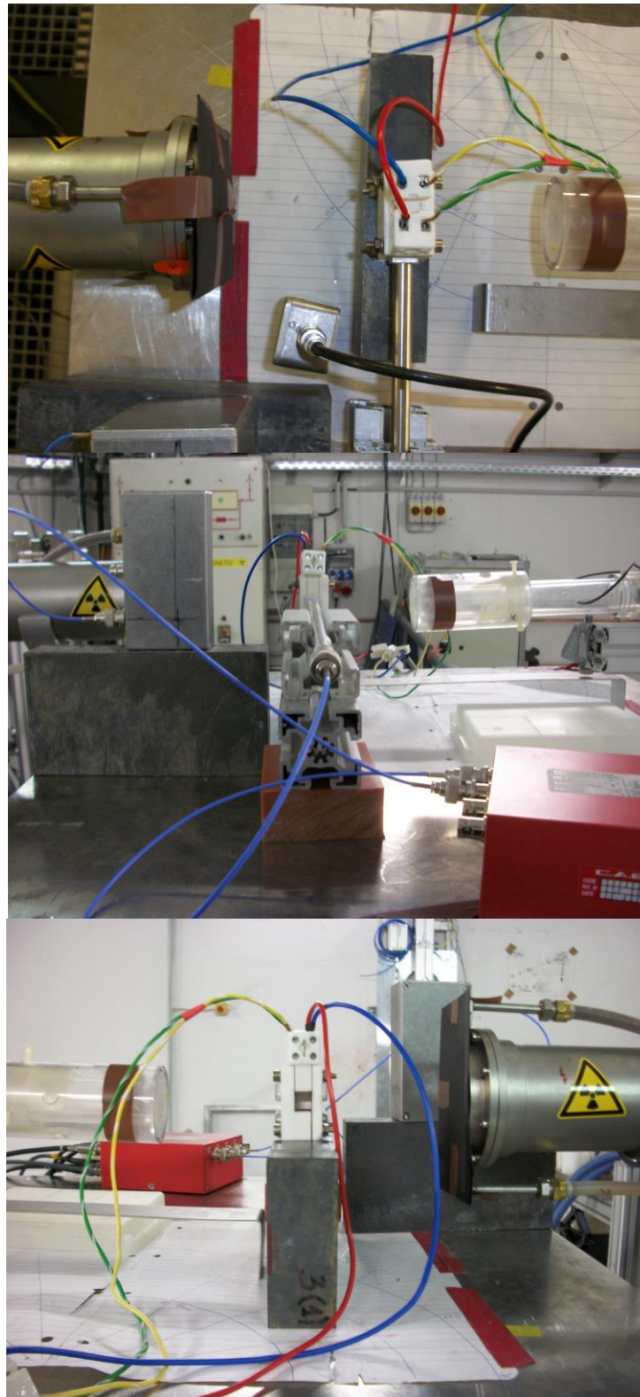
Set-up arrangement for fast neutron measurements at high temperatures up to 500 °C, a- Tritium target and macor housing from above, b- CEAN preamplifier attached to the 50 Ohm stainless steel coaxial cable through a coaxial connector, c- Tritium target, macor housing and CAEN preamplifier from the side
