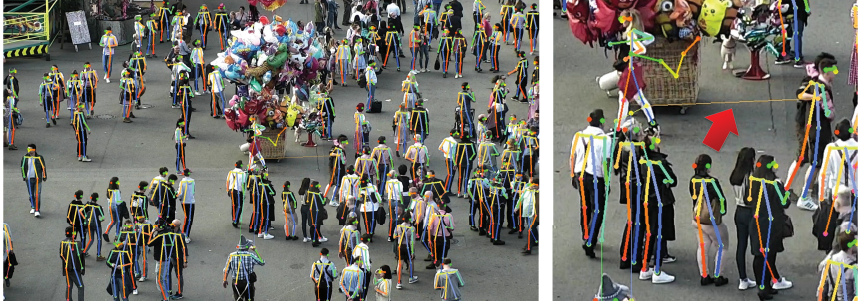
Figure 4.2: Exemplary result generated with AlphaPose. On the the first glance, the left side shows promising results. The right part shows a central patch taken from the left image. The red arrow indicates a wrong connection between key points of different persons, which is just one of multiple wrong poses within the patch.
