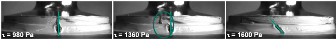
Figure 2.5: Cutouts from video recordings at varying shear stress. Here using the example of paste A measured with plate roughness R_q = 2-4 \mu m .
