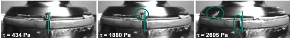
Figure 2.6: Cutouts from video recordings at varying shear stress. Here using the example of paste A measured with plate roughness R_q = 9 \mu m .
