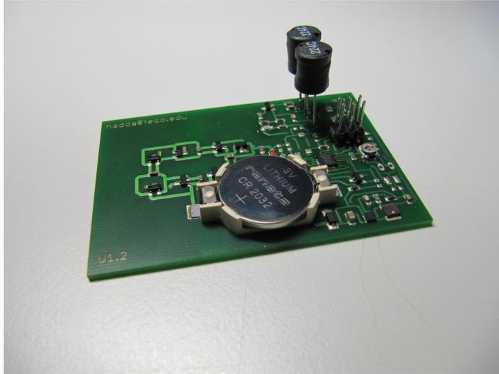
(A) Si-based transponder, a replacement for an organic and printed transponder.
