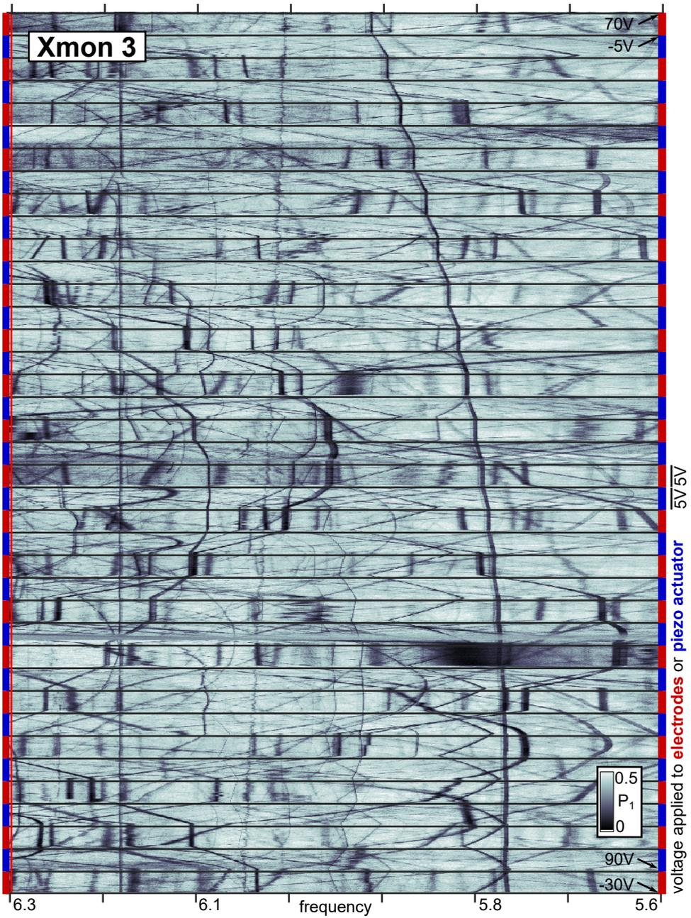
**Figure D.4:** Raw data recorded with Xmon 3 using the swap-spectroscopy protocol ( $\tau = 5\mu\text{s}$ ). The red line ( $\sim 6.3\text{GHz}$ ) is the qubit frequency at zero applied magnetic flux.
