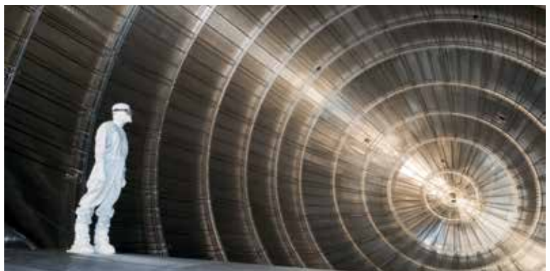
A view of the wire electrode system lining the interior walls of the vacuum vessel of the KATRIN main spectrometer. (Photo: Michael Zacher, KATRIN Collaboration)
