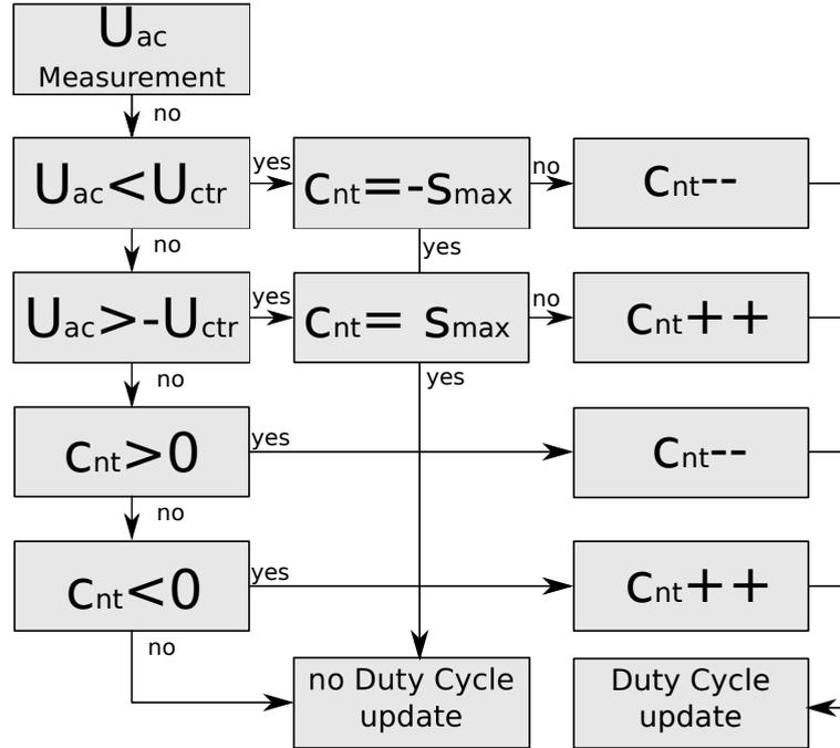
Figure 72: Determination algorithm for the grid voltage polarity, represented in the count variable  $c_{nt}$ .
