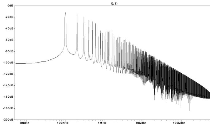
Figure 69: SLC inductor current FFT at  $f_{sw} = 100\text{kHz}$  and  $D = 0.3$ .
