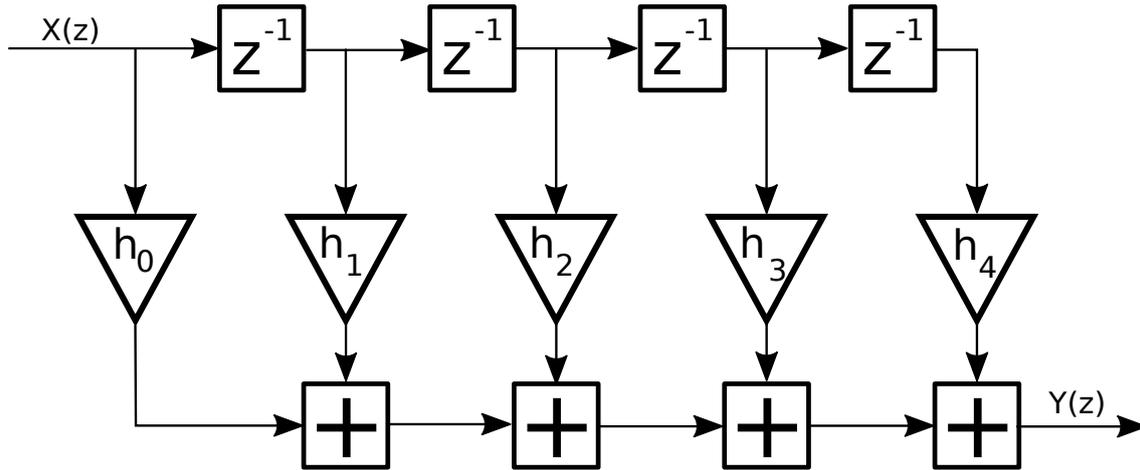
Figure 86: A fourth order FIR filter topology is shown: Every sample is multiplied with a weighting factor and is then delayed by one cycle.
