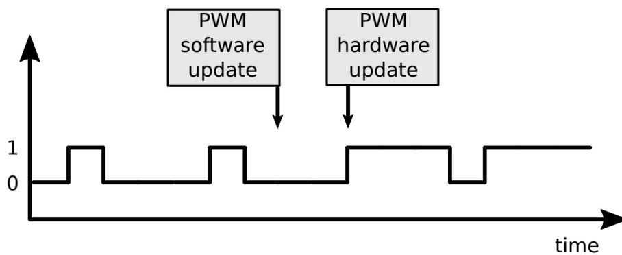
(b) First one waveform is fully issued, then the next waveform is transmitted.
