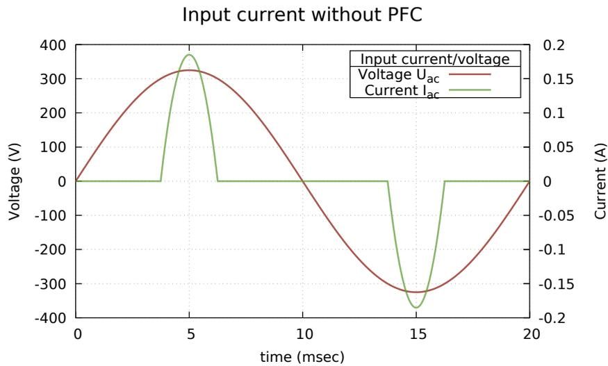
Figure 33: Without an PFC, AC current is only taken from the grid at peak values. Therefore, a relatively high current flows when the grid voltage peaks, otherwise no current is taken from the grid. This introduces reactive power, resulting in a low power factor. The actual current shape may differ from load to load. This Figure as only an illustration of a possible grid current caused by a full bridge rectifier.
