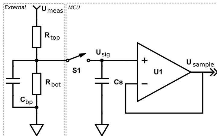
Figure 76: Direct drive of ADC using a resistive divider.
