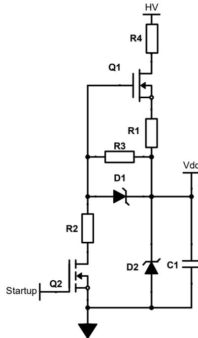
Figure 93: The startup circuit consists of a constant current depletion mosfet Q2 that charges the capacitor C1. A zener/TVS diode is used to limited the maximal voltage for the downstream buck converter.
