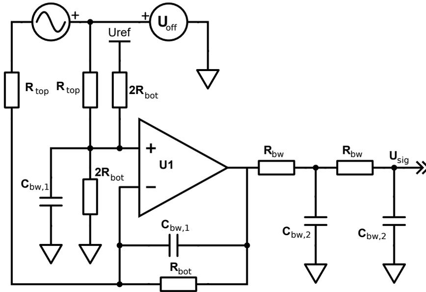
Figure 81: Differential quasi isolated high voltage current sense circuit.
