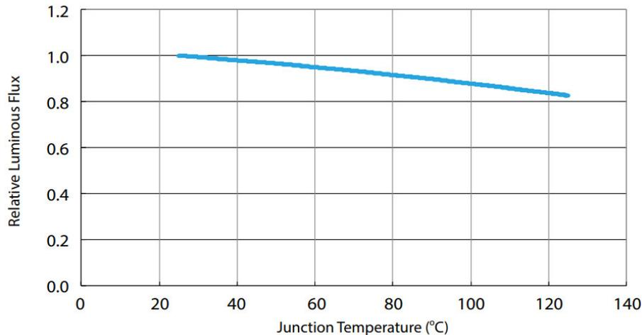
Figure 7: The light output of LEDs decreases with the increase of temperature. Exemplary data of the Edison 2835 LED is shown [5].
