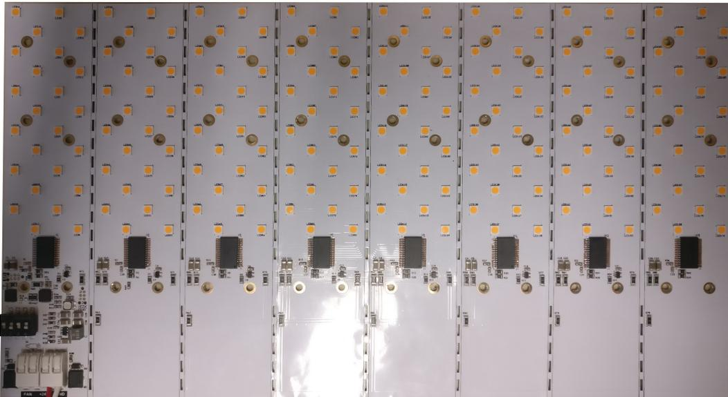
Figure 12: This LED engine is used in LED street light luminaries. It may be directly touched, as safety extra low voltage (SELV) below 60 V is used. Hence, this PCB is inherently safe.
