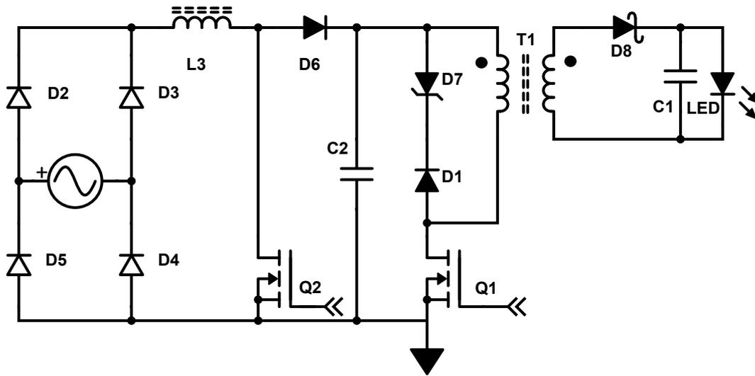
Figure 36: PFC/Flyback topology consists out of a standard PFC with a downstream flyback converter.
