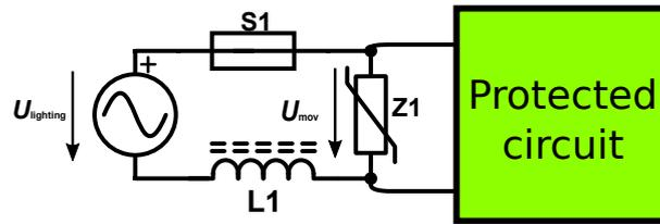
Figure 63: A metal oxide varistor  $Z_1$  is placed directly after the fuse to absorb incoming overvoltage. The subsequent circuits are protected by the metal oxide varistor.
