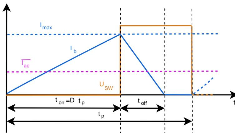
Figure 65: The boost converter waveform shows the three time steps  $t_{on}$ ,  $t_{off}$  and  $t_p$  of the boost PFC converter.
