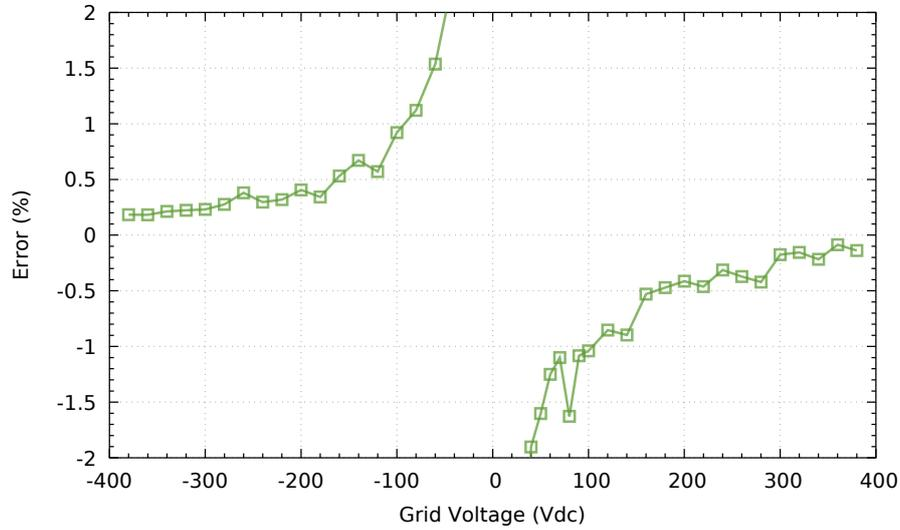
(b) Relative AC voltage measurement error.
