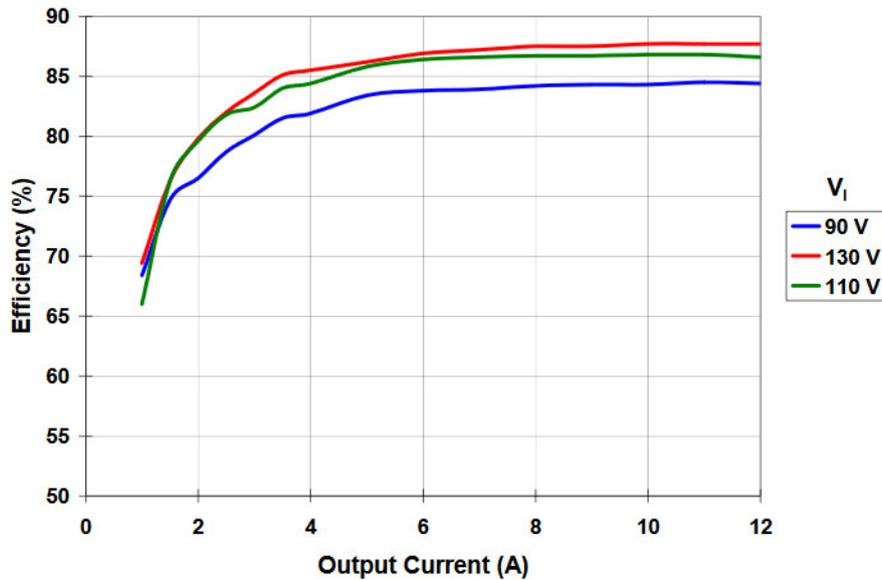
Figure 37: Efficiency of a flyback converter used for LED TVs. The efficiency increases with increasing output power. The higher the input voltage, the higher the efficiency. The measurement is reproduced from the reference design [8].
