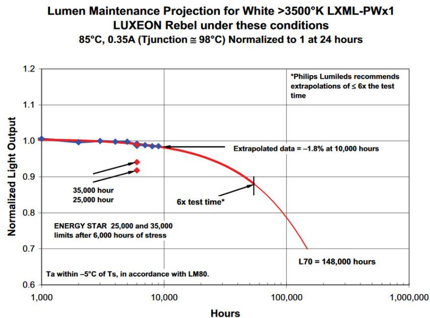
Figure 8: Lifetime of LEDs at high temperature operating conditions, based on a Lumileds study[6].
