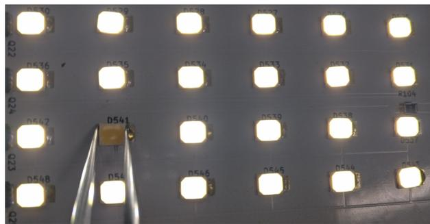
Figure 53: A short circuit of a LED is compensated without affecting the LED drive current of the other LEDs in the string.
