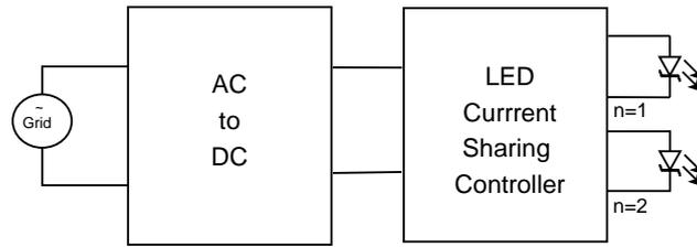
Figure 42: Generic LED driver topology for paralleling LED strings.
