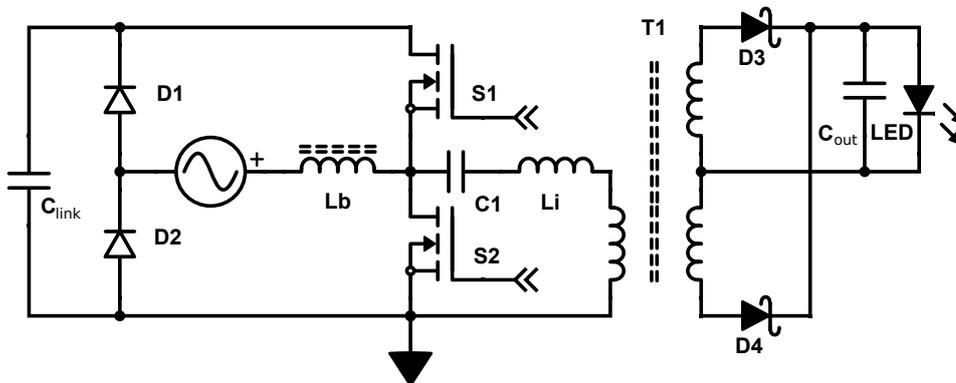
Figure 41: Integrated PFC/SLC converter: The boost stage and the SLCC share the switchnode.
