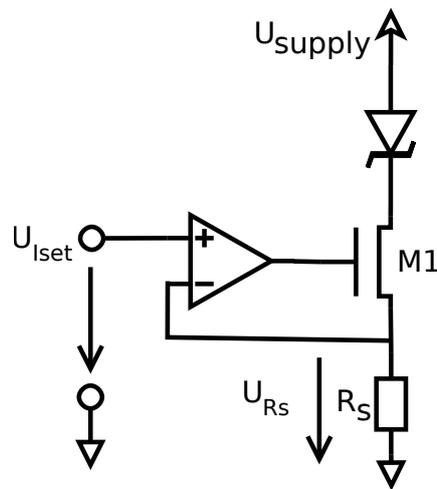
Figure 19: Simplified LED driver implemented using an operational amplifier, mosfet and sense resistor.
