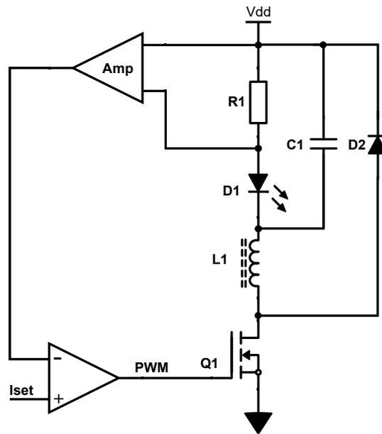
Figure 28: Hysteresis mode controller implementation: The LED current is measured by means of the sense resistor R1. The current sense voltage is amplified and passed to the hysteresis comparator that switches on when the minimum threshold is reached and switches off when the maximum threshold is reached.
