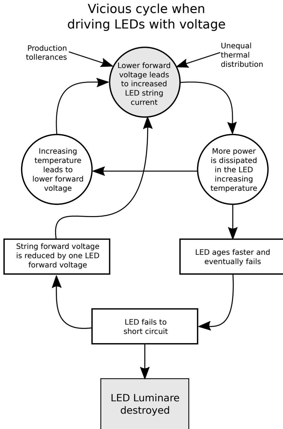
Figure 11: A vicious cycle when driving LEDs with a constant voltage can be observed due to their exponential current characteristic. In the best case, lifetime is reduced, in the worst case the LEDs are destroyed.
