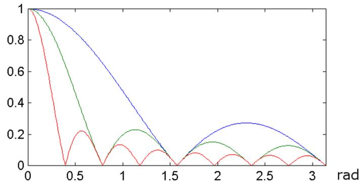
Figure 85: Low pass characteristic of a sinc filter for averages of 16 (red), 8 (green), and 4 (blue), based on [11].
