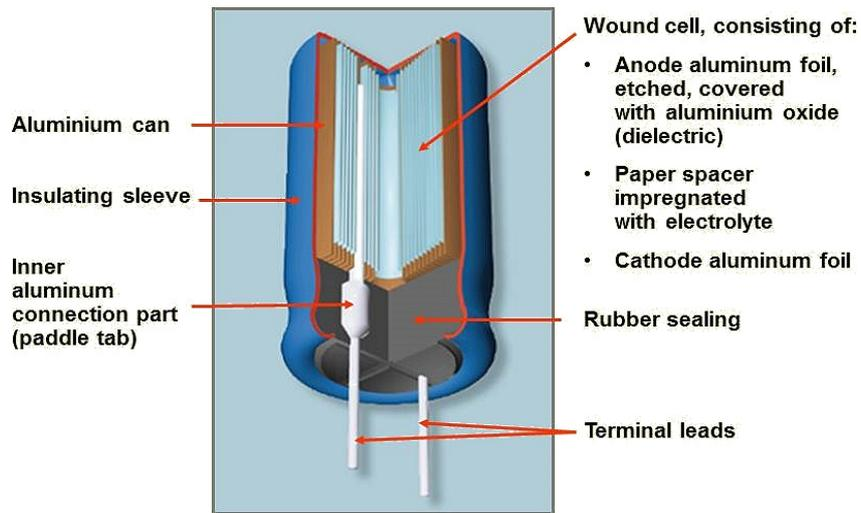
Figure 60: Electrolytic capacitor construction. Public domain graphics from Elcap.
