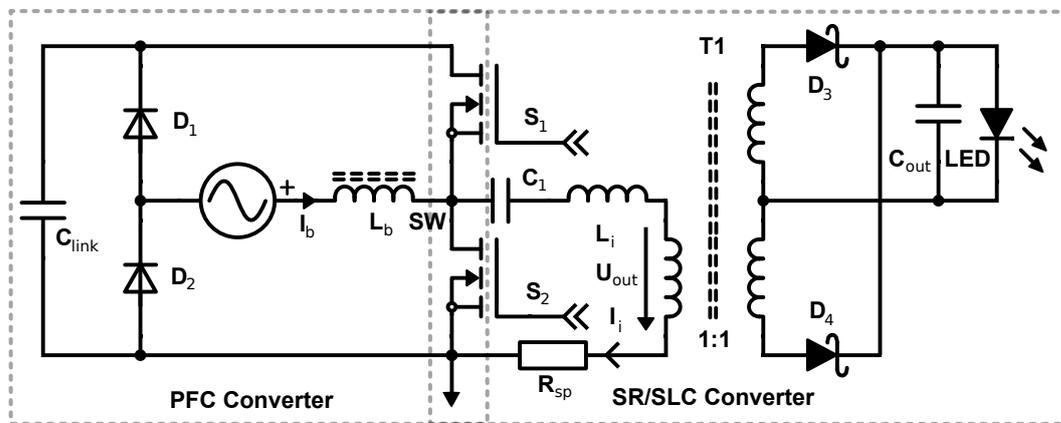
Figure 89: The SLCC current  $I_i$  is sensed by the shunt resistor  $R_{sp}$  that is connected to an overcurrent protection.
