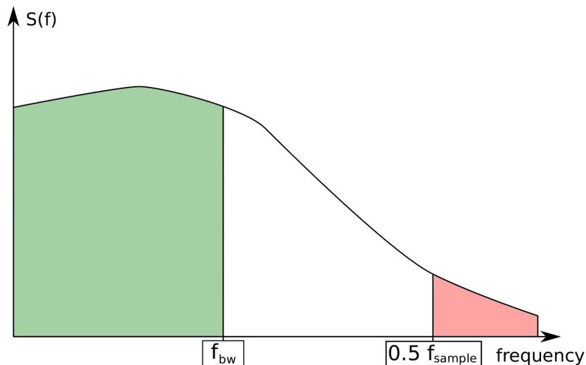
Figure 78: An arbitrary signal over the sampling frequency, based on [10, p. 70], is depicted. The green area is the signal part, the red area would introduce anti-aliasing noise. Hence, for a good reproduction a filter has to be designed that attenuates this aliasing noise.
