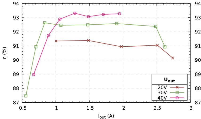
Figure 124: Efficiency of the PFC/SLC converter over output current.
