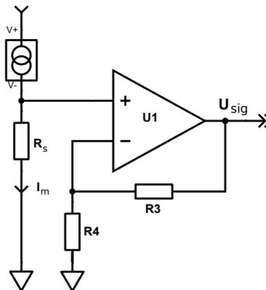
Figure 79: Standard op-amp current shunt amplifier without offset generation.
