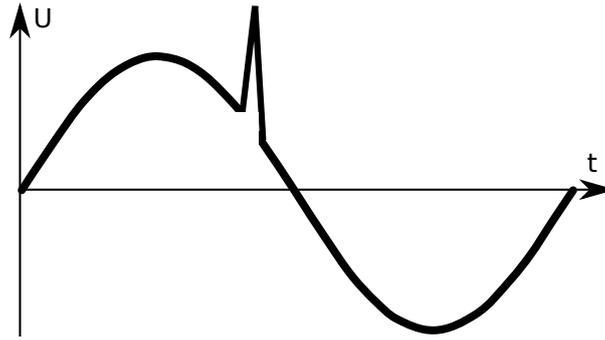
Figure 62: Example of a surge on a sinusoidal voltage.
