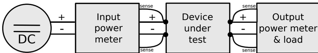
Figure 112: Measurement setup
