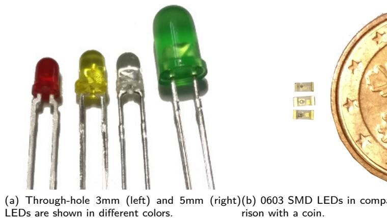
Figure 3: Indicating LEDs are used for status indication, having low optical and electrical power. They are available in through hole and surface mount technology.
