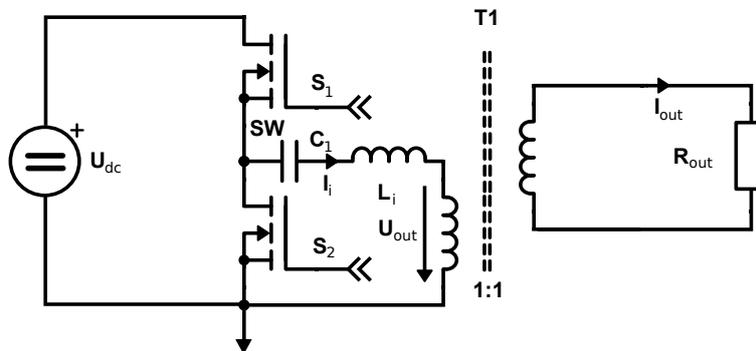
Figure 67: The SLCs output rectifier and capacitor are replaced by a load resistor for FHA.
