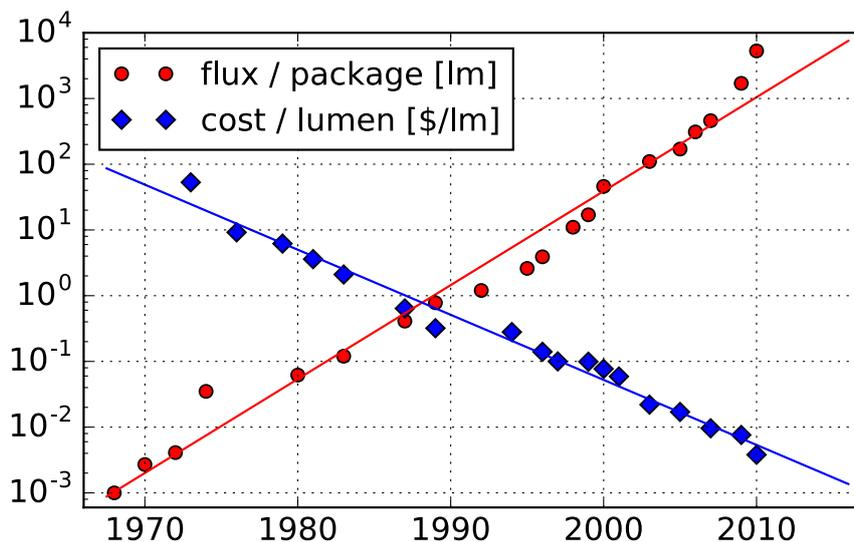
Figure 1: The Haitz law claims that the power per package increases by a factor of 20 every ten years, while the cost per lumen reduces by a factor of ten. [1, 2, 3] (Image Source: Wikimedia Commons)
