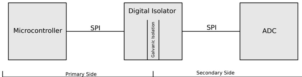
Figure 84: The MCU requests data over the digitally isolated SPI bus from the secondary side ADC.
