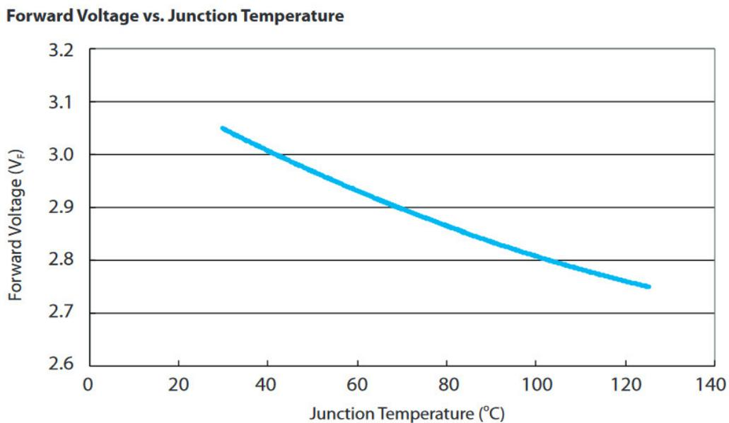
Figure 10: Temperature dependence of the forward voltage over the temperature for the Edison 2835 LED is shown [5]. The higher the LED junction temperature, the lower is its forward voltage.
