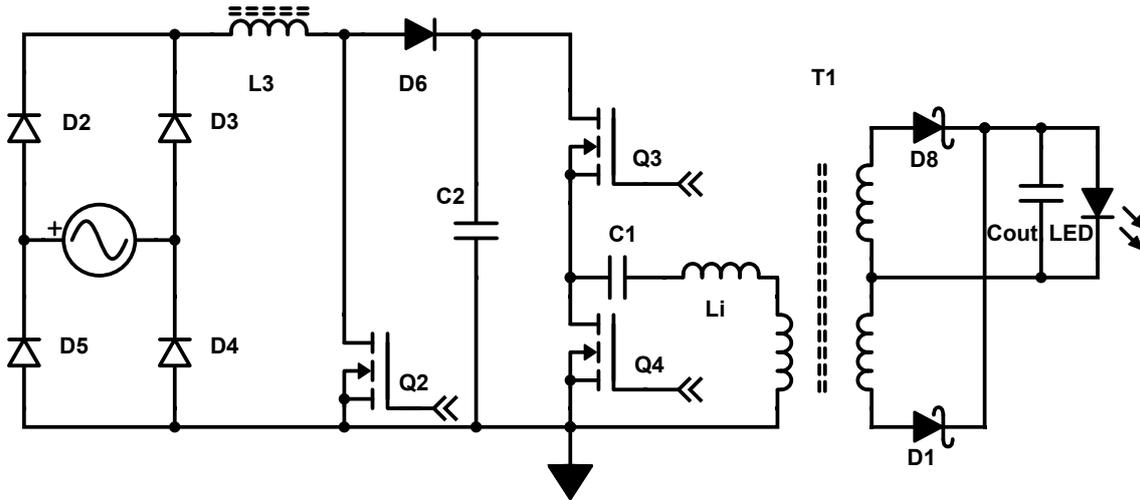
Figure 38: Series resonant converter with a standard boost PFC: Q2 is used to control the input current from the grid, where as Q3/Q4 are driven with a constant duty-cycle of  $D=0.5$  and the frequency is changed.
