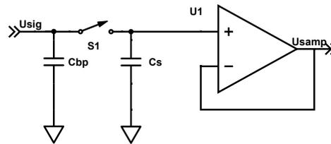
Figure 75: An additional bypass capacitor delivers the peak current required for charging the sampling capacitor.
