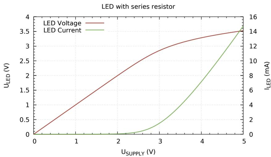
Figure 16: Characteristic curve of a LED driven by a series resistor. A sweep of the DC voltage shows that the current increases approximately linear when the supply voltage is larger than the typical LED forward voltage. This example shows a spice simulation, of the LED 'NSCW100' and a series resistor  $R_{LED} = 100 \Omega$ .
