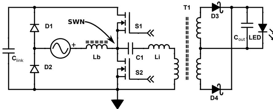
Figure 21: The switchnode (SWN) of the Series LC converter is between the two mosfets S1 and S2.
