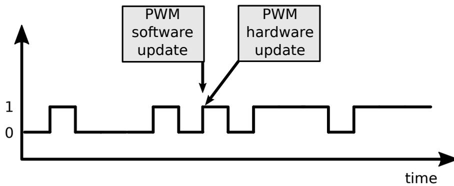
(a) Distorted waveform due to asynchronous write to the PWM register
