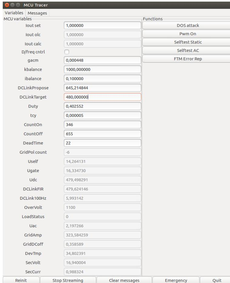
Figure 104: The MCU Tracer can be used to read data from the MCU. Data may be modified using the MCU Tracer. By this, parameters can be adjusted actively during software operation. Functions can be executed by clicking on the corresponding button.
