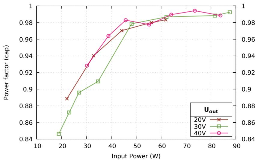
Figure 123: Power Factor of the PFC/SLC converter.
