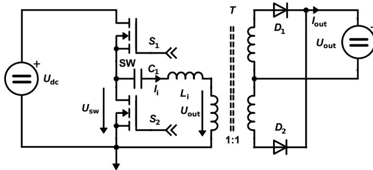
Figure 66: Series resonant converter topology.
