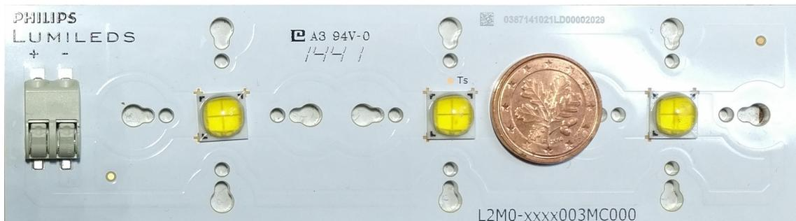
Figure 5: HighPower LED Module with three 10 W Luxeon-M LEDs. The PCB is produced by Philips and is available in a standardized format for easy deployment.
