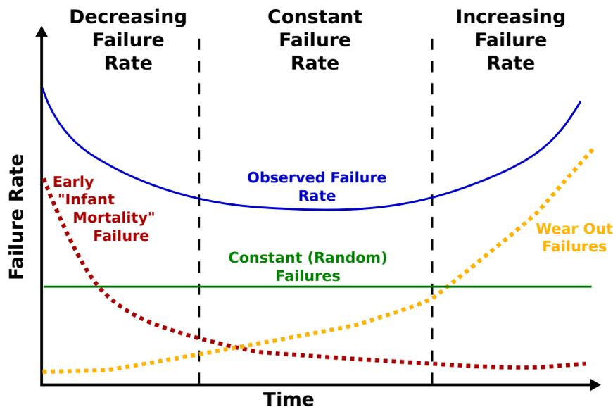
Figure 57: Bathtub curve with failure types. Image by the US Army, McSush.
