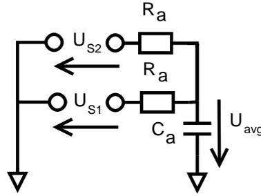
Figure 46: Averaging circuit determining the set current  $U_{Iset}$  using the individual sense voltages.
