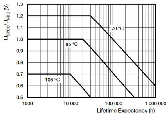
Figure 61: Lifetime of a film capacitor. Extracted from capacitor datasheet Vishay MKP1848.
