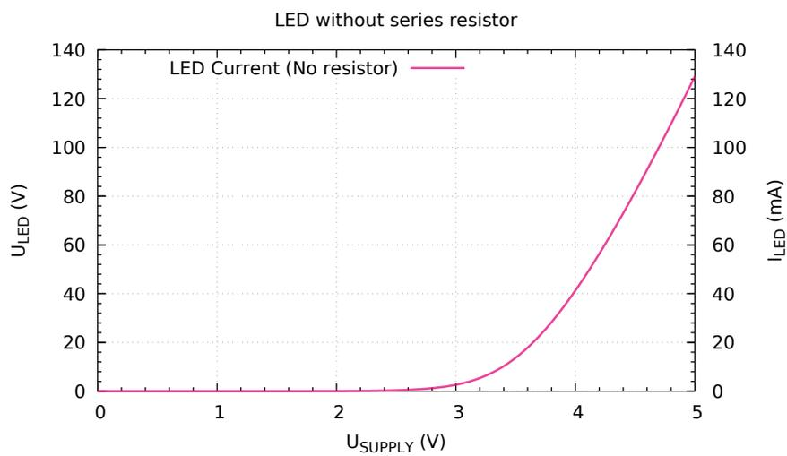
Figure 17: The LED current of the LED 'NSCW100' without series resistor is depicted for reference. Clearly, it can be observed that the LED output current rises exponentially at low voltage differentials.
