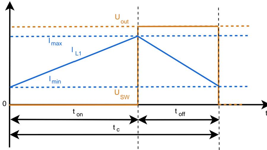
Figure 30: The Boost converter is operating in continuous mode and its operating waveform is shown. The inductor current  $I_B$  rises when the switch is closed to GND, thus  $U_{SW} = 0$ . When the switch opens, the inductor releases its energy to the output, supplying it with power.
