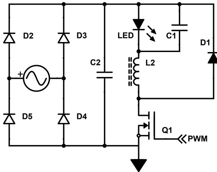
Figure 32: An AC buck converter is a classic LED driver topology. The upstream full bridge rectifier is connected to the AC grid.
