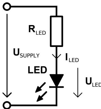
Figure 15: The simplest implementation of a LED driver is to use a series resistor.
