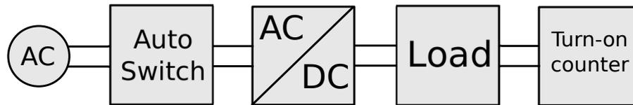
Figure 98: Testing setup for switch on/off test switches the converter on, operates it, and switches it off. A counter measures the repeated cycles.
