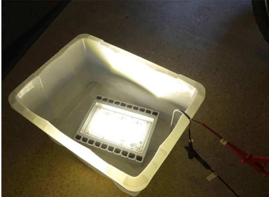
Figure 55: The LED module can be operated under water.
