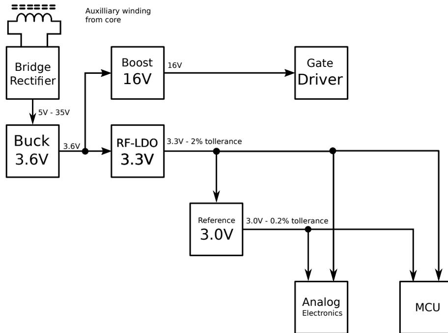
Figure 92: The self supply voltage converter supplies the converters auxiliary power. The auxiliary winding is used to obtain this power, then the power is rectified, down-converted to a 3.6 V rail by a POLC. The 16 V gate driver supply and the 3.3 V internal operation voltage are generated out of this supply. For accurate measurements, a  $\pm 0.2\%$  3.0 V reference is used. For an accurate measurement, analog electronics, like Op-amps, and digital MCU are decoupled by low pass filters.
