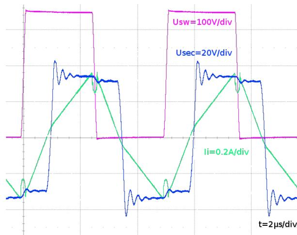
Figure 113: Switching waveform at switching frequency of 200 kHz.
