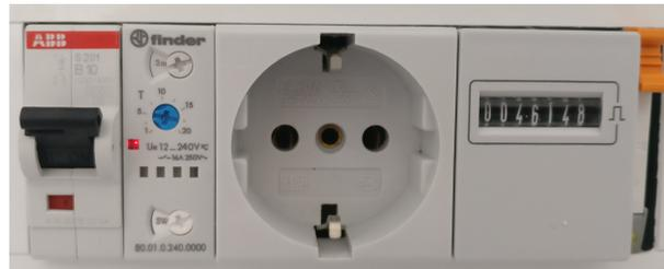
Figure 99: The on/off switching test jig turns the LED driver on for 30 seconds and then turns the LED driver off for 30 seconds. The counter increments with every successful LED driver turn-on.
