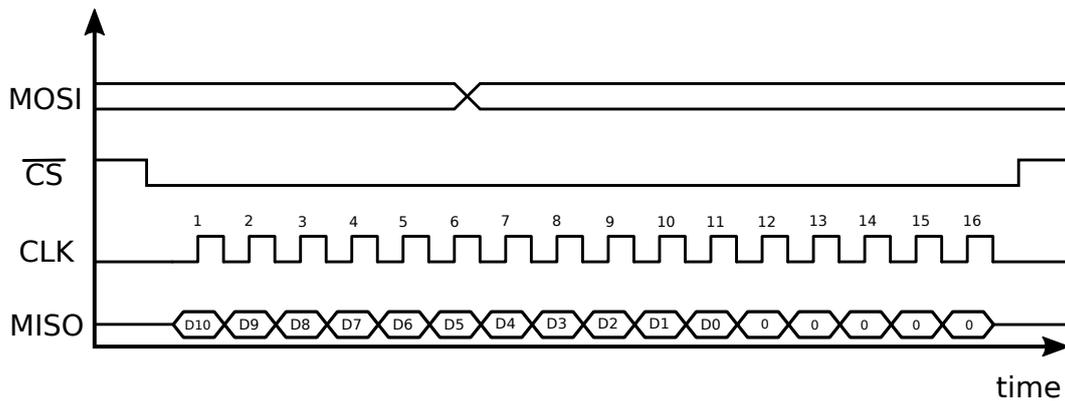
Figure 102: Data acquisition from the ADC using the SPI interface. The DMA requests ADC data in an infinite loop for channel one and two alternatively.
