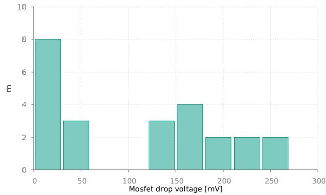
Figure 51: The voltage drop measured over the mosfet without the sense resistor voltage is depicted. It can be observed that even though one batch of LEDs is used, a significant difference in voltage drop can be observed.
