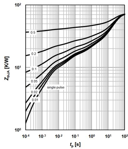
Figure 94: Thermal impedance of the BSP135 depletion mosfet, reproduced from the datasheet [13].
