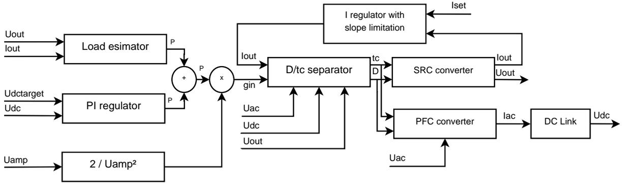
Figure 73: The D-tc separator obtains the input conductance  $g_{in}$  from a load estimator and a PI regulator. The DC output current  $I_{out}$  is measured on the secondary side and offsets are corrected with an I regulator.
