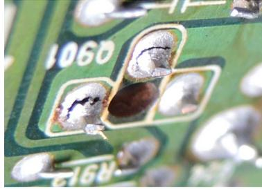
Figure 59: Cracked solder joint of a TV set.
