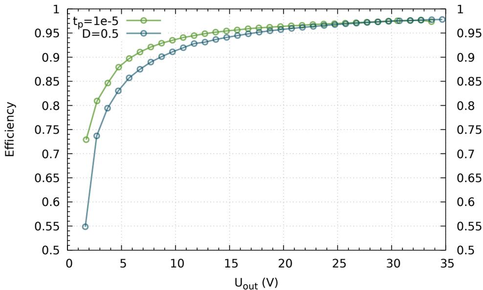
Figure 119: The efficiency is measured over the output voltage range at an output current of  $I_{out} = 1$  A.
