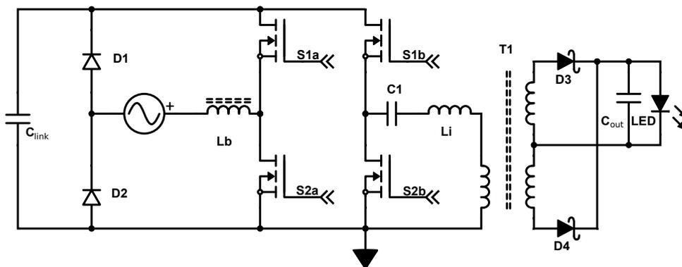
Figure 40: By replacing the bridge rectification by a totem pole PFC topologies, two diode voltage drop may be saved.
