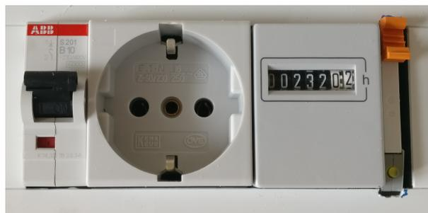
Figure 97: Continuous operation test jig for demonstrating long time operation.
