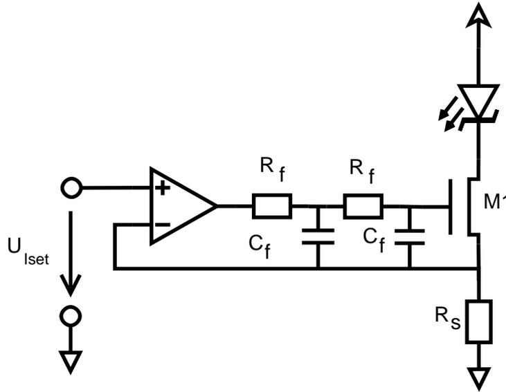
Figure 45: Compensated constant current source, in this example using a second order low pass filter.
