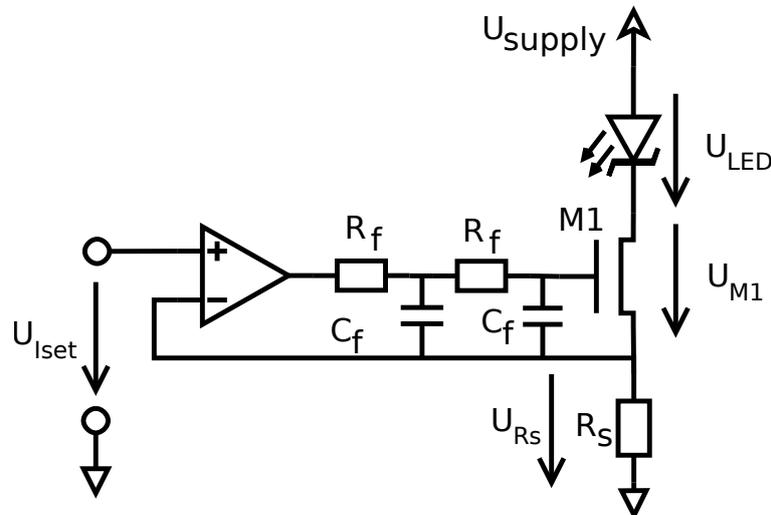
Figure 20: The constant current LED uses an additional low pass filter, to maintain control loop stability.
