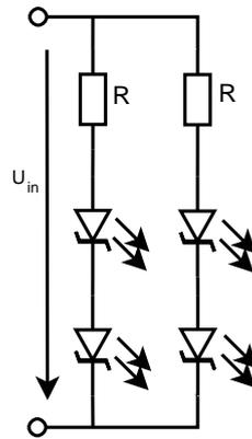
Figure 43: LEDs can be paralleled in the simplest manner by using resistors. While being simple and straight forward that approach has high electric losses.
