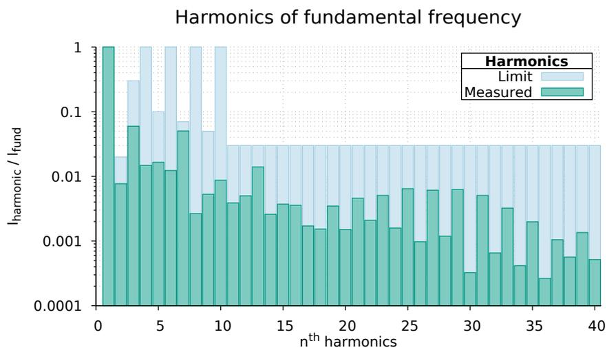
Figure 122: Harmonic measurements according to IEC6100-3-2 Class C
