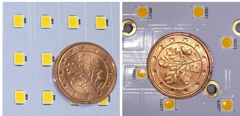
(a) Model "Luxeon 2835" by Lumileds (b) Model "Luxeon 3030HV" by Lumileds
