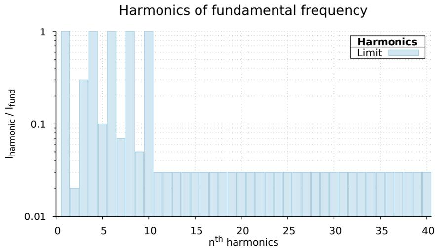
Figure 13: Legal limits of harmonic power consumption relatively to the fundamental frequency[7].
