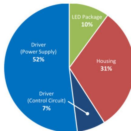
Figure 2: Percentage of failures in outdoor luminaires. Graphic by [4].
