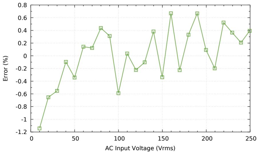
(b) Relative voltage measurement error.
