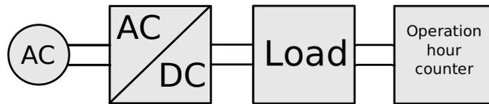
Figure 96: Test setup for continuous operation.
