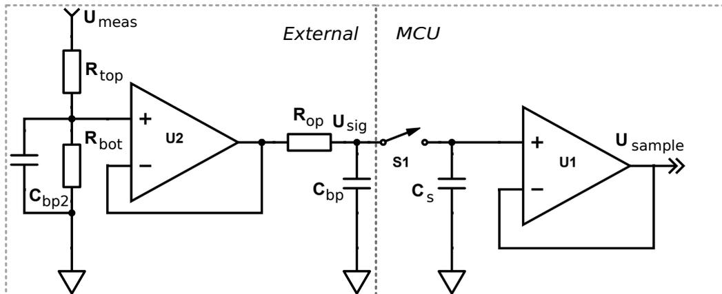
Figure 77: The ADC is driven by an operational amplifier that is configured as an impedance converter. By having a cascaded RC filter a second order low pass filter is implemented.
