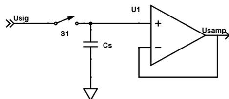
Figure 74: The equivalent input of an ADC sampling circuit. When the switch is closed, the voltage is sampled. When the switch is opened, the signal is on hold.
