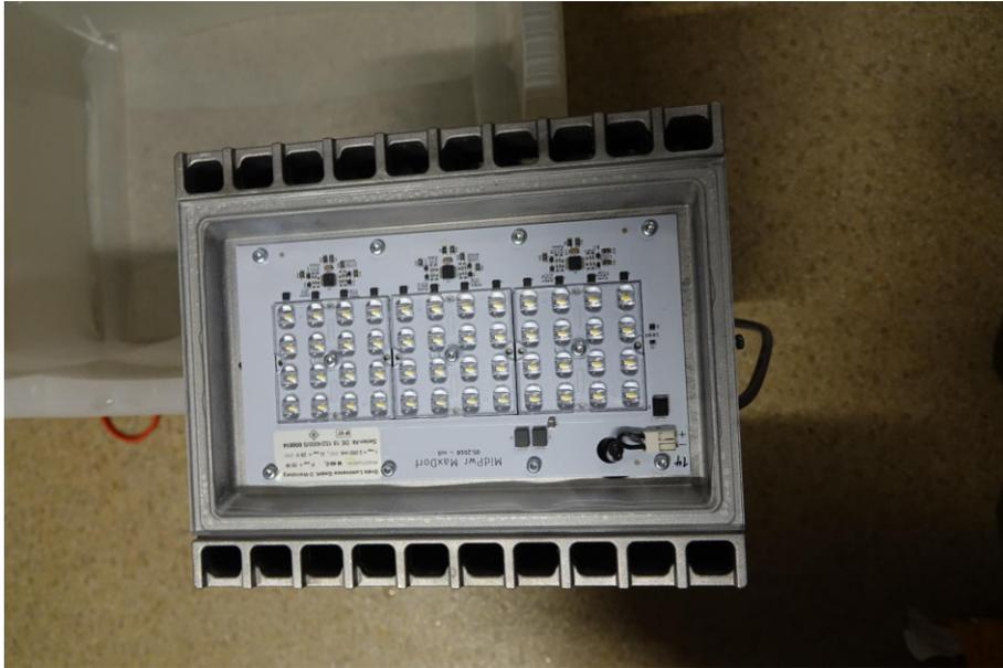
Figure 54: LED Module is integrated in a die cast case.
