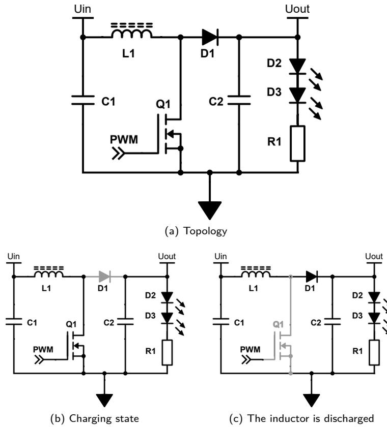
Figure 29: Simplified LED boost converter, showing the the two phase operation principle of a boost converter. A boost converter increases the output voltage.
