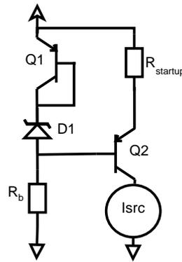
Figure 48: Zener constant current source, which is temperature compensated using matched Q1 and Q2 same die transistors.
