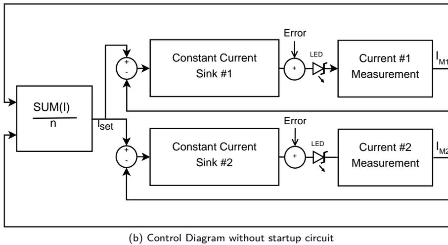
Figure 44: Proposed novel current matching topology, based on a dissipative current limiter with self-determining set current. For startup an additional startup circuit is required.
