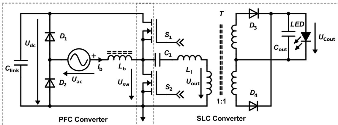
Figure 64: A power factor correction (PFC) circuit and a SLC converter share a single half bridge. State-of-the-art modulation techniques do not filter the double mains frequency on the secondary side [9]. A novel modulation technology will be used to separate the  $C_{link}$  ripple from the secondary side.
