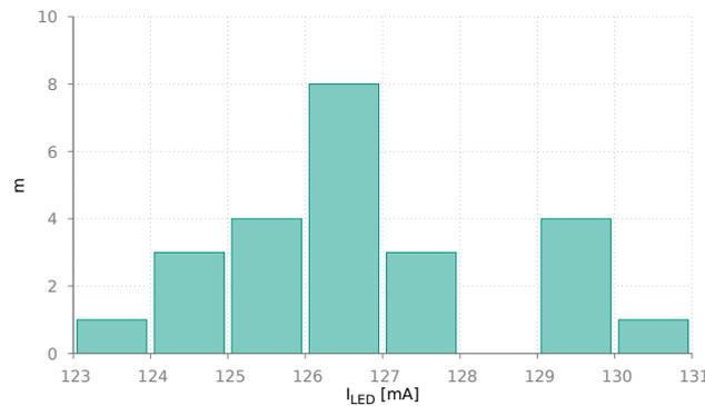
Figure 50: LED current distribution in the range of 123 mA to 131 mA, shows that the LEDs are sufficiently matched.
