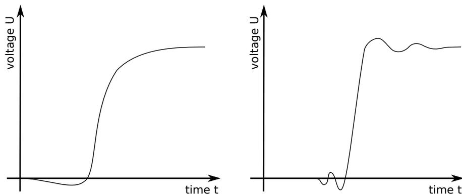
(a) Soft-switching waveform, which has a soft shape without instant changes. (b) Hardswitching shows a significant amount of ringing.
