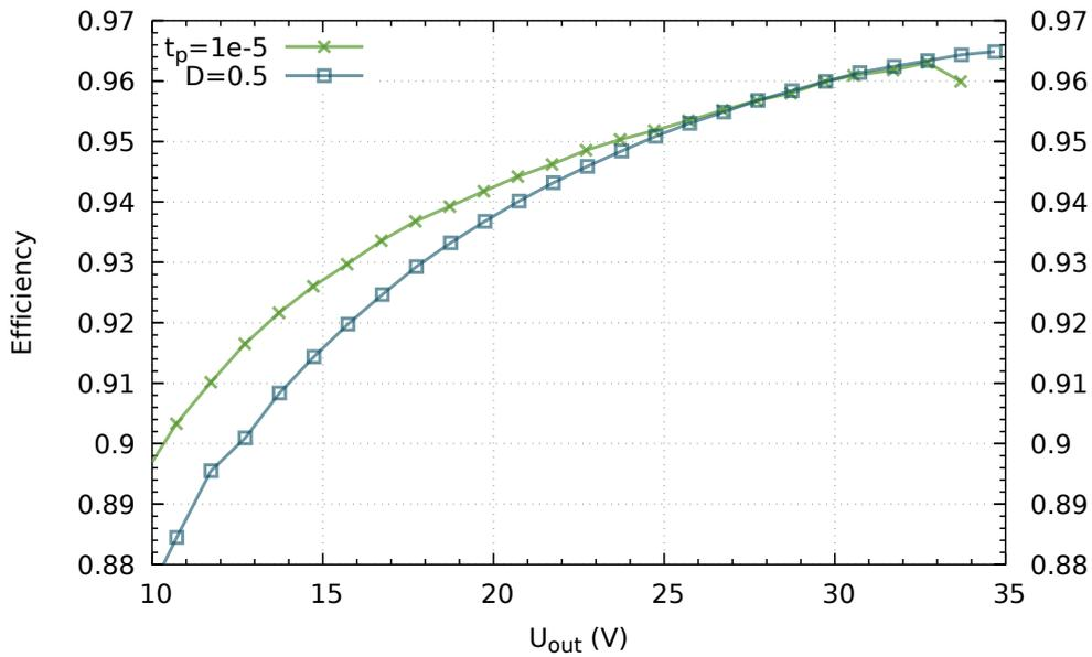
Figure 120: Efficiency at typical operating conditions at an output current of  $I_{\text{out}} = 1 \text{ A}$ .
