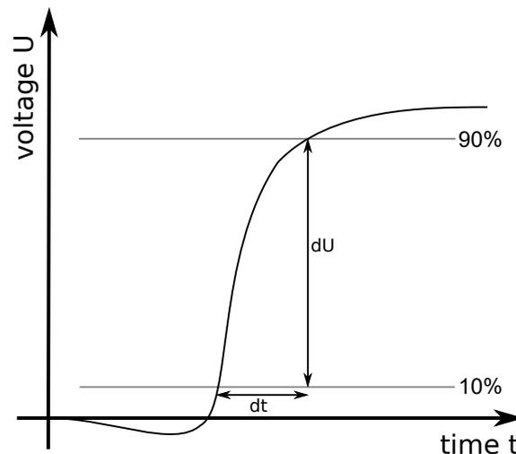
Figure 24: The commutation speed is measured at the switchnode from 10% to 90%.
