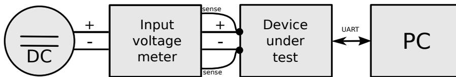
Figure 107: Basic measurement setup: The internal values are measured at the input with a voltmeter. The internal values are monitored using UART by the MCU Tracer. Both measurements values are compared with each other to calculate the measurement accuracy.
