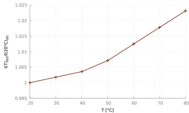
Figure 52:  $I_{SRC}$  temperature drift of the zener transistor startup circuit. (Section 5.4.6).
