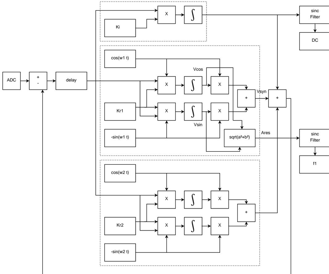
Figure 87: The filter topology is based on [12]. The separator is a control loop consisting out of an integrator tuned to the measurement frequencies. The bandwidth of the resonant observers can be determined by  $Kr_n$ .
