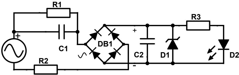
Figure 31: Capacitive voltage dropper for driving LEDs. The voltage is lowered by the capacitor  $C_1$  and  $R_2$ .
