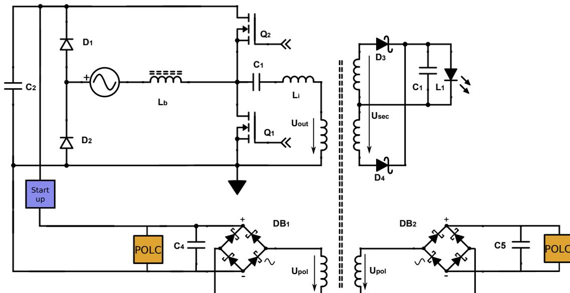
Figure 91: The SLC topology is extended by two auxiliary windings: One on the primary side, one on the secondary side to supply point of load (POL) DC/DC converters that generate all internal voltages.
