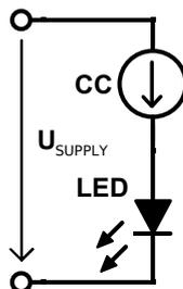
Figure 18: A constant current LED driver ensures a supply voltage invariant LED drive current.
