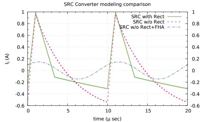
Figure 68: Spice simulation of the inductor current according to topologies in Figure 66 and Figure 67 at  $f_{sw} = 100\text{kHz}$  and  $D = 0.3$ .
