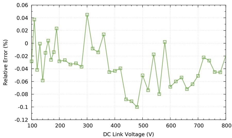
(b) Relative voltage measurement error.
