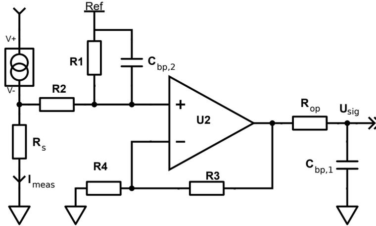
Figure 80: The operational amplifier circuit adds an offset to the sensed current. This allows to measure low currents, where the voltage drop over the sense resistor is below the operational amplifiers offset voltage.
