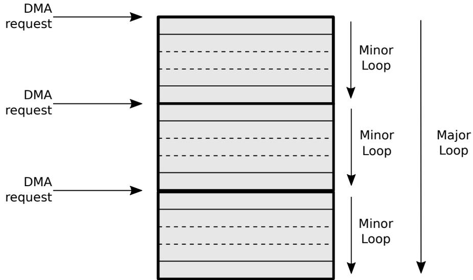
Figure 100: DMA acquisition structure: The data is acquired automatically by the responsible unit. Each data-element is transferred to SRAM by the DMA. After a specific number of transfers an interrupt is issued and the data is processed.
