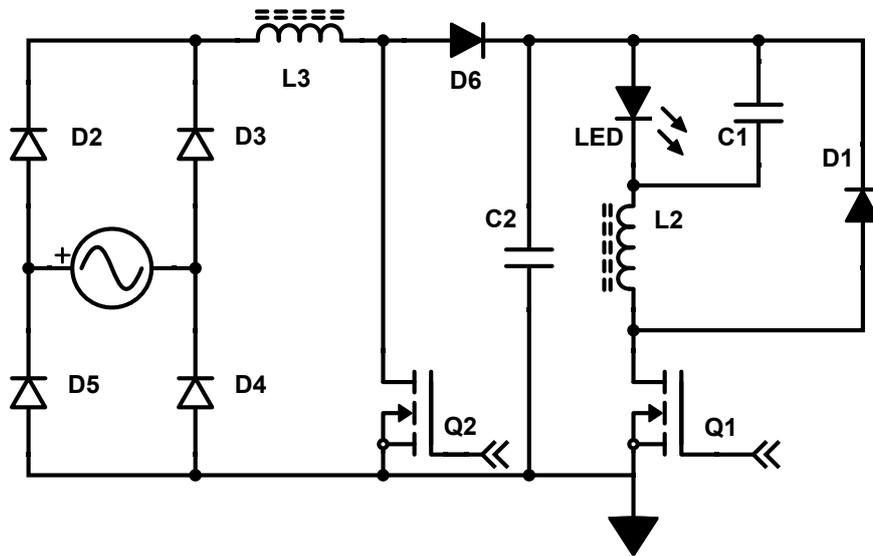
Figure 34: The PFC generates a sinusoidal input current waveform to obtain a power factor close to one. The PFC is an additional circuit, which is placed upstream to the buck converter.
