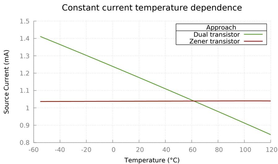
Figure 49: Temperature dependence of the two constant current sources (spice simulation). It can be observed that the zener transistor solution offers improved temperature stability.
