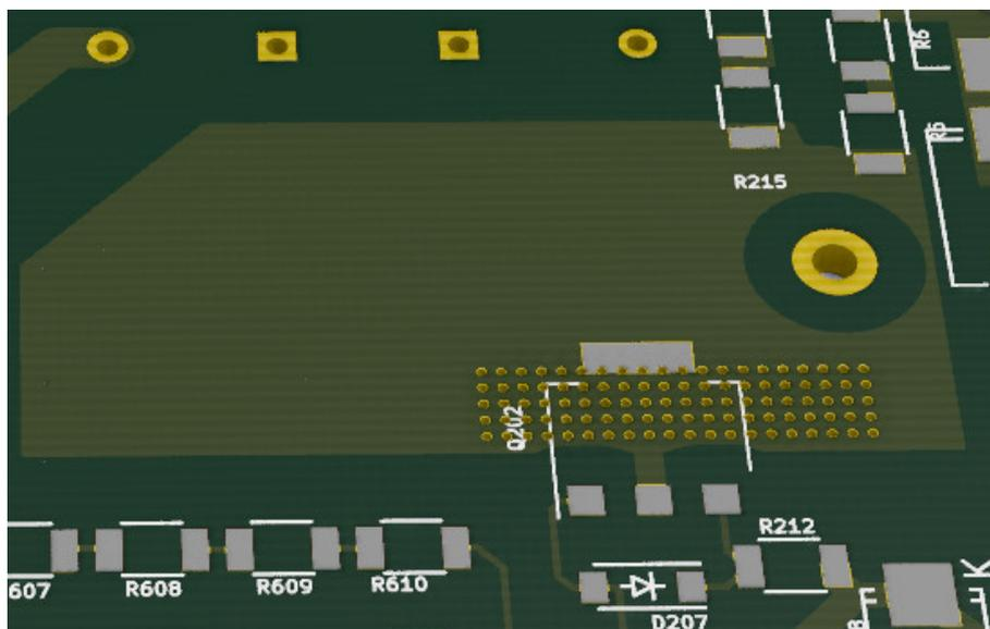
Figure 95: Power planes may be used for cooling power devices: Depletion mosfet Q202 is cooled via a significant power plane, the heat is also conducted to the other side of the PCB by the use of thermal vias.
