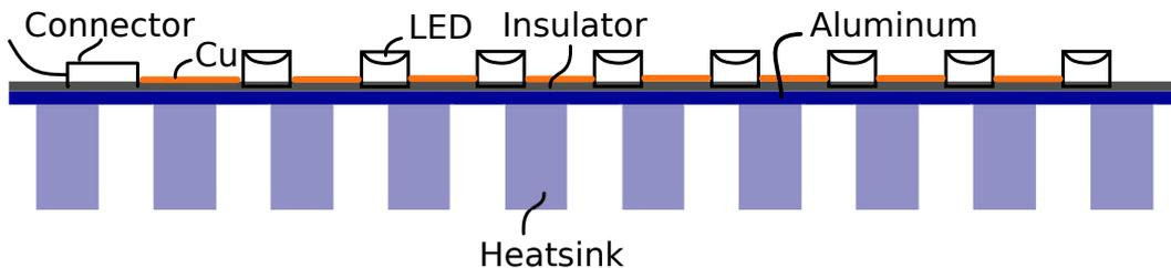
Figure 6: A LED engine consists out of connector, the copper traces for wiring, an insulator and below an aluminum base-plate for mechanical stability and thermal conductivity. Additionally a heatsink is often utilized for maintaining low operating temperatures for long product lifetime.
