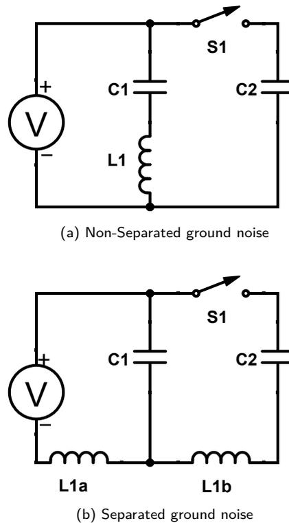
Figure 82: Measurement noise in power converters has often its issue in switching noise that is caused by switching.
