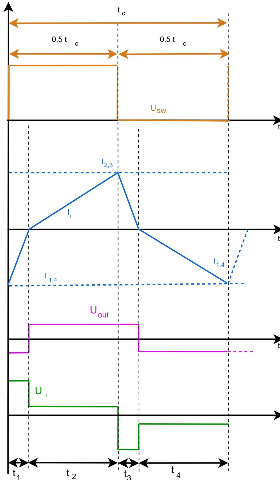
Figure 39: Operational waveforms of the SLC converter operating at a duty cycle of 0.5. The positive and the negative waveform are perfectly symmetric. Therefore, the maximum inductor currents are equal ( $I_{1,4} = I_{2,3}$ ).
