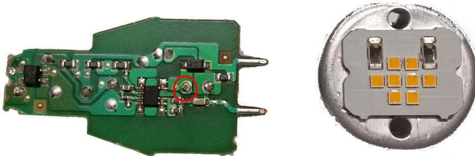
Figure 58: Example of a cracked solder in an Osram buck-converter LED retrofit
