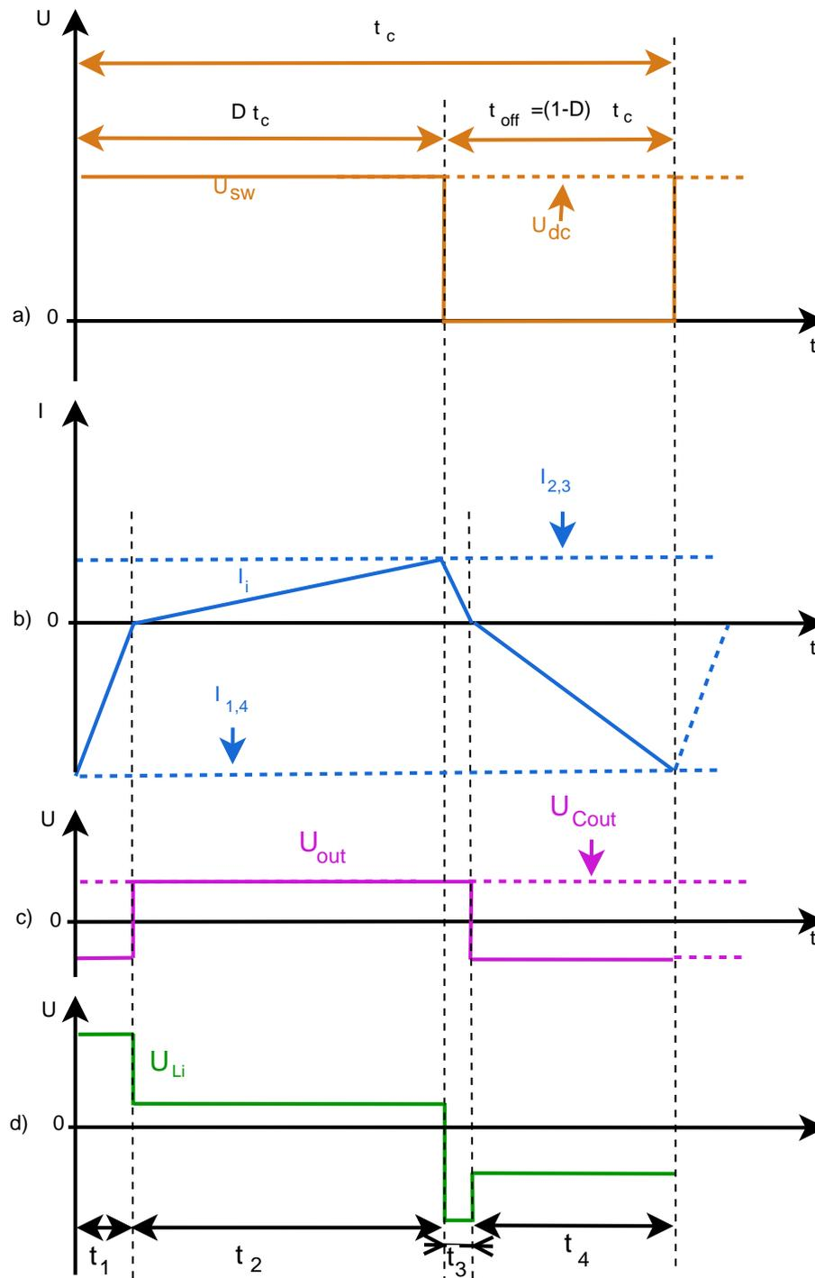
Figure 70: SLC converter switching waveform.
