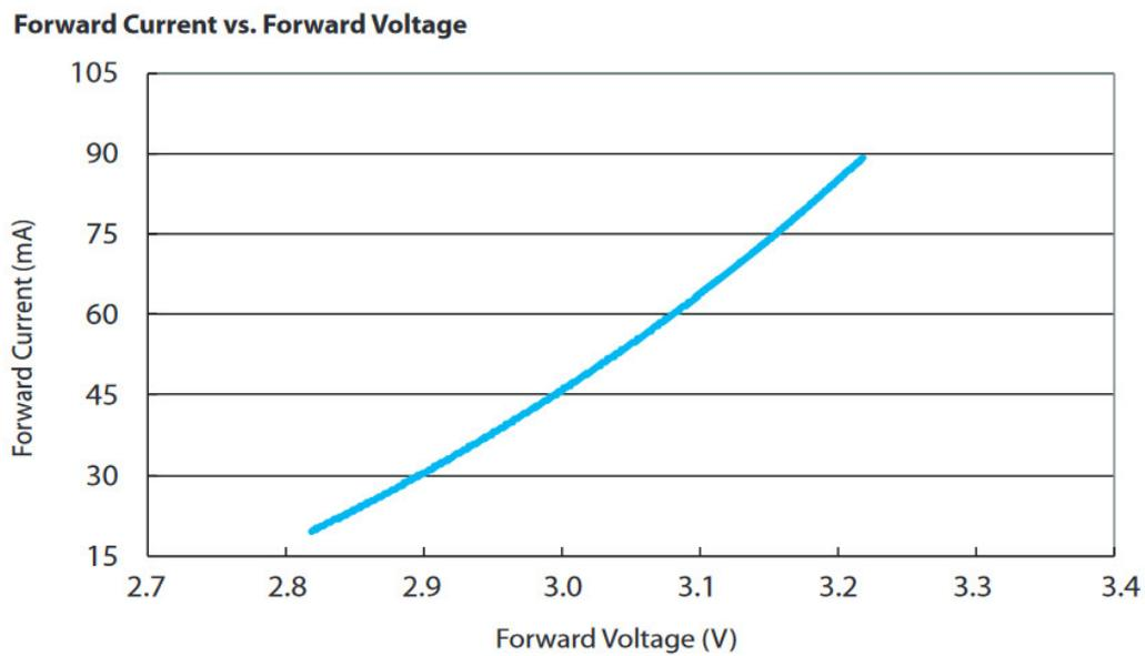
Figure 9: The voltage over current is depicted for the Edison 2835 LED [5]. Clearly the exponential characteristic of the LED forward current can be observed. A small change in voltage leads to a significant change in current.
