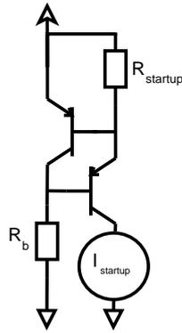
Figure 47: Transistor constant current source, using two transistors. This constant current approach is known to be temperature sensitive.
