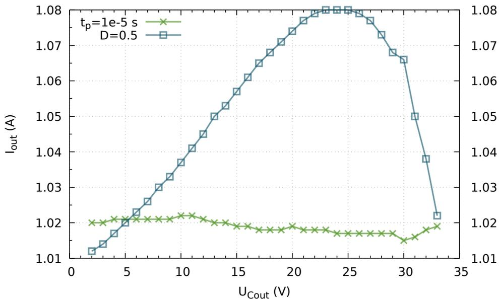
Figure 115: Output current variation over output voltage for duty cycle and frequency modulation.
