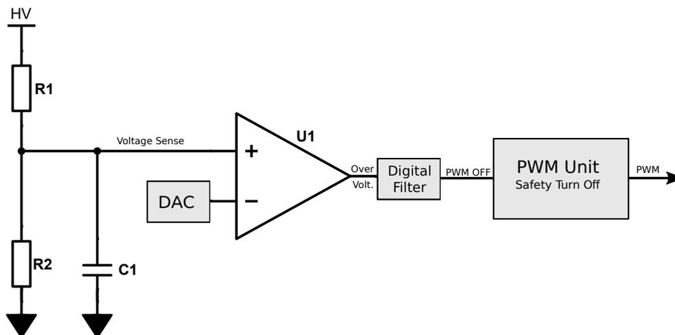
Figure 88: An overvoltage comparator turns off the PWM waveform generator. The overvoltage is filtered analog and digitally.
