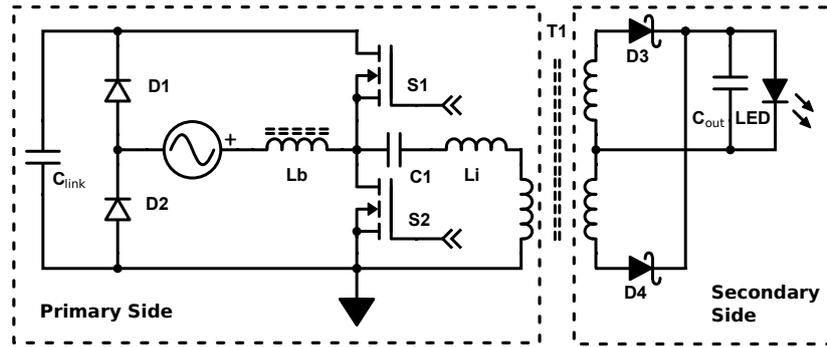
Figure 22: Primary and Secondary Side of a SLC converter.
