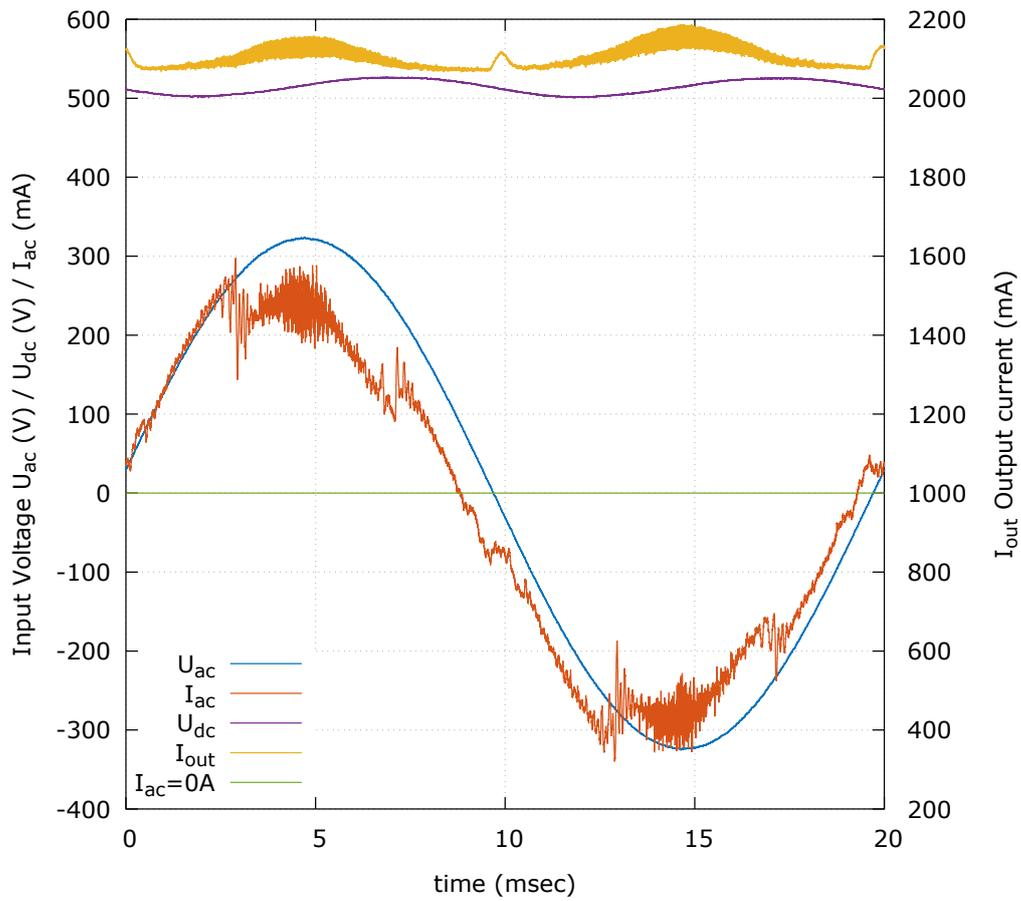
Figure 121: Waveforms of the PFC-SLC Converter
