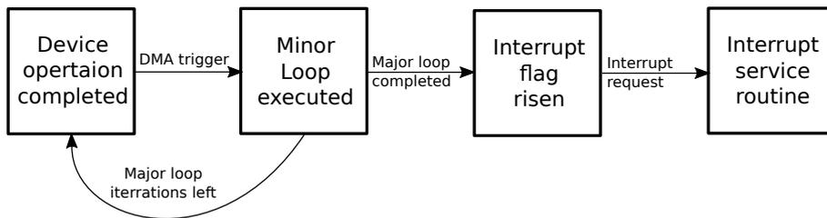
Figure 101: Data transfer flow from acquisition units, e.g. ADCs, is illustrated: When a device operation is complete its data is transferred within the minor loop. When the major loop is completed after several transfers, a interrupt flag is risen. The CPU can perform its calculations based on the acquired data in the interrupt service routine.
