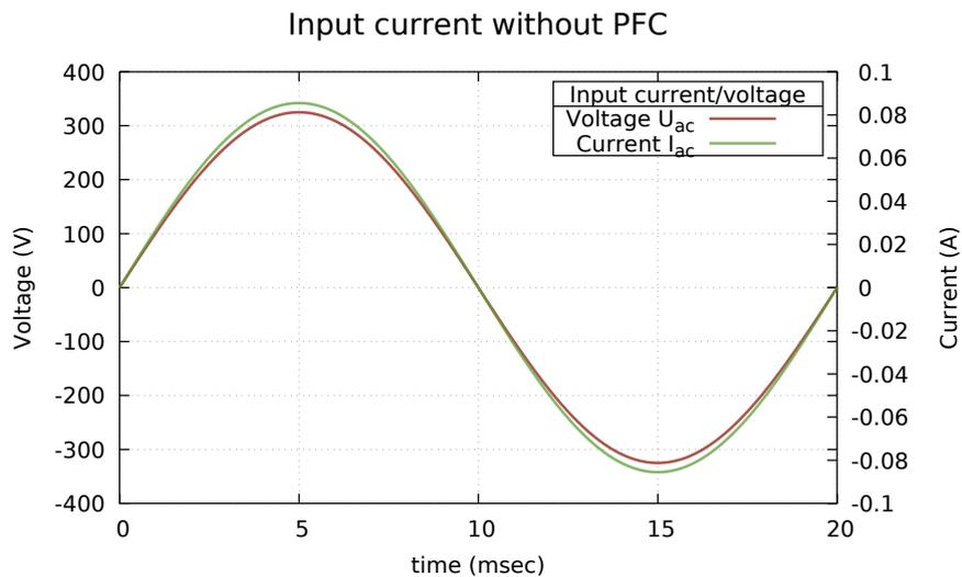
Figure 35: The ideal input current of an ideal PFC converter has a perfectly sinusoidal shape. No phase lag or lead of the current can be observed.
