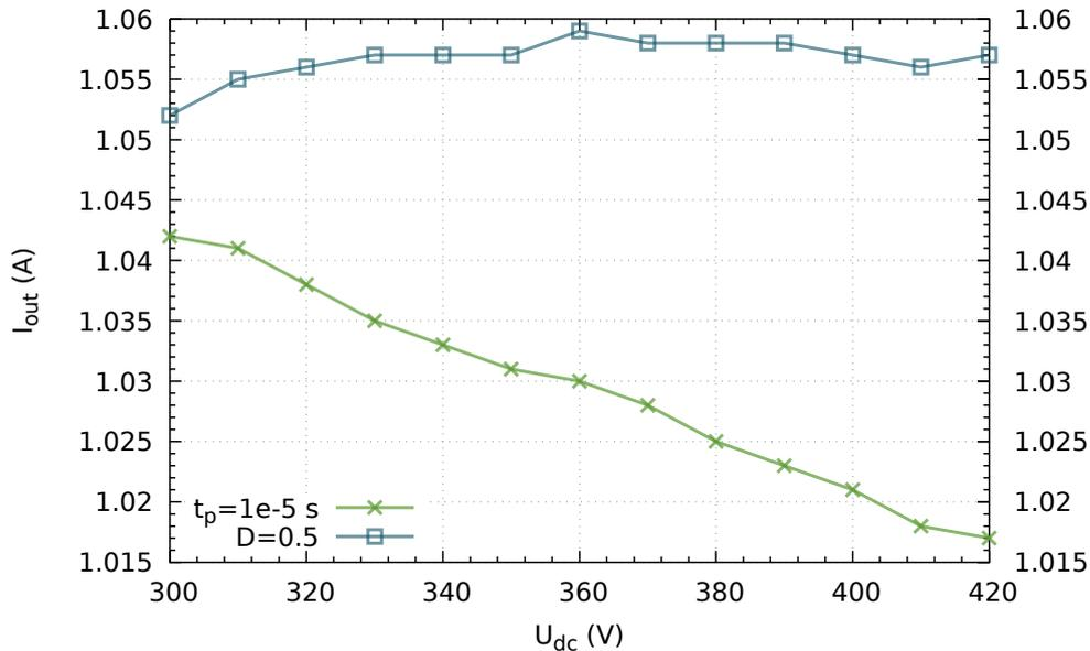
Figure 116: Output current over input voltage for duty cycle and frequency modulation.
