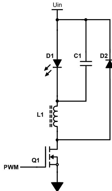
Figure 26: Simplified schematic of an LED buck converter: When the mosfet Q1 is closed, L1 stores the surplus energy. When Q1 turns off and the energy stored in the inductor is used to drive the LED. The current then commutates over the free-wheeling diode D2.
