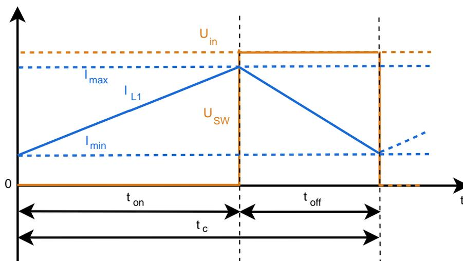
Figure 27: Buck converter waveform showing the inductor current  $I_B$  and the switch-node voltage  $U_{SW}$  over time. The buck converter in this example operates in continuous conduction mode, as  $I_B(t) > 0 \forall t$ .
