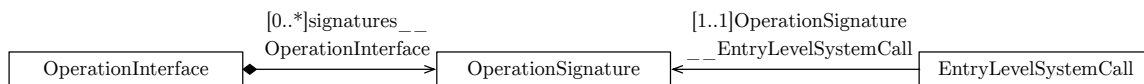
Figure 9.3.: Relationship between an operation interface and the corresponding signatures and entry level system calls - An excerpt from a simplified metamodel based on the PCM [BKR09]
