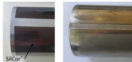
Fig. 6 Pipe coated with SilCor®SiC (left), wrapped and laser-welded (right).
