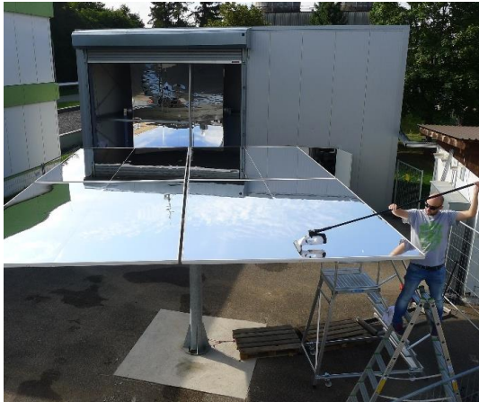
Fig. 7: Test facility SOMMER for concentrated solar power in the Liquid Metal Laboratory.
