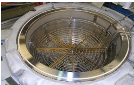
Fig. 1: View into the open test facility LIVE for in-vessel melt retention experiments.
