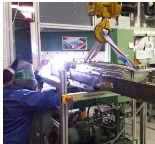
Fig. 6: Insertion of a NaK test loop into the magnet of the MEKKA laboratory.
