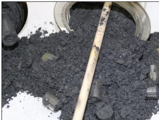
Fig. 10: Carbon produced from pyrolysis of methane in the KALLA laboratory.
