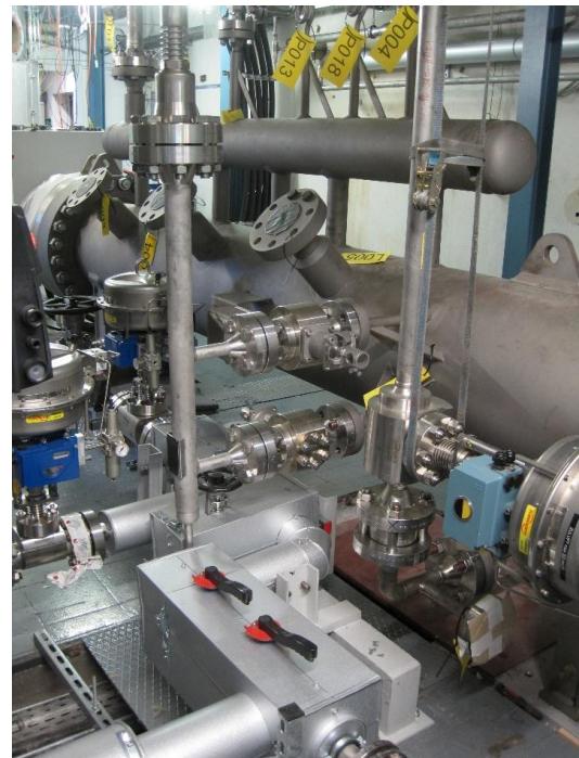
Fig. 11: Evaporator of COSMOS-H, designed for critical heat flux experiments at high pressure.
