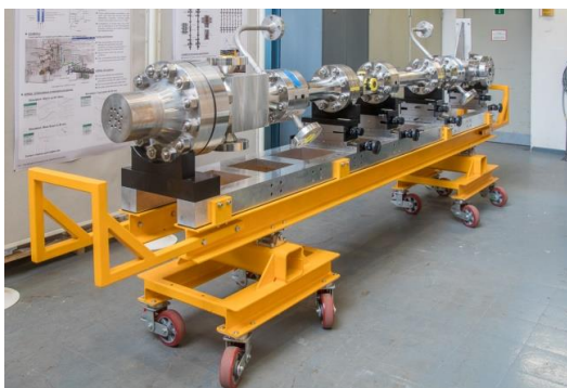
Fig. 7: (top) Ground floor at construction Site COSMOS-H, (bottom) modular high pressure test section for COSMOS-H
