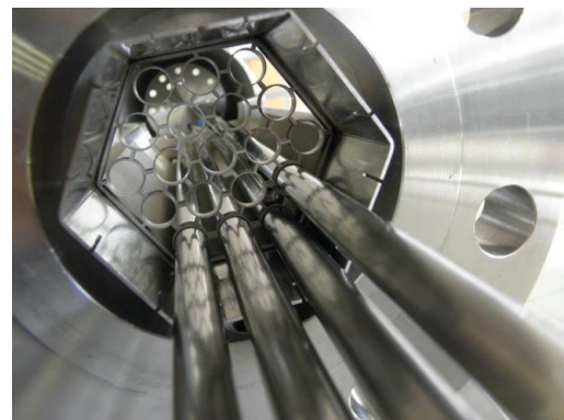
Fig. 1 top view of the fuel pin bundle simulator for the NACIE facility, schematic view (top), actual picture (bottom), [2].
